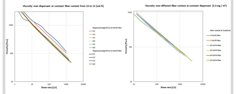
Viscosity vs dispersant concentration. Best flowability could be reached with dispersant concentrations > 2.2 mg/m<sup>2</sup>
