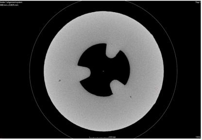
CT cross section image with internal guide bars
