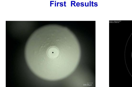
Front view of ceramic capillary  $\emptyset = 40 \ \mu m$
