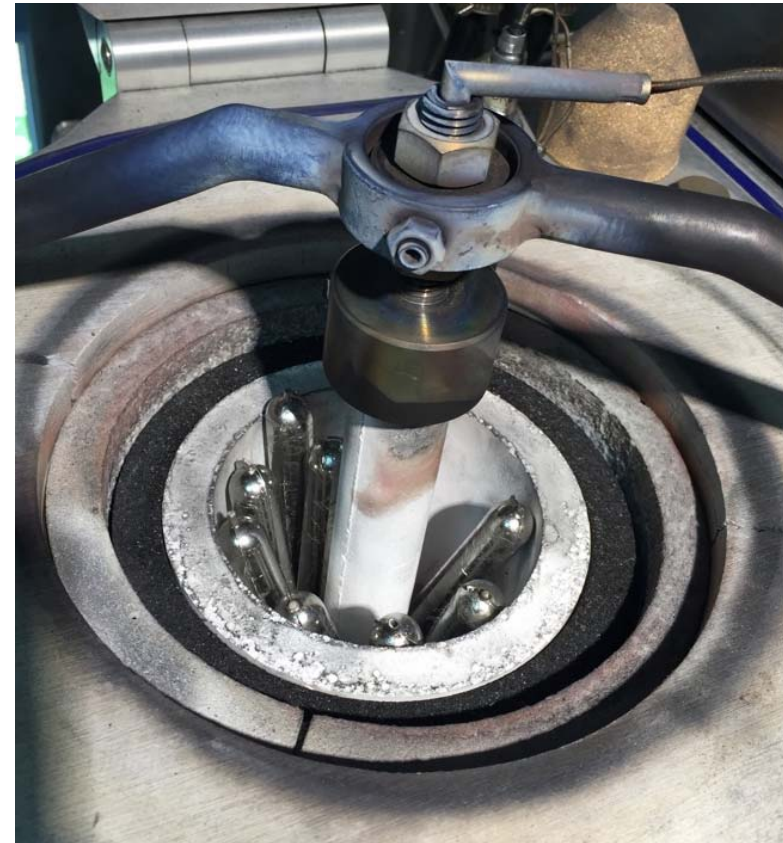
CoCrFeMnNi rods in a crucible of a vacuum induction furnace
