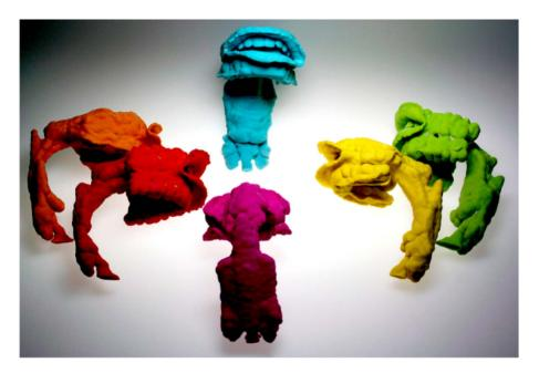
Fig. C.2 3D printouts of different phonations of the vocal tract acquired by MR imaging and printed with a powder printer.
