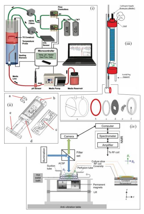
Fig. 4.1 The most significant MR compatible incubation systems. (i) The microcontroller controlled e-incubator for monitoring of engineered bone tissue reprinted from [55]. (ii) Incubation chamber for MR imaging of rat optic nerves reprinted from [63]. (iii) In-bore oxygenator for vertical MR systems for cortical rat brain slices reprinted from [67]. (iv) Open low field system for 1D MR measurements of cortical rat brain slices reprinted from [65].
