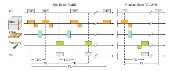
Fig. 2.2 Timing diagrams for gradient echo (FLASH) and (turbo) spin echo (RARE) imaging sequences.
