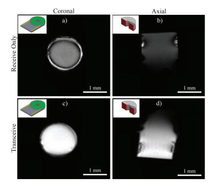
Fig. 3.16 Coronal and axial MRI sections through a hollow micro-coil in receive only (a and b) and in transceive mode (c and d). Image reprinted from [196].
