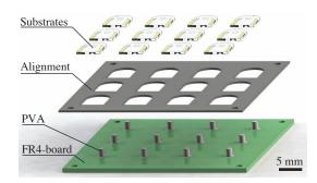
Fig. 3.10 Cast PVA posts on a FR4-board. The substrates are aligned with an alignment frame. Image reprinted from [196].
