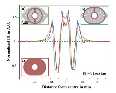
Fig. 3.21  $B_1$  field profile simulation three Lenz lenses normalised by a  $B_1$  field of a 50 mm diameter Helmholtz excitation coil.
