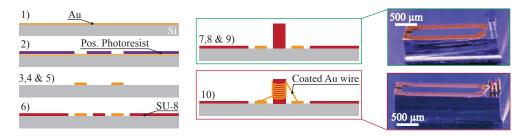
Fig. 3.3 Process flow for MRFM microcoils
