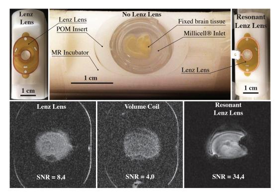
Fig. 5.3 A fixed half brain slice mounted in the MR incubator with the Lenz lens as signal amplifier. The signal to noise ratio increases significantly from a 72 mm diameter volume coil to a broadband Lenz lens and a resonant Lenz lens.
