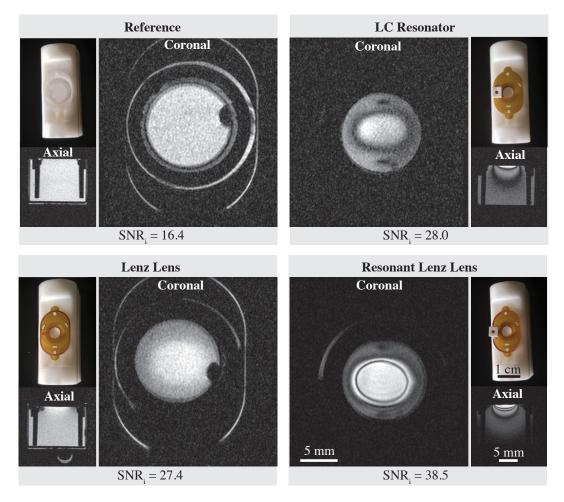
Fig. 3.24 Comparison of MR imaging using only a 72 mm volume coil (reference), an LC resonator, a Lenz lens and a resonant Lenz lens (all with an inner diameter of 5 mm). A non-RF-spoiled FLASH sequence was used with parameters TR = 200 ms, TE = 3 ms, slice thickness = 1 mm, FOV = 2 x 2 cm<sup>2</sup>, MTX = 200 x 200 and NEX = 8.
