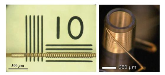
Fig. 3.2 Left: A micro coil manufactured by laser-lathe lithography with a diameter of  $100\,\mu$ m. Image reprinted with permission from [182]. Right: A solenoidal micro coil manufactured by winding with a wire bonder. Image reprinted with permission from [185].
