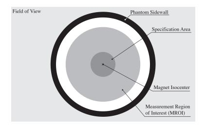
Fig. 2.6 Areas of interest in an MR image for computing the image SNR according to [112].
