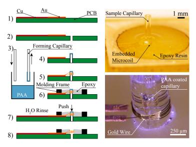
Fig. 3.7 Hollow coils first trials. Image adapted from [205].
