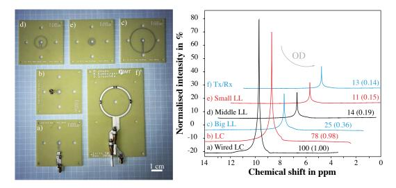
Fig. 3.20 Left: Images of the (a) the wired LC resonator, (b) the LC resonator, (c) the big, (d) the middle, (e) the small lenz lenses with inner coil diameter of 5 mm and (f) the reference Tx/Rx coil. Right: Collected spectra from a 4.5 mm diameter  $40\,\mu$ l water sample with their normalised intensities in %. The values for the normalised integrals (integrated from 8 ppm to 2 ppm) are given in brackets.
