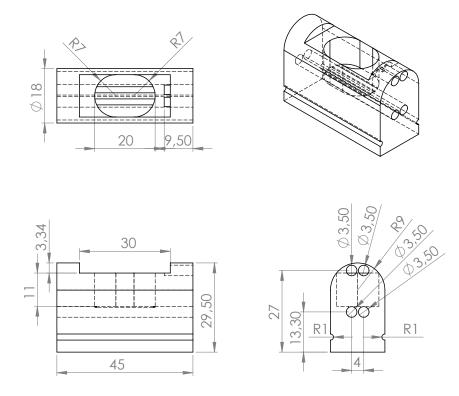
Fig. H.1 Technical Drawing of the MR compatible incubation platform. All values are given in mm.
