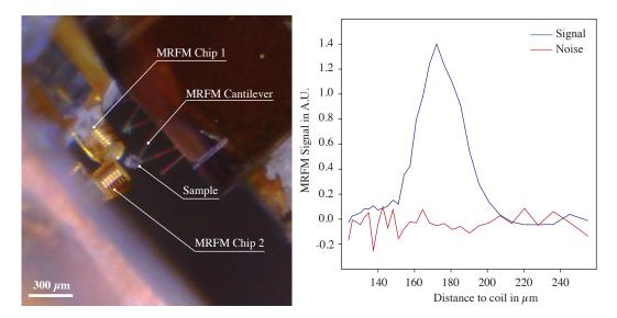
Fig. 3.5 Left: Photo of the the MRFM measurements setup, with two of the manufactured MRFM chips built in. The MRFM cantilever and the Ammonium sulfate crystal (sample) are clearly visible. Right: MRFM measurement recorded with the depicted setup.
