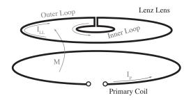
Fig. 3.18 Schematic representation of the primary coil and the Lenz lens w.r.t. each other.
