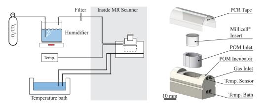
Fig. 4.4 Left: Schematic of the MR compatible nurturing system for brain slice culturing, incorporating a humidified gas supply, a temperature bath for temperature control and the MR incubator itself. Right: Exploded view of the MR incubator.
