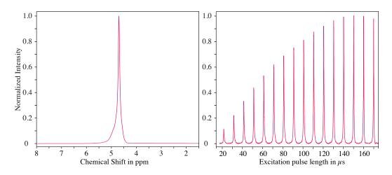
Fig. 3.15 NMR spectrum (left) and nutation spectrum (right) of water, recorded in a 400 MHz Bruker Biospin system with the manufactured micro-coil.
