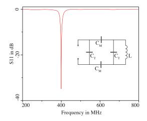
Fig. 3.14 S11 curve of a hollow micro-coil, tuned and matched to 400 MHz and 50 Ohm and a schematic of the tuning and matching network.
