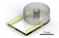
Fig. 3.9 Rendered CAD model of the externally supported microcoil mounted on the Pyrex substrate (designed and rendered with Solidworks 2014 (*Dessault Systems SE, France*)). Image reprinted from [196].
