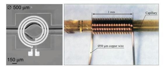
Fig. 3.1 Left: A spiral surface micro coil (image reprinted with permission from [164]). Right: Hand-wound solenoidal micro coil as introduced by Olson *et al*,. Reprinted with permission from [165]. The labels have been added.
