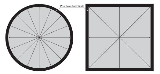
Fig. 2.7 Distances to be compared in a circular phantom (left) and a rectangular phantom (right) to compute the geometric distortion modified from [111].
