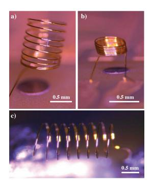
Fig. B.1 Two different free standing micro coils manufactured by wire bonding. Top: By dissolving the support post. Bottom: By coil transplantation.
