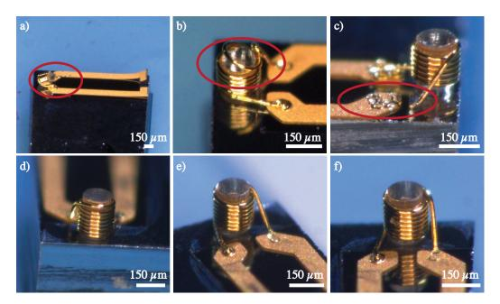
Fig. 3.4 Failure mechanisms during wire bonding of small micro coils. a) If the adhesion of the wire bond post is not promoted by an adhesion layer, the posts chips off during wire bonding. b) If the SU-8 post height is too low, the top winding(s) do not form a coil. c) If the bond pads are not clean, the wire bond rips off. A micro coil, manufactured with the described process. d) front view, e) side-view and f) back side.
