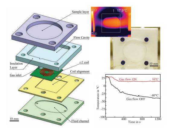
Fig. A.1 A modular platform for cryogenic cooling of an r.f. coil with active insulation. When the gas flow for active insulation is switched on, the temperature at the sample are stabilises at 16 °C. A significant part of this platform was developed in the master thesis of Agazi Tesfai [MA1].
