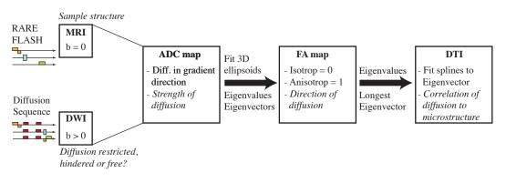
Fig. 2.4 Processing pipeline from DWI to DTI.
