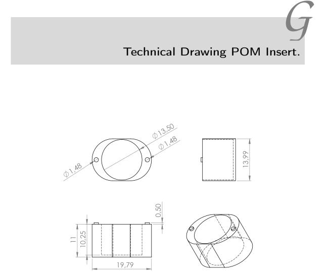
Fig. G.1 Technical Drawing of the POM insert used in the MR incubator. All values are given in mm.
