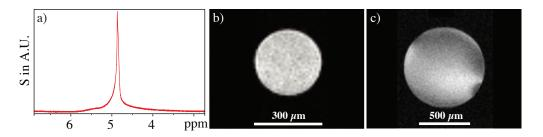
Fig. 3.8 MR measurements of a micro coil, manufactured by dip-coating of capillaries. Left: An MR spectrum of pure de-ionized water with FWHM = 0.055 ppm. Middle: MR image of the micro coil with a capillary inserted, with  $SNR_i = 9.6$ . Right: MR image of the micro coil volume completely filled with de-ionized water yielding  $SNR_i = 16.6$ .
