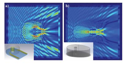
Fig. 6.1 COMSOL simulation of an impinging microwave at 500 GHz. While the current design (a) of the hollow micro coils embedding material reflects the microwave, a redesign (b) focuses the microwave into the sample area. These simulations were done by Suleman Shakil, Laboratory of Simulation, University of Freiburg.
