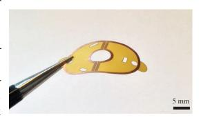
Fig. 3.22 Photo of a flexible Lenz lens manufactured with the described process.
