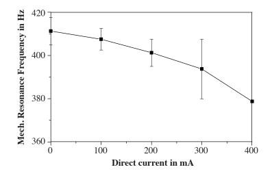
Fig. B.2 The mechanical resonance frequency of free standing micro coils drops with the application of direct current. This measurement was recorded with a vibrometer on 4 seperate free standing micro coils.
