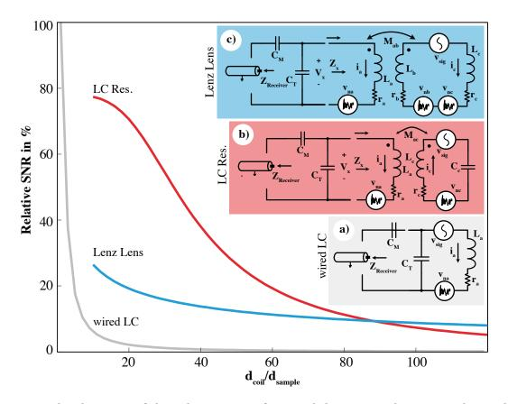
Fig. 3.19 The decrease of the relative SNR of a wired detector coil (a), an inductively coupled LC resonator (b) and a Lenz lens (c) and computed from their circuit schematics for increasing coil diameters and a fixed sample diameter.
