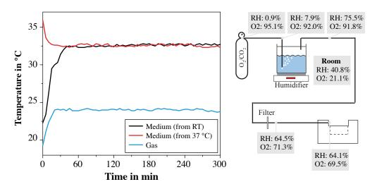
Fig. 4.6 Left: Temperature profiles of the nurturing medium in the incubator and the carbogen gas, wich stabilises over time. Right: Relative humidity (RH) and oxygen content (O2) of the gas supply at different points of the set-up.
