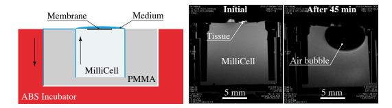
Fig. 4.3 The nurturing medium is presumably sucked out of the PMMA inlet by capillary forces. This leads to rapidly vanishing nurturing medium.
