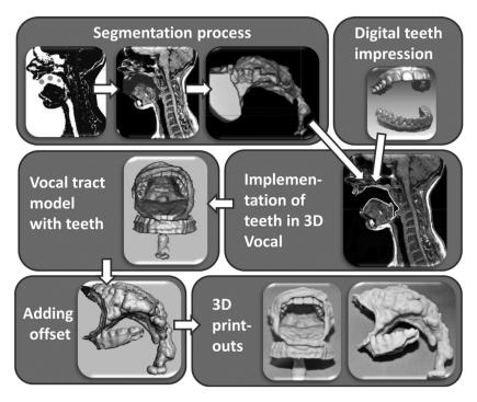
Fig. C.1 Workflow from MR image acquisition to 3D printout of a human vocal tract while phonation. Reprinted with permission from [269].
