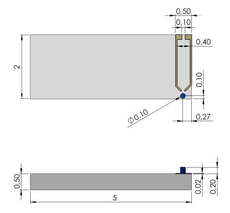
Fig. F.1 Layout of the MRFM Chips. All values are given in mm.
