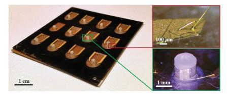
Fig. 3.11 Bottom: Array of wire bonded microcoils, wound around PVA posts. Upper right: Magnified view of one of the wire bonded microcoils. Upper left: Secured wedge bond. Image reprinted from [196].
