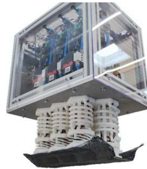
Fig. 9. Built prototype of a drape gripper
