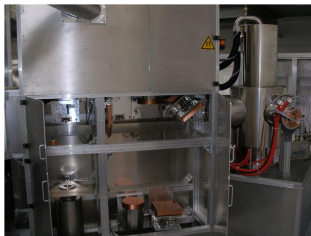
Fig. 2. Gyrotron (right) connected to a Matching Optics Unit (left)
