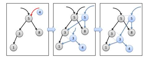
Figure 6.1.: The figure shows the insertion of a node with key 4 into a tree which is shared among two sets. Since the root has a reference count of 2 the copying of nodes is propagated along the insertion path. On the last figure we fix the reference counts of the nodes which have been copied and adjust the pointers accordingly.
