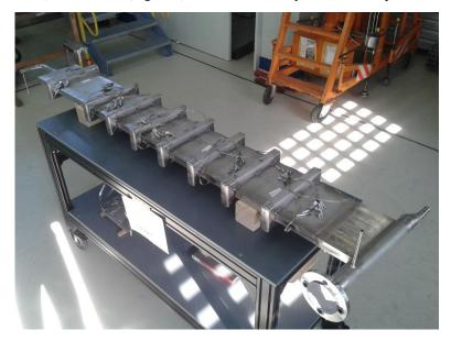
Figure 1: Test section of DITEFA with its 85 installed thermocouples prior to be pre-cleaned before filling.
