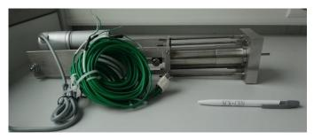
Figure 2: First prototype of the permanent magnetic probe.
