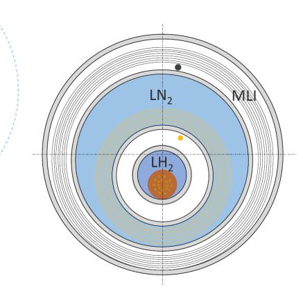
MgB<sub>2</sub> cable:  $d_c = 9 \text{ mm}$  I = 10 kAU = 320 kV
