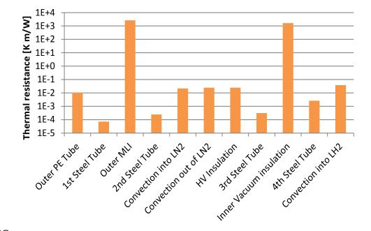
Calculation based on literature data  $\dot{q}_{300 \text{ K} \to 77 \text{ K}} = 4.3 \text{ W m}^{-2}$  $\dot{q}_{77 \text{ K} \to 20 \text{ K}} = 0.9 \text{ W m}^{-2}$
