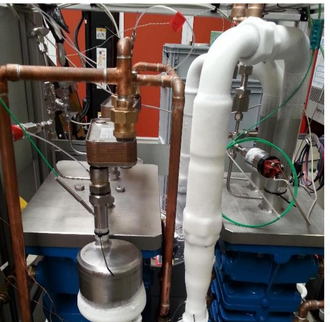
High capacity pulse tube cryo cooler at test stand
