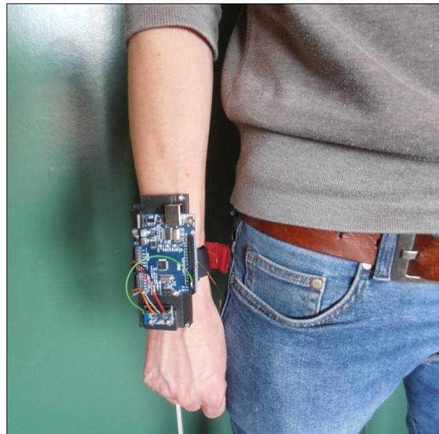
Figure 3: The prototype generator with a microcontroller and accelerometer during the evaluation.
