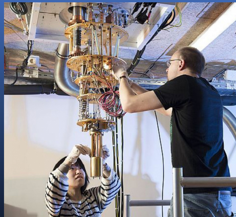
Dilution refrigerator (QUTECH - TU Delft)
