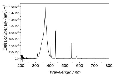
Figure 7-3. Emission spectrum of the lamp iSOLde Cleo Compact PL-L 36 W.
