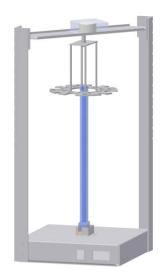
**Figure 7-1.** Schematic setup of the photoreactor used in this study. The samples are placed in the holder and rotated during the irradiation.<sup>266</sup>
