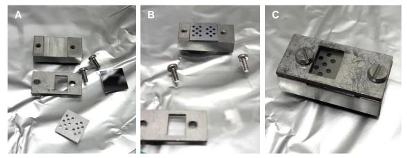
**Figure 7-4.** Assembly of the sample holder for the photo-induced spatially resolved surface immobilization. A: Individual parts disassembled, **B**: Surface and photomask placed onto the sample holder. **C**: Sample holder fully assembled with the photomask mounted onto the silicon wafer.
