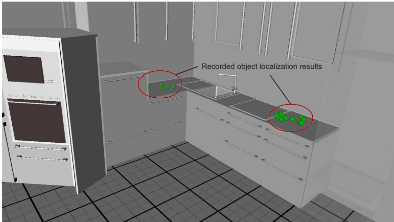
Figure 6.4: Previously seen locations of an object (green spheres), which are clustered to density distributions in order to generate common object locations. The cluster on the right side represents the top location hypothesis, since the object has been seen at this location more often. Source: (Wächter et al., 2018) © Elsevier 2018
