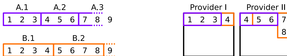
Figure 2. Files are allocated to provider nodes with the grouping observed in jobs. The example shows two jobs A and B, processing the same data with jobs A.1, A.2, and so on. Groups are first randomly allocated for the more often occurring jobs A. The similar groups of B are allocated to hosts where most files are already present.
