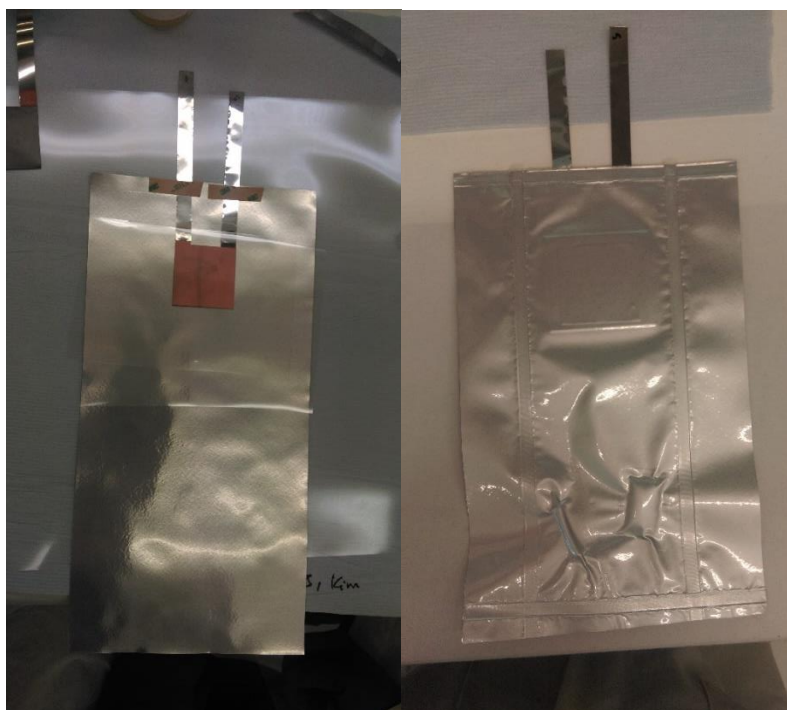
Figure 58. a) Open and b) closed full pouch cell.
