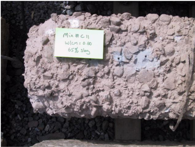
Fig. 7—Scaling on Concrete Block C11 with 0.6 w/cm and 65% GGBFS.
