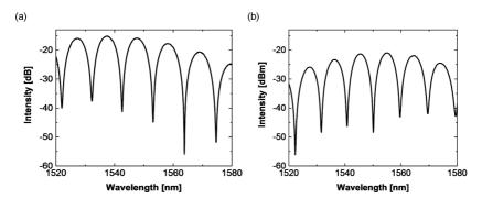
**Fig. 5.8**: Fiber-to-fiber transmission for MZM coated with SEO100. (a) optical transmission measurement of a MZM with a 1.1 mm long active slot waveguide section. (b) optical transmission measurement of a 0.5 mm long MZM. An intentional imbalance in the interferometer leads to the fringes with approx. 5 nm periodicity. The envelope of the transmission curves is due to the response of the grating coupler over wavelength.
