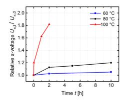
**Fig. 5.2:** Measurement of the increase in  $\pi$ -voltage over time for SOH MZM with SEO100. The devices were tested at 60 °C, 80 °C and 100 °C for 10 h. While for 100 °C a large increase is measured after the first 2 h, for 80 °C and 60 °C after a burn-in of 2 h the increase of the  $\pi$ -voltage is significantly reduced.
