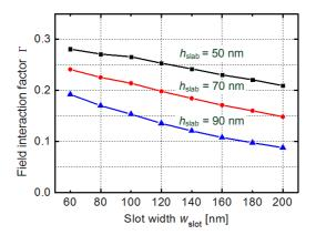
**Fig. 3.2:** Field interaction of the optical mode with the EO material in the slot  $A_{\rm slot}$  as function of slot width at a wavelength of 1550 nm. The rail width was fixed at  $w_{\rm rail} = 240$  nm which is approx. the optimum value for a height of the silicon layer of  $h_{\rm Si} = 220$  nm. Thin slabs and narrow slots lead to a high field interaction factor, however, it has to be balanced with bandwidth requirements of the modulation.
