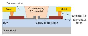
**Fig. 5.6:** Partial cross-section of an SOH phase modulator in the IME process flow. An oxide opening process is used to access the slot waveguide after backend processing and deposit the EO material in the slot. Highly doped silicon with a height of 220 nm is used to provide a path with low resistivity between the slot and the metal electrodes. Only in the vicinity of the slot thin, lightly doped silicon slabs are used for a good confinement of the optical mode.
