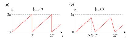
**Fig. 4.3:** (a) Illustration of an ideal sawtooth signal with period T and. The linear slope reaches from 0 to  $2\pi$ . (b) Approximation of a real sawtooth signal with fall time  $T_f$ , the slope of the signal is the same as for the ideal signal.
