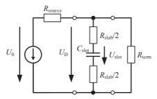
**Fig. 3.7:** Equivalent circuit of an SOH phase modulator in a lumped element approximation. The source is described with the open loop voltage  $U_0$  and the source resistance  $R_{\rm source}$ . The modulator is modeled as RC element with the resistance  $R_{\rm slab}$  for both silicon slabs and the capacitance of the slot  $C_{\rm slot}$ . The device is terminated with  $R_{\rm term}$ .
