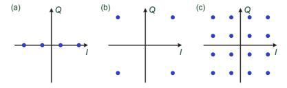
**Fig. 2.3:** Exemplary constellation diagrams for advanced modulation formats. (a) Constellation diagram of a 4ASK signal, only the in-phase component of the carrier is modulated with a multi-level signal. (b) Constellation diagram of a QPSK signal. The in-phase and quadrature component are each modulated with a binary signal. (c) Constellation diagram of a 16QAM signal, the in-phase and quadrature component of the carrier is modulated with a multilevel signal.
