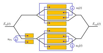
Fig. 2.2: Schematic of an IQ modulator. The incoming carrier is split in two arms. After inducing a relative phase shift of  $\pi/2$  using the static voltage  $u_{ps}$ , the in-phase and the quadrature component can be modulated independently by two MZM in push-pull configuration. At the output, both signals are combined. With an IQ modulator each point in the complex plane can be addressed.
