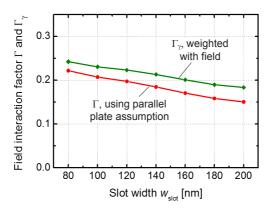
**Fig. 3.3:** Comparison between field interaction factor  $\Gamma$  and weighted field interaction factor  $\Gamma_{\gamma}$  for different slot widths. The slab height is  $h_{\rm slab} = 70~{\rm nm}$ , the rail width  $w_{\rm rail} = 240~{\rm nm}$  and the device height  $h_{\rm Si} = 220~{\rm nm}$ . The weighted field interaction factor shows approximately 10% higher value than the field interaction factor calculated only with parallel plate assumption.
