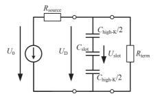
**Fig. 3.8:** Equivalent circuit of a capacitive coupled SOH phase modulator in a lumped element approximation. The source is described with the open loop voltage  $U_0$  and the source resistance  $R_{\rm source}$ . The modulator is modeled as capacitor comprising the capacitance  $C_{\rm high-K}$  for the dielectric and the capacitance of the slot  $C_{\rm slot}$ . The device is terminated with  $R_{\rm term}$ .
