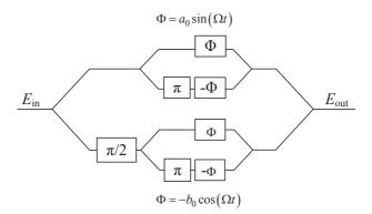
**Fig. 4.1:** Schematic of the modulator structure. To obtain a frequency shift with the SOH phase modulators, two each pair of the phase shifter is used as a Mach-Zehnder modulator (MZM) in push-pull operation. In the optical path there is a relative phase difference of  $\pi/2$  between both MZM.
