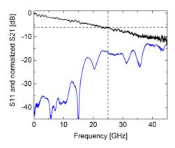
**Fig. 5.9:** EOE frequency response of a 0.4 mm long MZM. In black the normalized S21 parameter is depicted. The 6 dB point of the EOE response corresponds to the 3 dB point of the EO response and is indicated by a dashed line. The bandwidth of the device is measured to be 25 GHz. The S11 stays below 20 dB up to 20 GHz and below 15 dB up to 35 GHz, an indication for a good impedance matching to the 50 Ohm measurement system.
