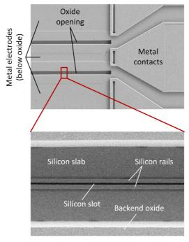
**Fig. 5.7:** SEM images of an SOH MZM. The backend oxide is partially removed, exposing the slot waveguide. Although two mask layers are used to define the slot waveguide, it can be seen in the SEM image that the slot is well centered within the waveguide.
