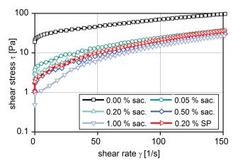
Fig. 6 Influence of sugar (sac.) and superplasticizer (SP) on the flow behaviour of the cement suspensions with a water/cement ratio of 0.5 and 15 min after addition of water at atmospheric pressure and a temperature of 20  $^{\circ}$ C
