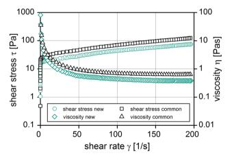
Fig. 10 Shear stress and viscosity over the shear rate of the new mixture (*green*) and the common mixture (*black*)
