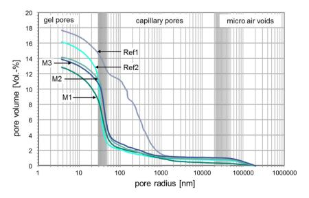
0.05~% and bentonite with 0.5~% by mass of the cement. It shows a high strength and a low porosity with only a small share of capillary pores. By increasing the sand content, the higher cement content due to the lower water/cement-ratio was compensated. Compared to the Indonesian reference mixture, even a reduction of the cement content of 10~% was achieved while maintaining the known workability.
