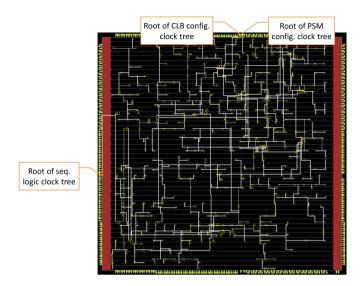
Figure 7.7.: Result of Clock Tree Synthesis (CTS) in inner tile macro of V-FPGA
