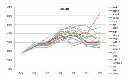
Figure 6.12.: Multi-level Utilization Ratio (MLUR) of MCNC20 benchmarks after technology mapping onto *V-FPGA* for K = 2..8, which is mapped onto Xilinx Virtex-7 underlying platform
