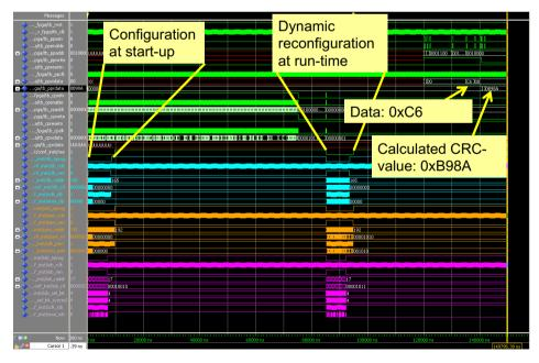
Figure 8.3.: Simulation of dynamic reconfiguration of a *V-FPGA* core that is hosted by an Actel ProASIC3 FPGA
