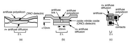
Figure 2.10.: Dielectric anti-fuse technology [11]
