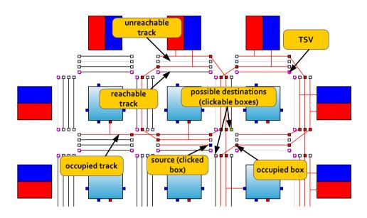
Figure 5.4.: Editing the routing graphically with V-FPGA Explorer
