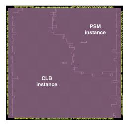
Figure 7.6.: Amoeba view of a placed inner tile macro showing the outlines of CLB and PSM instances
