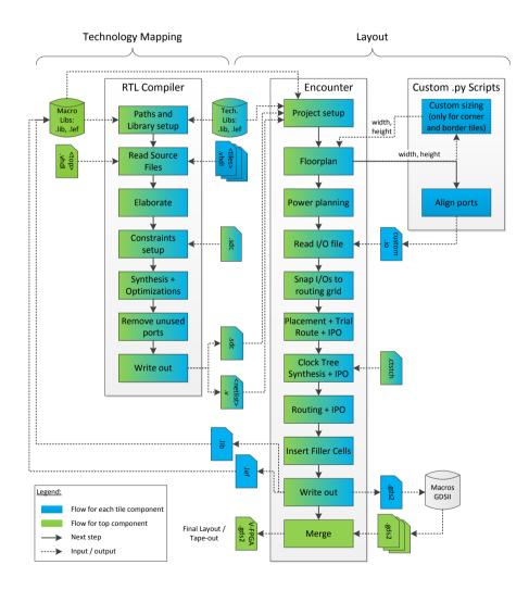
Figure 7.2.: Physical design flow for mapping the V-FPGA onto an ASIC
