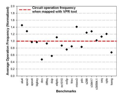
Figure 8.14.: Average operation frequency for multiple benchmark mappings with our framework, normalized to VPR solution [90]
