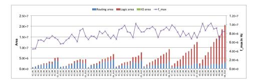
Figure A.4.: Area and performance of *bigkey* benchmark mapped on *V-FPGA* with various LUT and cluster sizes
