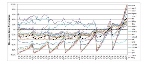
Figure 4.16.: Effects of Lut size *K* and cluster size *N* on area, shown through variance of area relative to median of series for combinations of *K* and *N*
