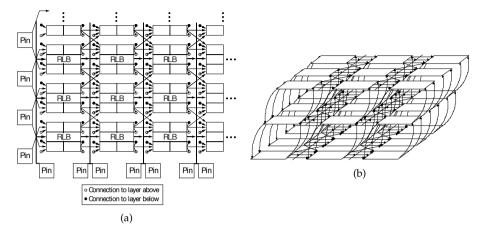
Figure 3.10.: Rothko 3D FPGA [59]: a) routing structure of a layer, b) connectivity between RLBs
