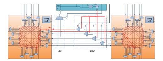
Figure 4.11.: Example of Loopback Propagation in bi-directional tracks
