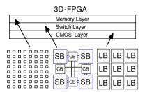
Figure 3.11.: Lin et al.: Monolithically stacked 3D FPGA [61]
