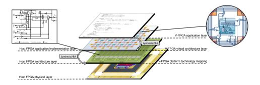
Figure 4.1.: Layer model of the *V-FPGA* approach with island based virtual architecture hosted by an Actel (now Microsemi) COTS FPGA
