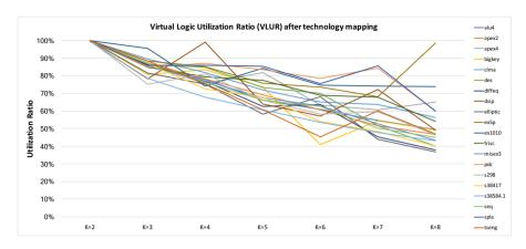
Figure 6.9.: Virtual Logic Utilization Ratio (VLUR) of MCNC20 benchmarks for K = 2..8 after technology mapping
