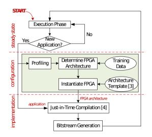
Figure 8.17.: Methodology for supporting self-aware reconfigurable platforms [98]
