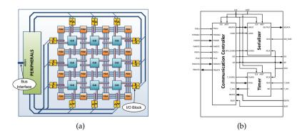
Figure 6.2.: Peripheral unit to connect the *V*-*FPGA* to an AMBA bus: a) mapping to IOBs of the *V*-*FPGA*, b) structure with additional frequently used function units
