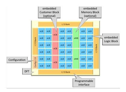
Figure 3.3.: Menta eFPGA Core IP architectural features [71]
