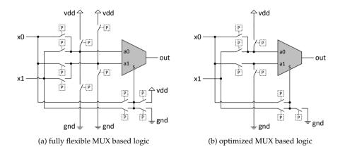
Figure 2.6.: Multiplexer based logic: (a) fully flexible (b) optimized. Both alternatives can implement the same function set (see Table 2.1)
