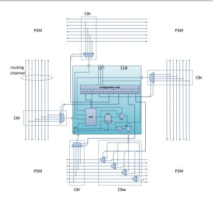
Figure 4.3.: Unclustered CLB with connection boxes
