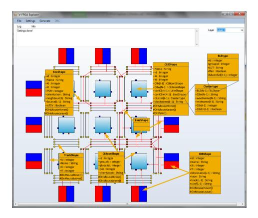
Figure 5.3.: View of object oriented graphical representation in *V-FPGA Explorer* with respective classes and relevant attributes
