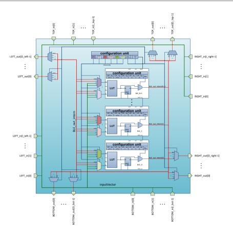
Figure 4.14.: Clustering of BLEs within a CLB of V-FPGA
