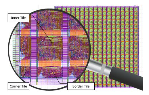
Figure 7.12.: Merged layout of V-FPGA top level and tile macros
