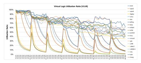
Figure 6.10.: Virtual Logic Utilization Ratio (VLUR) of MCNC20 benchmarks for K = 2..8and N = 1..10 after placement on autosized arrays
