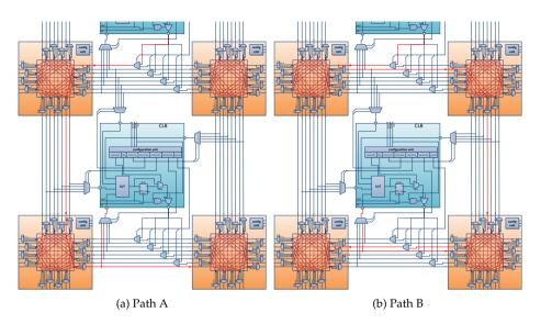
Figure 4.12.: Connection between two CLBs through two different paths
