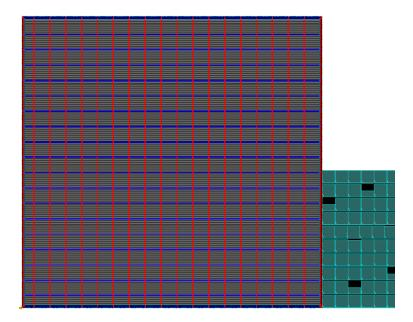
Figure 7.9.: Floor plan of V-FPGA with power rings and power grid
