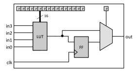
Figure 2.5.: Logic cell containing a LUT, a flip-flop and a bypass MUX, programmable through SRAM cells P
