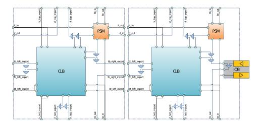
Figure 4.20.: Routing channels within tiles
