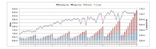
Figure A.20.: Area and performance of *tseng* benchmark mapped on *V-FPGA* with various LUT and cluster sizes
