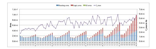
Figure A.9.: Area and performance of *elliptic* benchmark mapped on *V-FPGA* with various LUT and cluster sizes
