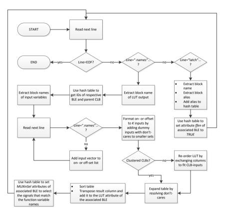
Figure 5.11.: Import of function mapping information in V-FPGA Explorer
