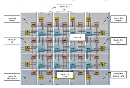
Figure 4.19.: Partitioning of V-FPGA structure into recurring tiles
