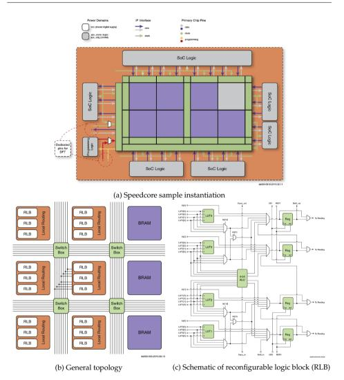
Figure 3.4.: Speedcore eFPGA by Achronix [1] - a) Instantiation in SoC design, b) topology and c) reconfigurable logic block
