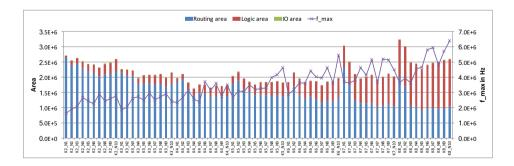
Figure A.19.: Area and performance of *spla* benchmark mapped on *V-FPGA* with various LUT and cluster sizes
