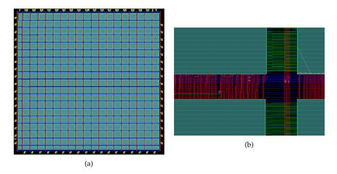
Figure 7.10.: Automated placement of macro tiles in *V-FPGA*: a) array of 19x19 tiles, b) detailed view of inter-tile connections
