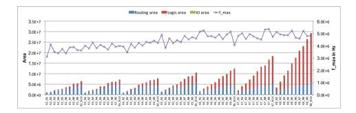
Figure A.6.: Area and performance of *des* benchmark mapped on *V-FPGA* with various LUT and cluster sizes
