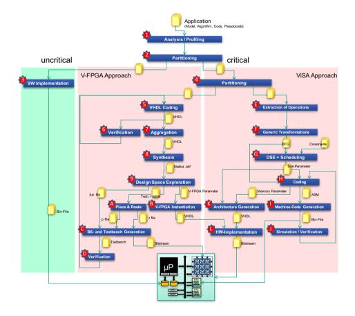
Figure 6.5.: Customization flow for heterogeneous SoC architectures based on the V-FPGA framework
