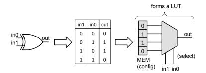
Figure 2.4.: Principle of lookup table (LUT) as programmable logic
