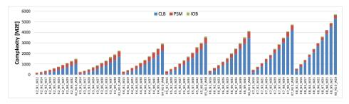
Figure 6.13.: MUX2-equivalent module-level complexity of *V*-*FPGA* for various *K*, *N* and *W* combinations
