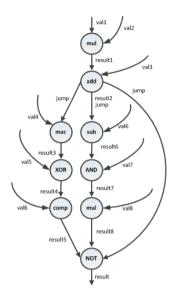
Figure 6.6.: Dataflow graph of an example application scheduled for *ViSA* with all executable operations
