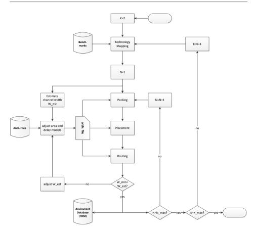
Figure 6.15.: Concept of parametric DSE flow
