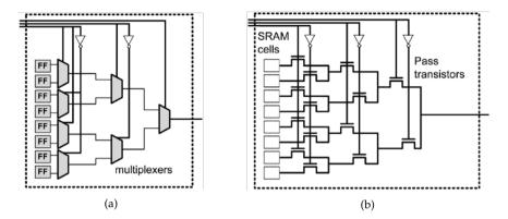
Figure 3.1.: Comparison of a LUT implementation in a) a soft IP core using standard cells and b) a hard IP core [107]
