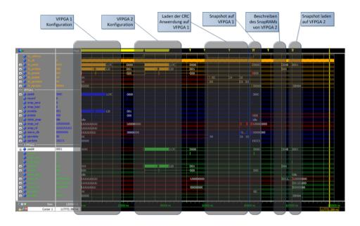
Figure 4.34.: Simulation of a migration of a running application from one *V*-*FPGA* core to another [21]
