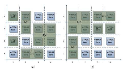
Figure 4.35.: Example of a fragmented *V-FPGA* core array (a) and the result after defragmentation (b) [21]
