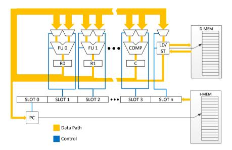
Figure 4.36.: Generic VLIW-inspired Slot Architecture consisting of multiple functional units, registers, multiplexers, a program counter, data and instruction memory
