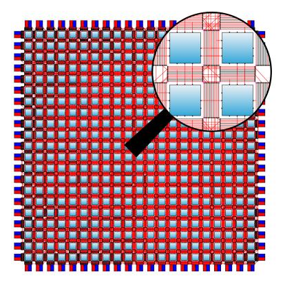
Figure 5.12.: V-FPGA Explorer: Layout of diffeq circuit mapped onto V-FPGA after import from VPR 7
