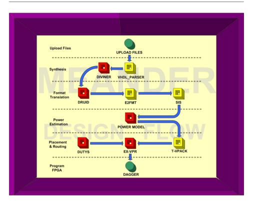
Figure 5.2.: Main screen of GUI-featured MEANDER framework [69]
