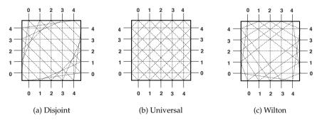
Figure 4.8.: Structure of (a) *Disjoint*, (b) *Universal* and (c) *Wilton* switch block patterns [67]
