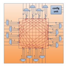
Figure 4.7.: Schematic of PSM in V-FPGA, here with Wilton structure
