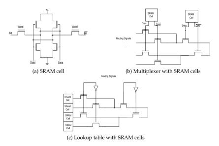
Figure 2.8.: SRAM programming technology [57]
