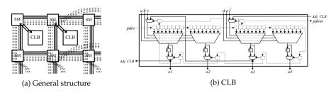
Figure 3.7.: Structure of the virtual FPGA by Lysecky et al. [65]: a) general topology and b) configurable logic block (CLB)
