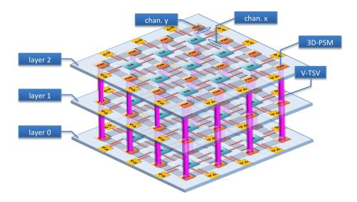
Figure 4.21.: Structure of 3D V-FPGA
