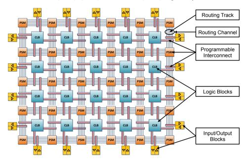
Figure 4.2.: Structure of V-FPGA
