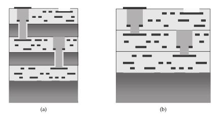
Figure 2.14.: Illustration of through via 3D technology: (a) bulk, (b) silicon on insulator [28]
