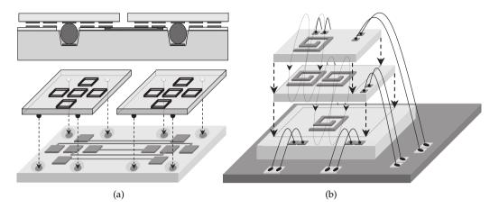
Figure 2.15.: Illustration of contactless 3D technology: (a) capacitive, (b) inductive [28]
