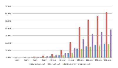
Figure 8.10.: Resource utilization of ViSA manycore on Xilinx Virtex-6
