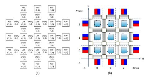
Figure 5.8.: Difference between coordinate systems in (a) VPR and (b) V-FPGA Explorer
