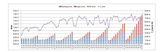
Figure A.17.: Area and performance of *s38584.1* benchmark mapped on *V-FPGA* with various LUT and cluster sizes
