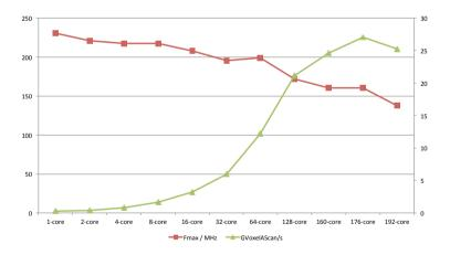
Figure 8.12.: Maximum frequency and throughput of *ViSA* manycore on Xilinx Virtex6. The optimum configuration contains 176 *ViSA* cores at a maximum frequency of 160.4 *MHz*, which gives a peak performance of up to 27.0 *GigaVoxelAScans/s*.
