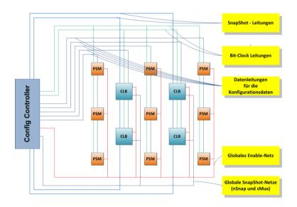
Figure 4.33.: Snapshot net in V-FPGA [21]
