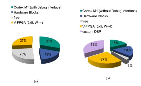
Figure 8.2.: Resource utilization for implementing the hetorogeneous reconfigurable SoC on an Actel M1A3P1000 device: (a) SoC with microprocessor, debug unit and *V-FPGA*, (b) SoC with microprocessor, *V-FPGA* and custom DSP
