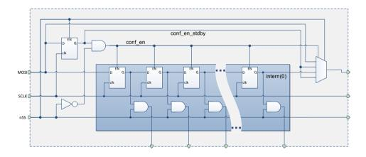
Figure 4.30.: Configuration unit with by-pass selector logic for enabling slice-level partial reconfiguration in *V-FPGA*
