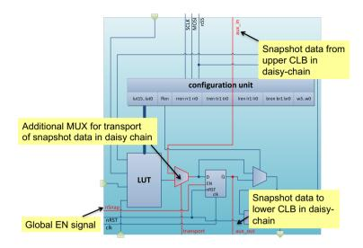
Figure 4.32.: Snapshot mechanisms in V-FPGA [35]
