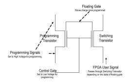
Figure 2.9.: Flash programming technology [57]
