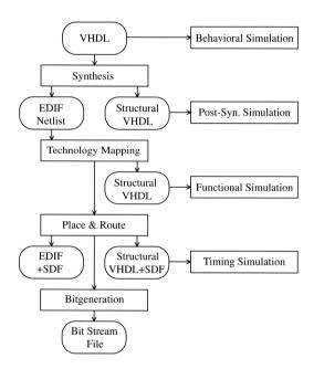
Figure 2.16.: Design flow for FPGAs [53]
