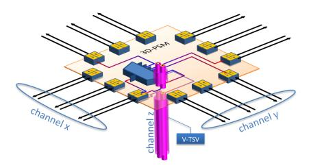
Figure 4.22.: Simplified scheme of 3D-PSM in V-FPGA
