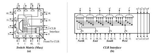
Figure 3.9.: Lysecky et al.: schematic of a multiplexor based switch matrix (MSM) [65]
