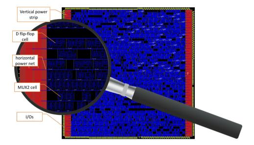
Figure 7.5.: Standard cell placement of V-FPGA inner tile macro in a 45 nm ASIC process
