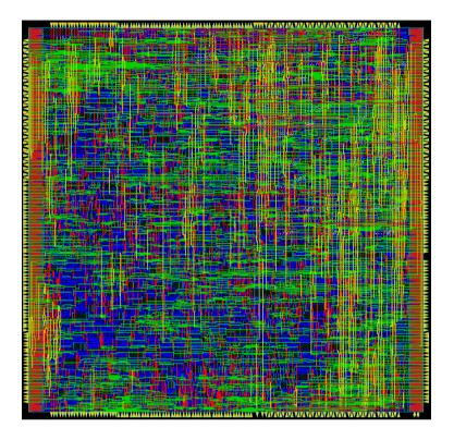
Figure 7.8.: Layout of V-FPGA inner tile macro after routing
