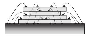
Figure 2.12.: Illustration of wire bonded 3D technology [28]
