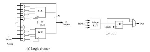
Figure 4.13.: General structure of a logic cluster combining a collection of basic logic elements (BLE) that are flexibly interconnected by multiplexers [13]
