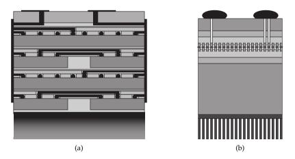
Figure 2.13.: Illustration of microbump 3D technology: (a) 3D package, (b) face-to-face [28]
