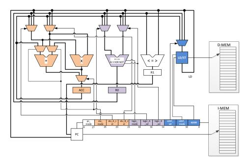
Figure 8.5.: Ultra low power VLIW-inspired Slot Architecture for measuring chains in process automation implementing a program counter, a MAC unit, a logic and a load/store slot
