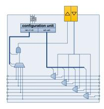
Figure 4.6.: Schematic of I/O block in V-FPGA
