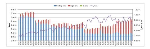
Figure A.16.: Area and performance of *s38417* benchmark mapped on *V-FPGA* with various LUT and cluster sizes
