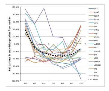
Figure 4.5.: Effects of LUT size *K* on area-delay product, shown through variance relative to medians of series within the range K=2..8
