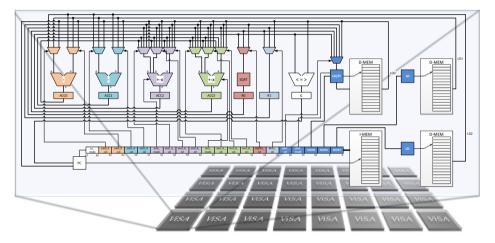
Figure 8.9.: VLIW-inspired Slot Architecture for high performance medical imaging implementing a program counter, several arithmetic and logic slots as well as a load/store slot. *ViSA* is realized as a homogeneous multicore system.
