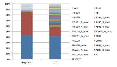
Figure 8.11.: Relative module level resource utilization on Xilinx Virtex-6. The square root unit (SQRT0) is the unit with the most resources, followed by the NoC inter-face (NI).
