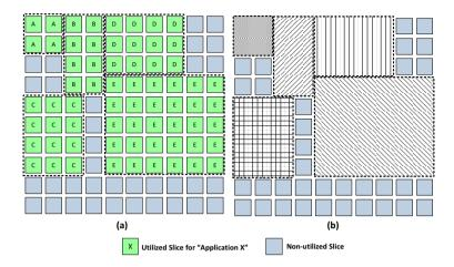
Figure 5.15.: Fragmentation problem introduced by typical task allocation: a) example allocation, b) respective area blockages [92]
