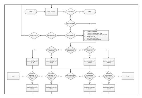
Figure 5.9.: Import of global routing information in V-FPGA Explorer
