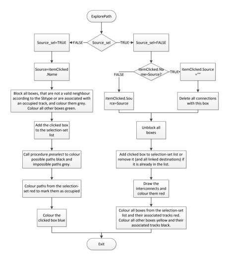
Figure 5.5.: Flow chart of ExplorePath algorithm in V-FPGA Explorer
