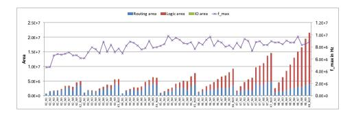
Figure A.8.: Area and performance of *dsip* benchmark mapped on *V-FPGA* with various LUT and cluster sizes
