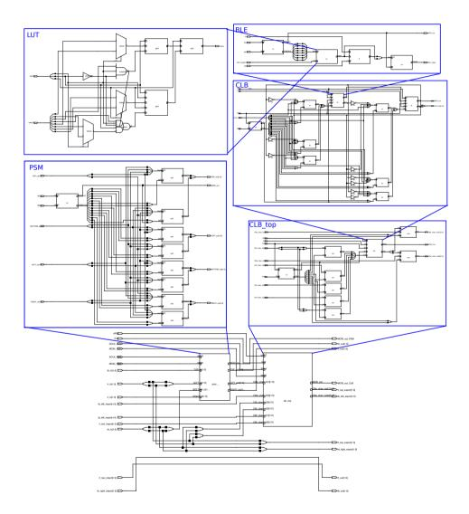
Figure 7.3.: Hierarchical schematic of a tile component after synthesis with RTL Compiler
