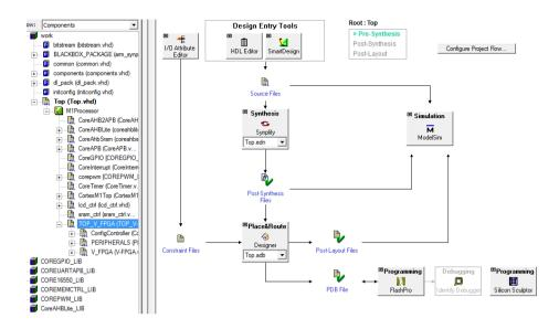
Figure 7.1.: Toolflow for mapping V-FPGA onto an Actel/Microsemi COTS FPGA
