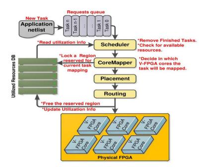
Figure 8.13.: Methodology for application mapping onto V-FPGA cores [90]
