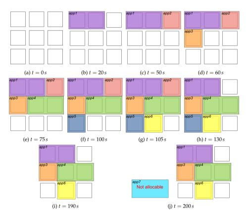
Figure 4.31.: Fragmentation scenario in runtime partial reconfigurable architectures
