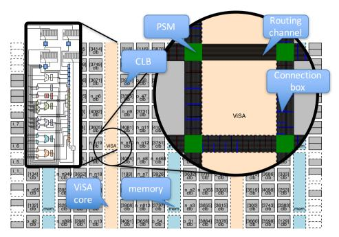
Figure 4.38.: Structure of ViSA and V-FPGA Integrated System (ViSA-VIS) with CLBs and ViSA cores aranged face-to-face in the V-FPGA
