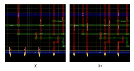
Figure 7.4.: Routability in user defined alignment of I/Os: a) locations as defined, b) after snapping to routing grid
