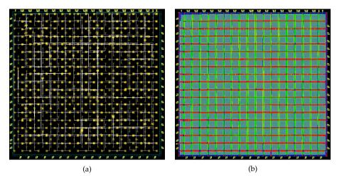
Figure 7.11.: a) Clock trees in V-FPGA, b) layout with abstract tile macros after routing
