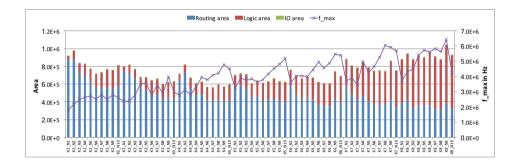
Figure A.15.: Area and performance of *s298* benchmark mapped on *V-FPGA* with various LUT and cluster sizes
