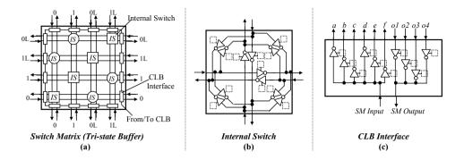
Figure 3.8.: Lysecky et al.: schematic of a tristate-buffer based switch matrix (TSM) [65]
