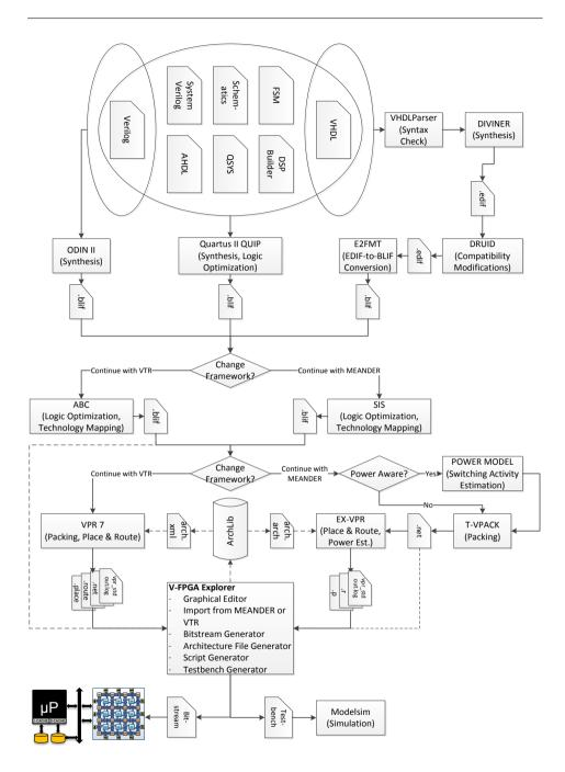
Figure 5.1.: Tool-flow for application mapping onto V-FPGA
