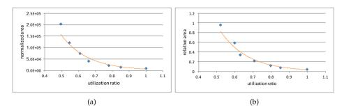
Figure 6.8.: Relationship between logic area and utilization ratio for (a) *alu4* circuit and (b) for the average over MCNC20 benchmark set
