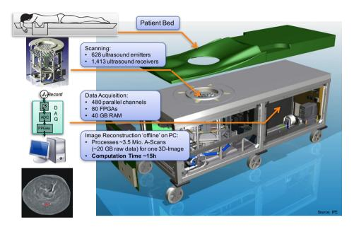
Figure 8.7.: Setup of 3D Ultrasound Computer Tomography for breast cancer detection
