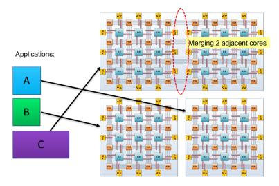
Figure 4.28.: The CoreFusion idea, merging adjacent V-FPGA cores [35]
