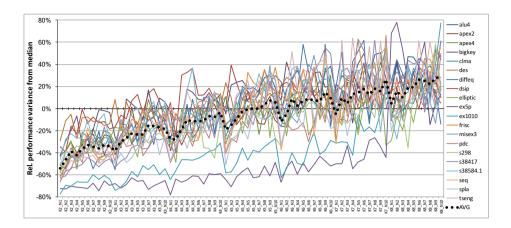
Figure 4.17.: Effects of LUT size K and cluster size N on performance, shown through variance of performance relative to median of series for combinations of K and N
