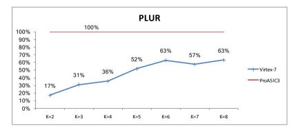
Figure 6.11.: Platform Logic Utilization Ratio (PLUR) on Actel ProASIC3 and Xilinx Virtex-7 for K = 2..8
