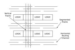
Figure 2.2.: Row-based FPGA topology [10]
