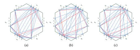
Figure 4.23.: 3D-PSM connectivity patterns based on (a) 2D Disjoint, (b) 2D Universal and (c) 2D Wilton origin horizontal patterns
