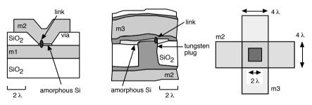
Figure 2.11.: Metal-to-metal anti-fuse technology [11]
