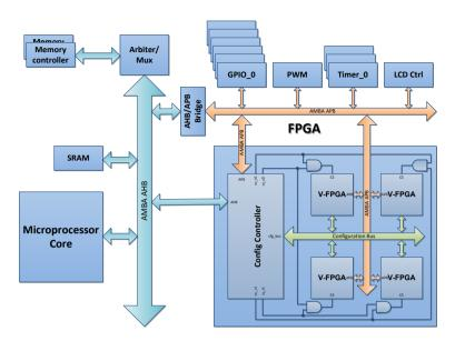
Figure 8.1.: Schematic view of the heterogenous SoC architecture with embedded V-FPGA cores
