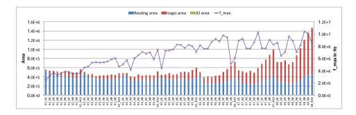
Figure A.7.: Area and performance of *diffeq* benchmark mapped on *V-FPGA* with various LUT and cluster sizes
