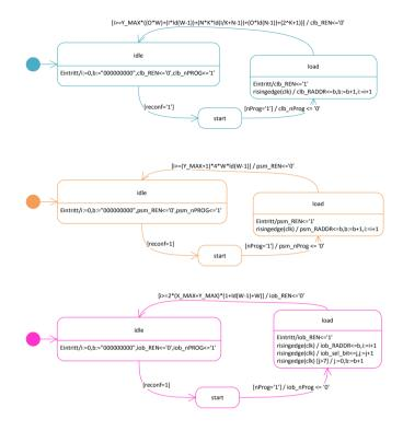
Figure 4.25.: Finite State Machines of bitstream loader
