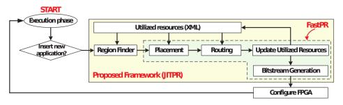
Figure 5.16.: JIT compilation framework for performing fast application implementation onto FPGA devices [92]
