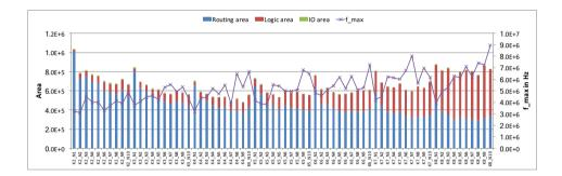
Figure A.3.: Area and performance of *apex4* benchmark mapped on *V-FPGA* with various LUT and cluster sizes
