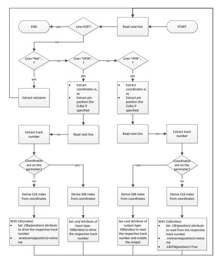
Figure 5.10.: Import of local routing information in V-FPGA Explorer
