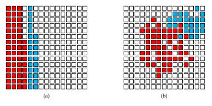
Figure 4.29.: PR regions and the effects on placement: (a) rectangular regions in framegranular PR, (b) free-form in fine-grained slice-level PR
