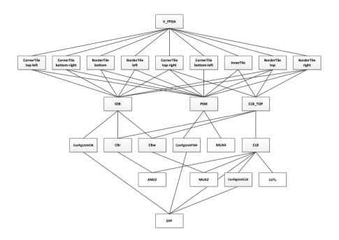
Figure 4.18.: Hierarchy of V-FPGA components and subcomponents
