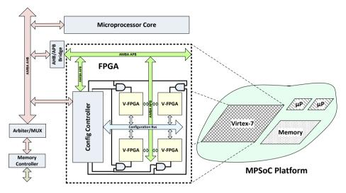
Figure 8.16.: System architecture of the self-aware platform
