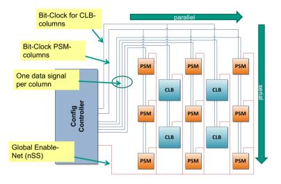
Figure 4.27.: Semi-parallel configuration infrastructure in V-FPGA
