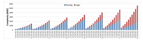
Figure 6.14.: Logic vs. routing complexity of V-FPGA expressed in MUX2-equivalents
