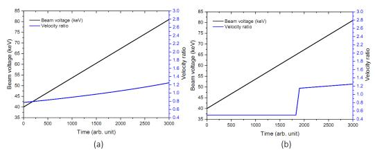
Fig. 1.5.5: Comparison of (a) diode type and (b) triode-type start-up scenarios.
