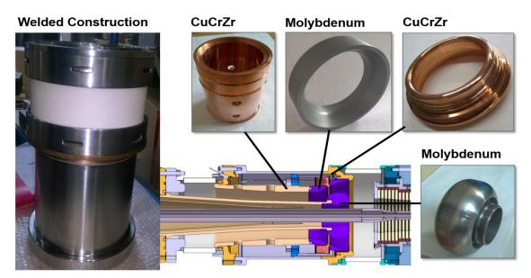
Fig. 1.4.1: 3D sketch of the Inverse Magnetron Injection Gun (IMIG) and the already manufactured subcomponents.
