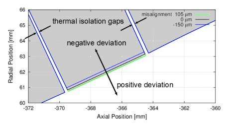
Fig. 1.4.4: Definition of the emitter deviation and representation of the thermal isolation gaps.
