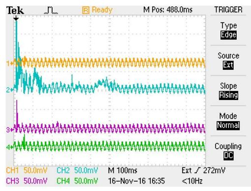
Fig. 1.2.29: Decay of the parasitic signal (blue) in the filter-bank after 300 msec.
