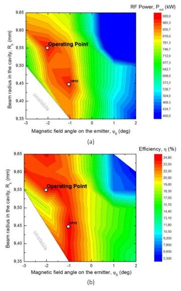
Fig. 1.2.9: (a) Generated RF power and (b) Efficiency with the magnetic field angle  $\phi_B$  and the beam radius  $R_b$  in the cavity.
