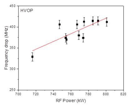
Fig. 1.2.33: Frequency drop with respect to the generated RF power at the HVOP.
