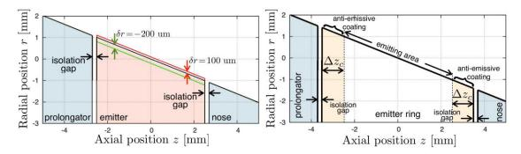
Fig. 1.3.2: Conventional (left) and the proposed type (right) of emitter ring which significantly decrease the sensitivity in the manufacturing tolerances.
