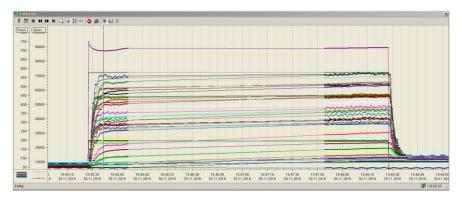
Fig. 1.2.22: Collector's thermocouple temperature and Ibeam during a 180 sec pulse.
