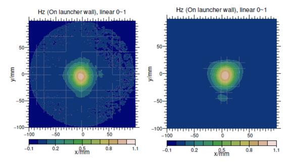
Fig. 1.3.4: The field distribution at 0.25 m away from the gyrotron window: experiment (left) and simulation (right).
