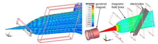
Fig. 1.5.7: Transformation of elliptic beam.
