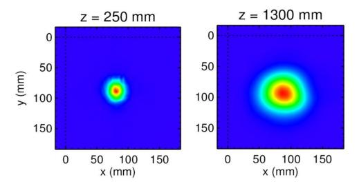
**Fig. 1.2.16.** Thermographic images from the microwave output beam of the gyrotron recorded on a PVC-target at different distances z from the gyrotron window.
