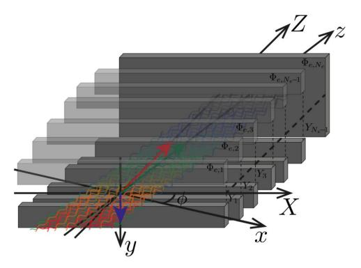
Fig. 1.3.1: Conceptual drawing of the proposed multistage depressed collector for sheet electron beam.
