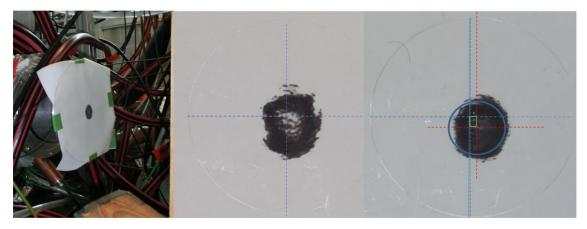
Fig. 1.2.14: Preliminary results of the beam profile measurements at the output window achieved with thermal paper.
