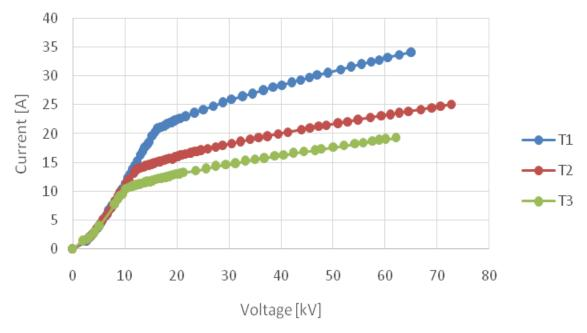
Fig. 1.2.7: Emitted current vs. accelerating voltage for three different temperatures of the emitter (T1>T2>T3).
