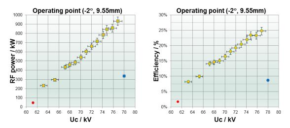
Fig. 1.2.11: RF generated power and efficiency vs. accelerating voltage achieved at LVOP with the beam current ~48 A.
