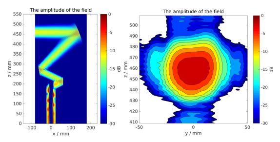
Fig. 1.3.5: Simulated electric field of the QO system for the W7-X gyrotron, in the x-z-plane (left) and at the output window (right).
