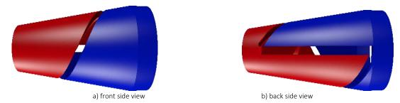
Fig. 1.5.9: Two stages separated by a conical helix slot for the E×B drift.
