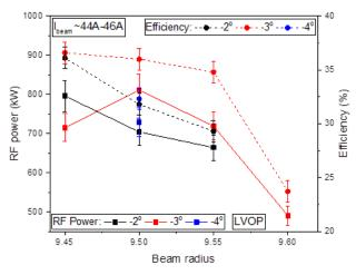
**Fig. 1.2.25:** RF Power and corresponding overall efficiency with respect to the beam radius and with the orientation of the magnetic field lines at the emitter as a parameter. Operation only at the LVOP.
