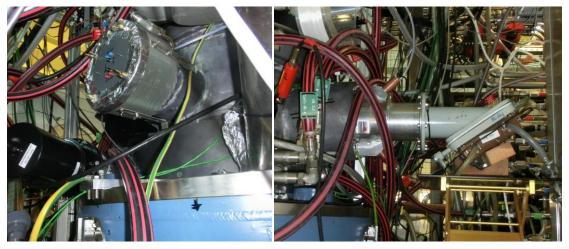
Fig. 1.2.8: Bolometer (stray radiation level monitoring) (left) and flow-calorimeter (measurement of the output power) (right).
