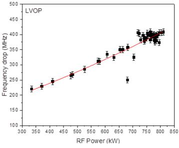
Fig. 1.2 28: Frequency drop with respect to the generated RF power.
