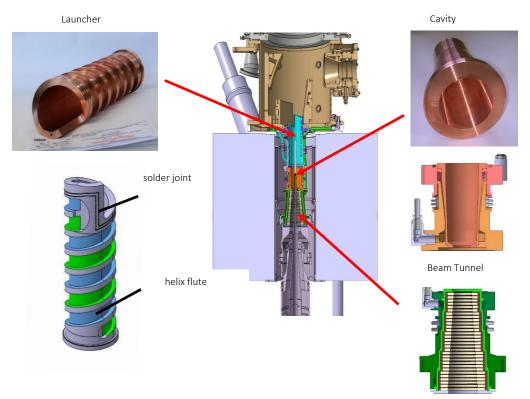
Fig. 1.5.2: Manufactured subcomponents of the coaxial long pulse gyrotron.
