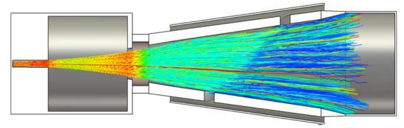
Fig. 1.5.10: Simulation of a two-stage collector with helixal slot.
