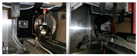
Fig. 1.2.15: Arrangement of the IR beam profile measurement setup.
