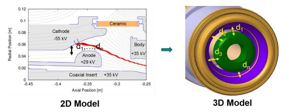
Fig. 1.4.2: Transformation procedure of the 2D into 3D model.
