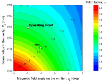
Fig. 1.2.10: Simulated Electron beam pitch factor
