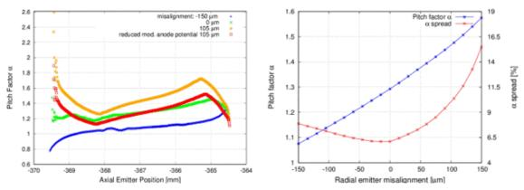
**Fig. 1.4.5:** Left: Pitch factor at the cavity as a function of the emitting point along the emitter surface for different radial misalignments. Right: Pitch factor and RMS α spread at the cavity center, regarding the radial misalignment
