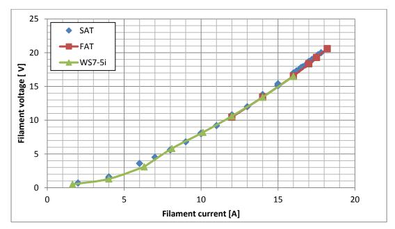
Fig. 1.2.6: Filament current vs. filament voltage (SAT) as comparison with the FAT and W7-X SN5i gyrotron results.
