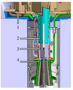
**Fig. 1.5.1:** Overview of the proposed cooling system for the most critical gyrotron subcomponents (1-mirror box, 2-launcher, 3-cavity, 4-beam tunnel).
