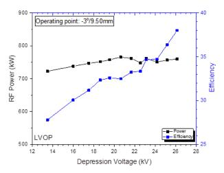
Fig. 1.2.26: RF power and corresponding overall efficiency with respect to the depression voltage for the LVOP.
