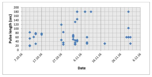
Fig. 1.2.20: Evolution of the pulse length achieved during the conditioning of the tube with RF.
