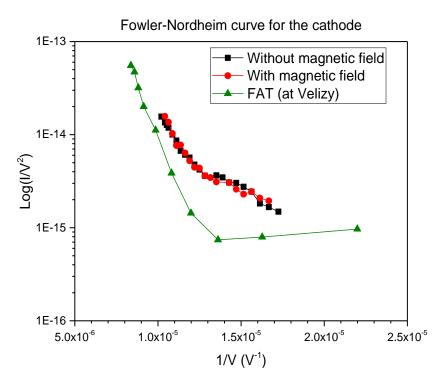
Fig. 1.2.4: Fowler-Nordheim diagram with the cathode on high voltage and the body grounded (maximum voltage applied 96 kV).
