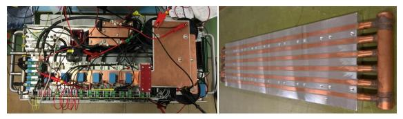
Fig. 1.6.3. Power module and cooling unit.
