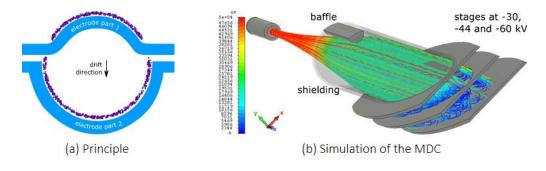
Fig. 1.5.8: Split a circular electron beam to semi-circular sheet beams.
