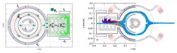
Fig. 1.5.6: Left: The previous E×B concept. Right: Beam thickness before and after optimizations.
