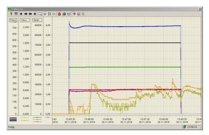
**Fig. 1.2.21:** 180 sec pulse achieved during the experiments. In the figure it is visible the beam current (blue), the accelerating voltage (black), the cathode voltage (green), the depression voltage (red), the vacuum reaction (yellow) and the mode-loss diode signal (magenta).
