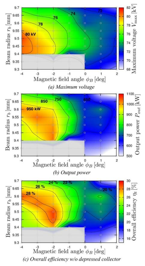
Fig. 1.3.3: Operational maps of the short-pulse prototype of the 1 MW Gyrotron.
