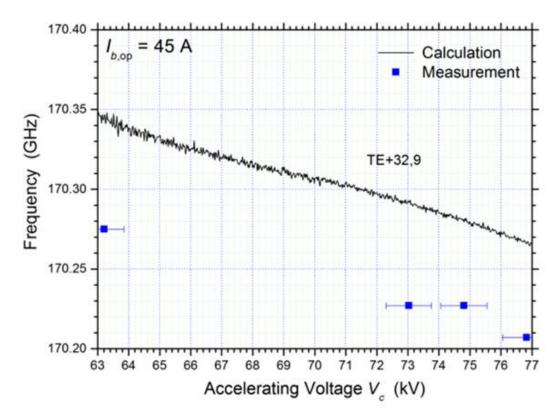
Fig. 1.2.13: Dependency of the gyrotron output frequency on accelerating voltage.
