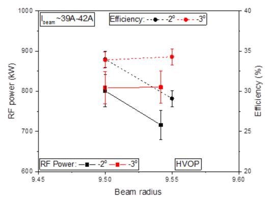
Fig. 1.2.32: RF power and corresponding efficiency at different operating parameters at the HVOP.
