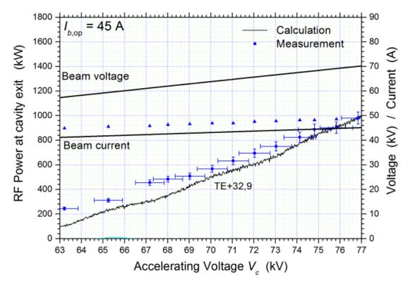
Fig. 1.2.12: Generated power vs. the beam voltage and comparison with simulated results from the code suite EURIDICE.
