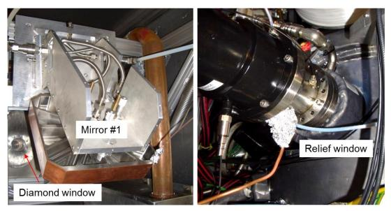
Fig. 1.2.19: Diagnostics installed inside the microwave box and at the relief window.
