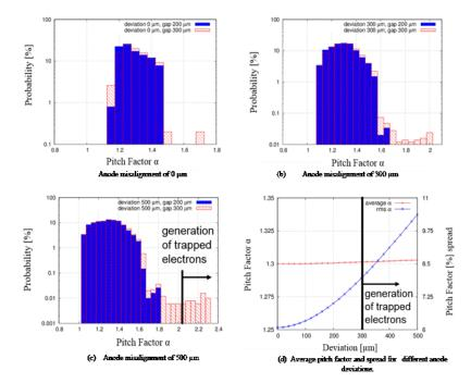
**Fig. 1.4.3:** Pitch factor distribution for different anode misalignments (a-c) with a gap width of 200  $\mu$ m (nominal case, blue colored) and 300  $\mu$ m (red colored), (d) describes the average pitch factor and spread for anode deviations in the range of 0  $\mu$ m to 500  $\mu$ m with a gap width of 200  $\mu$ m.
