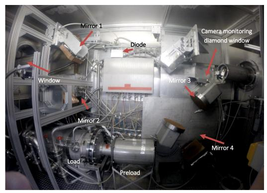
Fig. 1.2.17: Microwave box prepared for CW operation of the gyrotron.
