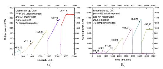
Fig. 1.5.4: Multi-mode, self-consistent, diode start-up analysis for (a) DM5 and (b) DM7 mode.
