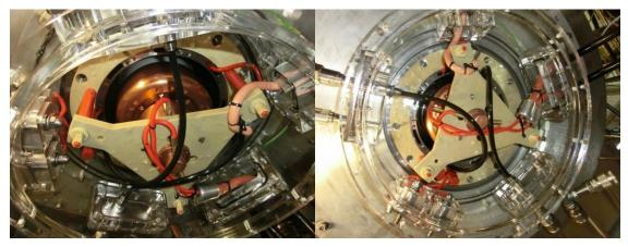
Fig. 1.2.3: Oil tank after installation of HV, electrical connections and cooling pipes.
