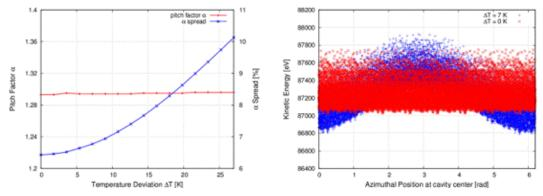
Fig. 1.4.6: Left: Pitch factor and RMS  $\alpha$  spread simulated at the cavity center for different temperature deviations. Right: Kinetic energy as function of the azimuthal position at the cavity center for emitter temperature deviations of 7 K (blue points) and 0 K (red points).
