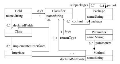
**Figure 6.2.:** Class diagram showing a metamodel for object-oriented designs that is simplified as needed for our running example
