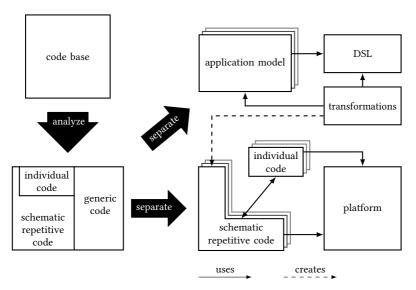
**Figure 2.1.:** Process for the development of a DSL based on an application code that was developed without the DSL, adapted from [VS06, p. 15]
