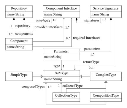
**Figure 6.1.:** Class diagram showing a simplified metamodel for models of componentbased software architectures
