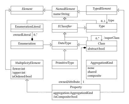
**Figure 2.2.:** Simplified class diagram showing central metaclasses of the EMOF metamodelling language [ISO14, p.27] (dotted lines denote indirect inheritance)
