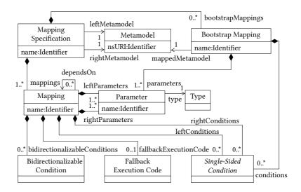
**Figure 7.1.:** Simplified class diagram with central metaclasses for representing mappings as an AST
