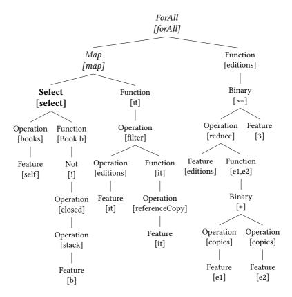
**Figure 8.4.:** Illustration of the custom expression tree obtained for the complete example invariant (matched iterator printed in bold, parents of it in italics)
