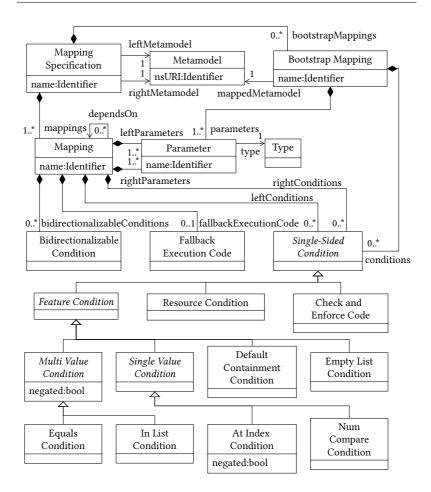
**Figure 7.9.:** Simplified class diagram with metaclasses for completely representing mappings as an AST
