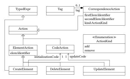
**Figure 6.6.:** Simplified class diagram for metaclasses for representing actions of the consistency preservation reactions language in an AST
