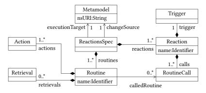
**Figure 6.3.:** Simplified class diagram with central metaclasses for representing consistency preservation reactions in an AST
