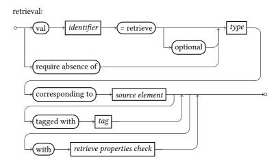
**Figure 6.5.:** Syntax diagram showing all possible correspondence retrievals that can be given in a match block
