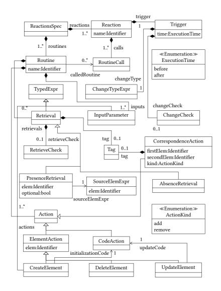
**Figure 6.8.:** Simplified class diagram with metaclasses for completely representing reactions in terms of an AST
