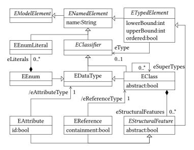
**Figure 2.3.:** Simplified class diagram showing central metaclasses of the Ecore metamodelling language according to [Ste+08, pp.97] and [Bur14, p.25]
