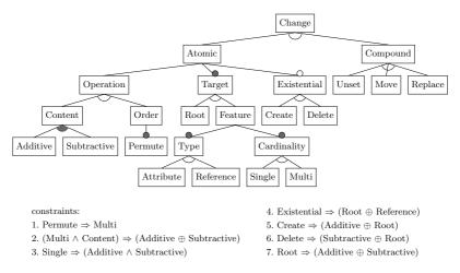
**Figure 5.3.:** Feature model for all changes in Ecore-based models that require different information or information of different types
