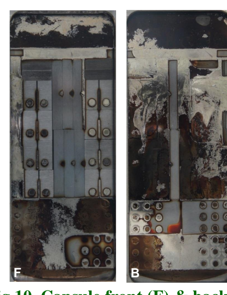
Fig.10. Capsule front (F) & back (B) views after cooling to RT.
