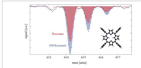
**Figure 2.** Isotope-selective interference contrast of TPP: the normalized signal difference is  $S_N = -0.293(3)$  for the isotopically pure TPP (614 amu),  $S_N = -0.289(3)$  for the next fermion (615 amu) and  $S_N = -0.290(3)$  for the 616 amu isotopomer. The normalized signal difference is computed from the area associated with each mass, using a Gaussian multi-peak fit (continuous lines). All  $S_N$  values are identical within the error bar of 1%.
