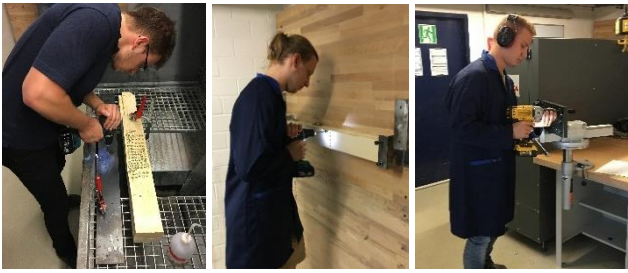
Fig. 2. Performing of different test-cases for screwdrivers (left, middle) and impact wrenches (right) at IPEK – Power-Tool Test center
