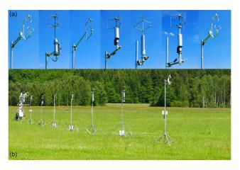
**Figure 2.** (a) Close-up pictures of all seven sonic anemometers; they are presented from left to right in the same order as they are listed in Table 1. (b) A photograph of the field intercomparison experiment; the micrometeorological installations of the TERENO/ICOS site DE-Fen can be seen in the background (left).
