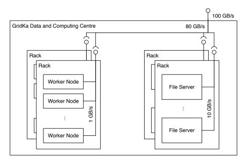
Figure 2.5.: Simplified network diagram of the GridKa data and computing centre. Worker nodes within a rack rely on 1 Gbit/s data transfer rates whereas inter rack communication and communication to file servers allows for 10 Gbit/s up to 80 Gbit/s. The GridKa also provides dedicated links with up to 100 Gbit/s, for example, to Tier 0.
