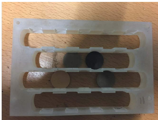
Figure 4 Three-dimensional printed sample holder.
