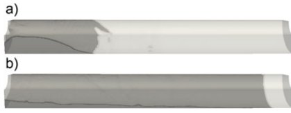
Figure 6. Comparison of the sediment buildup of (a) a poor-flowing and (b) an easy-flowing sediment after a simulation time of 50 s. Process and material parameters are kept constant, except the flow behavior.
