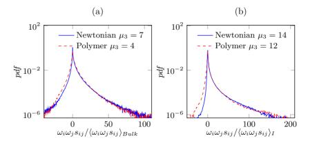
Figure 5.18: Probability density function of the enstrophy production  $\omega_i \omega_j s_{ij}$  normalized by its average value. (a) in the bulk (b) at the interface,  $\mu_3$  is the estimated skewness of the distribution. Adapted from [14].
