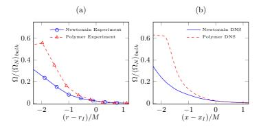
Figure 4.9: Average profiles of enstrophy as a function of the distance from the average position for the experiments (a) and for the simulations (b). The quantities have been normalized by the average enstrophy of the bulk for the Newtonian case.
