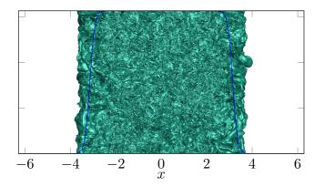
Figure 2.2: The smoothing function from Equation 2.4 superimposed over plotted iso-surfaces of the enstrophy field.
