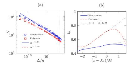
Figure 4.11: (a) Number of boxes *N* containing portion of the interface against box size  $\Delta/\eta$ . The dotted line marks the box of size  $\Delta = M$ . (b) Integral length scale as a function of the distance from the interface.
