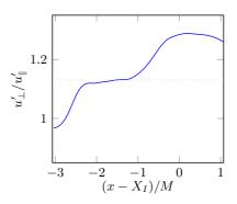
Figure 4.6: Anisotropy in the magnitude of velocity fluctuations as a function of the distance from the average interface position.
