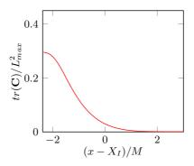
Figure 5.3: Average trace of the conformation tensor normalized by the maximum allowed extension  $L_{max}^2$  as a function of the distance from the average interface position.
