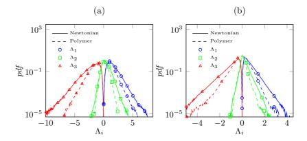
Figure 5.13: Probability density function of the strain eigenvalues  $\Lambda_i$  (a) in the bulk and (b) at the interface. Adapted from [14].
