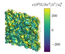
Figure 2.11: Viscous diffusion of enstrophy in a 2D cross-section of the turbulent/non-turbulent interface. Adapted from [12].
