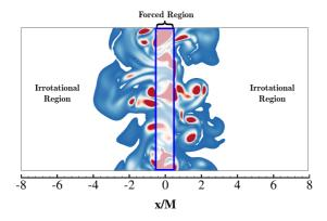
Figure 4.2: Depiction of the computational box with a slice of the enstrophy isocontour for a Newtonian simulation. Adapted from [14].
