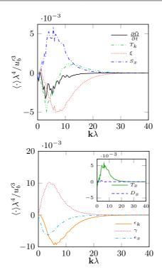
Figure 2.9: Spectral enstrophy budget within the inhomogeneous layer at  $(x - X_I)/\lambda = -2$  where the peak of enstrophy source due to the spatial flux takes place. The terms of Equation (2.8) are shown in (a) while the different components of  $\xi$  and  $S_x$  from Equation (2.7) are delineated in (b). Adapted from [12].
