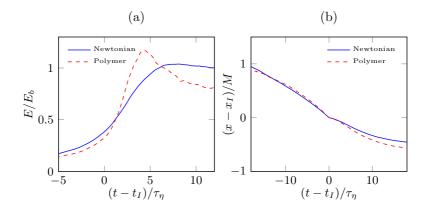
Figure 5.22: Conditional averages in time of entrainment events with respect to the distance from the interface crossing. Energy normalized by the energy in the bulk.
