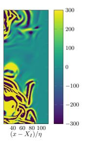
Figure 2.12: Viscous diffusion field in a cross-section of the flow.
