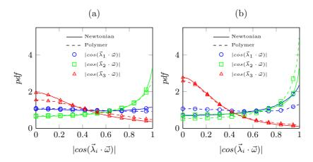
Figure 5.14: Probability density function of the cosine of the angle between the vorticity vector and the three strain eigenvector  $\vec{\lambda}_i$ . (a) in the bulk, (b) at the interface. Adapted from [14].
