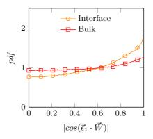
Figure 5.17: Probability density function of the cosine of the angle between the largest conformation tensor eigenvector  $\vec{\epsilon}_1$  and the vortex stretching vector  $\vec{W} = \{\omega_j s_{ij}\}$ .
