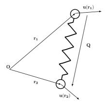
Figure 3.3: Single dumbbell model constituted of two beads linked by an elastic force.
