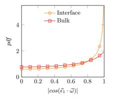
Figure 5.16: Probability density function of the cosine of the angle between the largest conformation tensor eigenvector  $\vec{\epsilon}_1$  and the vorticity vector. Adapted from [14].
