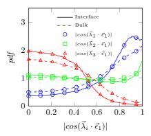
Figure 5.15: Probability density function of the cosine of the angle between the largest conformation tensor eigenvector  $\vec{\epsilon}_1$  and the three strain eigenvector  $\vec{\lambda}_i$ . (a) in the bulk, (b) at the interface. Adapted from [14].
