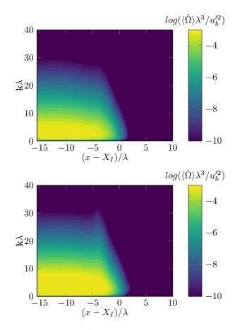
Figure 2.6: Isocontours of  $log(\langle \hat{\Omega} \rangle \lambda^3 / u_b^{\prime 2})$  in the  $(k, x - X_I)$ -space for (a)  $t/t_0 = 4.5$  and (b)  $t/t_0 = 8$ . Adapted from [12].
