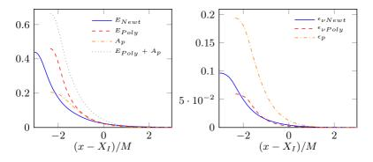
Figure 5.4: (a) Average profiles of kinetic energy and free energy of the polymers.(b) Viscous and polymer dissipation rates. Both as a function of the distance from the average interface position.
