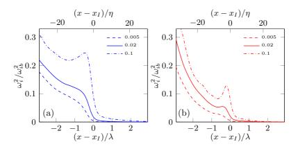
Figure 5.7: Conditional enstrophy profiles normalised by the average enstrophy in the bulk for three different thresholds  $\omega_{i,th}^2 = 0.1 - 0.02 - 0.005 \omega_{i,b}^2$ . (a) Newtonian case, (b) polymers.
