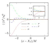
Figure 5.5: Enstrophy budget for the Newtonian case. The right scale refers to  $f_m$ , i.e. the maximum possible amplitude of the body force.
