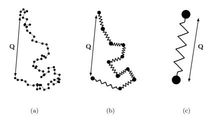
Figure 3.2: Various degrees of simplification of the polymer model with its endto-end vector Q. (a) Multi chain dumbbell model with rigid connectors between the beads. (b) Multi-chain dumbbell model with elastic connectors. (c) Single elastic dumbbell model.
