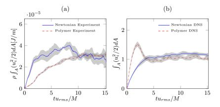
Figure 4.7: Time variation of the integral of the kinetic energy contained in the region between the bulk and the interface. Gray areas mark  $\pm 1.96$  standard errors of the mean. Adapted from [14].
