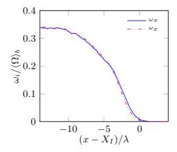
Figure 2.4: Average magnitude of the vorticity components  $\omega_p$  in the homogeneous plane and  $\omega_x$  normal to it as a function of the distance from the average interface position. The value are normalized by  $\langle \Omega \rangle_b$  the average magnitude of the total vorticity in the bulk. Adapted from [12].
