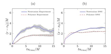
Figure 4.8: Time variation of the average interface position for Newtonian fluid and the dilute polymer solution, comparison between simulation and experimental measurements. The left *y*-axis refers to the experiments while the right one to the simulations. Grey areas mark  $\pm 1.96$  standard errors of the mean. Adapted from [14].
