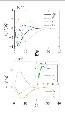
Figure 2.7: Spectral enstrophy budget within the bulk turbulent region for  $t/t_0 =$  4.3. The terms of Equation (2.8) are shown in (a) while the different components of  $\xi$  and  $S_x$  from Equation (2.7) are delineated in (b). Adapted from [12].
