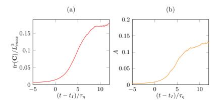
Figure 5.24: Conditional averages in time of entrainment events with respect to the distance from the interface crossing. (a) polymer extension normalized by average extension in the bulk, (b) free energy  $A_p$ .
