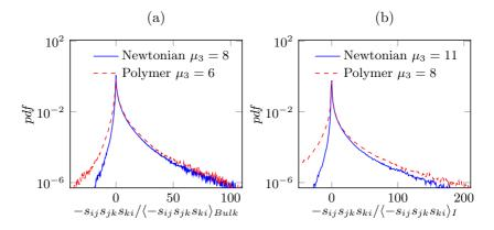
Figure 5.20: Probability density function of the normalized strain rate production  $s_{ij}s_{jk}s_{ki}$  normalized by its average value. (a) in the bulk (b) at the interface,  $\mu_3$  is the estimated skewness of the distribution. Adapted from [14].
