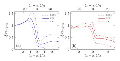
Figure 5.10: Condtional averages of the ratio  $\omega_i^2/2s_{ij}s_{ij}$  for three different thresholds  $\omega_{i,th}^2 = 0.1 - 0.02 - 0.005\omega_{i,b}^2$ . (a) Newtonian case, (b) polymers.
