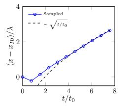
Figure 2.3: Average interface position with respect to time.  $x_{I0}$  denotes the position of the interface at the beginning of the decay. Adapted from [12].
