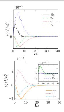
Figure 2.10: Spectral enstrophy budget within the interfacial layer at  $(x-X_I)/\lambda = 0$  for  $t/t_0 = 4.3$ . The terms of Equation (2.8) are shown in (a) while the different components of  $\xi$  and  $S_x$  from Equation (2.7) are delineated in (b). Adapted from [12].
