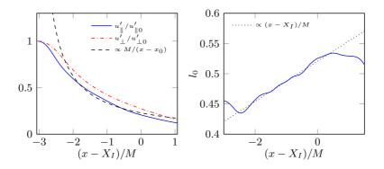
Figure 4.5: (a) Profiles of the magnitude of velocity fluctuations in the direction parallel to the homogeneous planes y - z and normal to them as a function of the distance from the average interface position. The black dashed line represent the fit with a function inversely proportional to the distance from a virtual origin in the forced region. (b) Variation of the integral length scale as a function of the distance from the average interface position.
