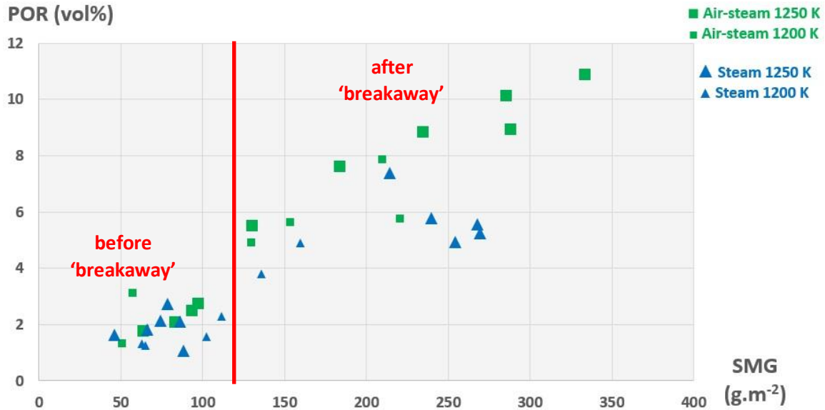
Figure 6: POR (vol%) of ZIRLO® samples corroded under pure steam or in the 50-50mol% air-steam mixture, at 1200 or 1250 K, as a function of the SMG ( \text{g}\cdot\text{m}^{-2} )
