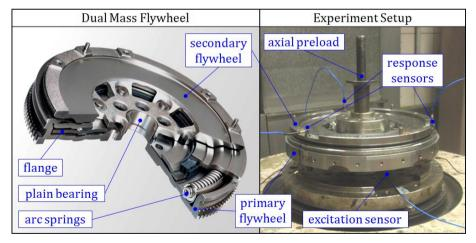
**Figure 5.1:** Basic components of a dual mass flywheel (left, source: http://blog.motoringassist.com/ motoring-advice/wp-content/uploads/2013/12 /dual .jpg, Accessed: 3rd March 2016). The experiment setup on the shaker platform (right) with adjustable axial preload of the secondary flywheel.
