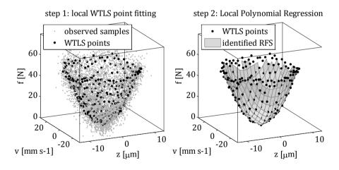
**Figure 2.17:** The two steps of the presented nonparametric surface fitting approach based on the synthetic correlated noisy samples of a paraboloid RFS. Intermediate samples are generated using local WTLS point fitting (left). The intermediate samples are then used in a subsequential quadratic Local Polynomial Regression (right).
