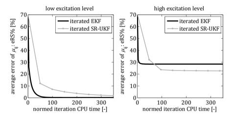
**Figure 4.6:** Average estimation error of the 3DoF system's (q.v. Section 3.3.2) inertia properties over the normed CPU time (q.v. Section 3.5) of the iterated EKF and the iterated SR-UKF based on the low amplitude (left) and the high amplitude (right) load case.
