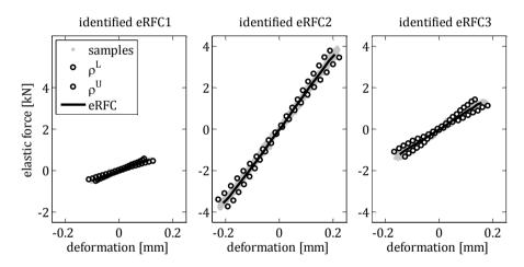
**Figure 5.9:** Identified elastic RFCs of the PFW's 3DoF model.
