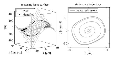
**Figure 3.15:** True and identified cRFS (left) of the Van der Pol oscillator and the state space trajectory (right) of the measured virtual system during a load case without external excitation, i.e. u(t)=0.
