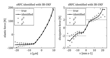
**Figure 3.13:** Comparison of the true and the identified eRFC (left) and dRFC (right) of a 1DoF dynamic system including the corresponding uncertainty curves  $\rho^L$  and  $\rho^U$ . The identification was carried out based on acceleration measurement using the SR-UKF.
