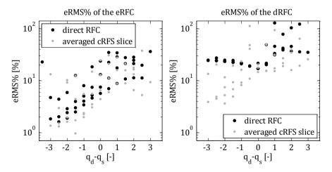
**Figure 3.6:** Results of the parameter study of  $q_s$  and  $q_d$  using the virtual frequency sweep measurement of a 1DoF system with additive nonlinearity. Additive identification ("direct RFC") is compared to coupled identification ("averaged cRFS slice") based on the *eRMS*% error (q.v. Appendix B) of the identified eRFC (left) and dRFC (right).
