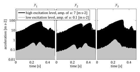
**Figure 4.1:** Noisy measurement signals of the virtual 3DoF system from Section 3.3.2 with logarithmic scaling in case of frequency sweep at two different excitation levels.
