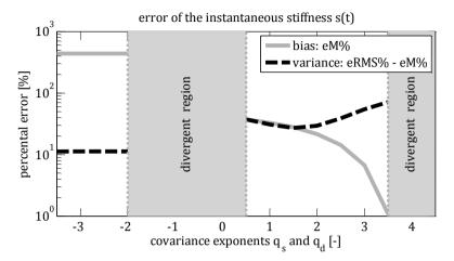
**Figure 2.7:** Bias and variance of s(t) (based on *eM%* and *eRMS%* according to Appendix B) on the example of the virtual 1DoF nonlinear oscillator from Section 3.1.1 using the EKF.  $q_s$  and  $q_d$  have been increased simultaneously.
