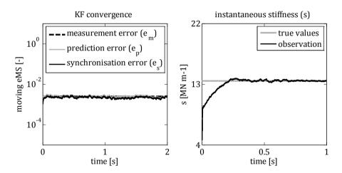
**Figure 2.4:** Classical tuning of the KF for the estimation of constant augmented states on the example of a virtual frequency sweep measurement of a 1DoF oscillator with constant stiffness and damping.  $q_s$  and  $q_d$  have been set to -2.
