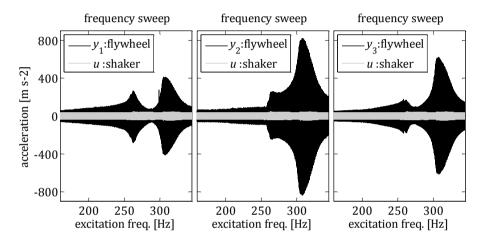
**Figure 5.7:** Measured axial vibration of the DMF's PFW during a forward frequency sweep with axially preloaded SFW. Both u and  $y_i$  were measured via accelerometers. The signals were captured at a sampling rate of 10 kHz. The time axis is replaced by the corresponding frequency of the excitation signal.
