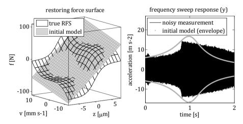
**Figure 3.1:** Comparison of the initial model and the true system based on the corresponding RFSs (left) and frequency sweep response time series (right).
