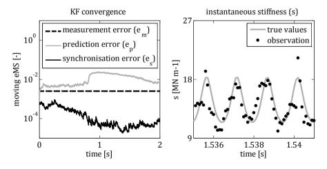
**Figure 2.6:** Optimised tuning of the KF for quickly varying augmented states on the example of the virtual 1DoF nonlinear oscillator from Section 3.1.1.  $q_s$  and  $q_d$  have been set to 3.
