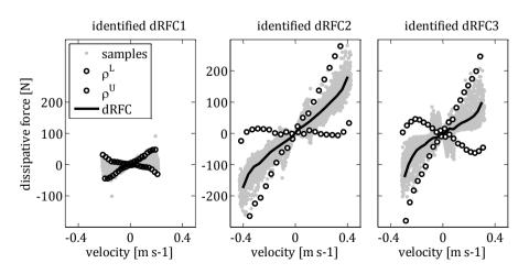
Figure 5.10: Identified dissipative RFCs of the PFW's 3DoF model.
