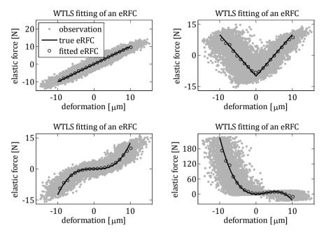
**Figure 2.15:** Different RFC fitting examples carried out using the proposed nonparametric WTLS approach based on synthetic correlated noisy observations.
