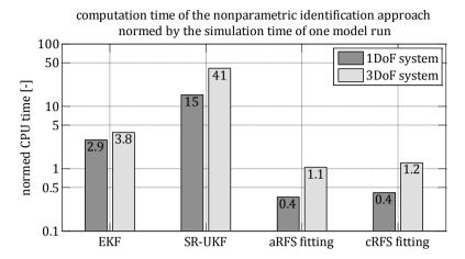
**Figure 3.26:** Computational efficiency of the proposed nonparametric technique's separate steps based on the identification examples from Section 3.1 and 3.3.
