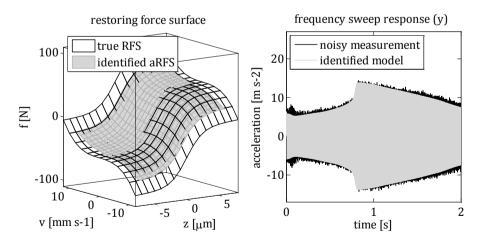
**Figure 3.2:** Comparison of the true and the identified system based on the corresponding RFSs (left) and frequency sweep response time series (right). The identification has been carried out assuming an additive nonlinearity (aRFS).
