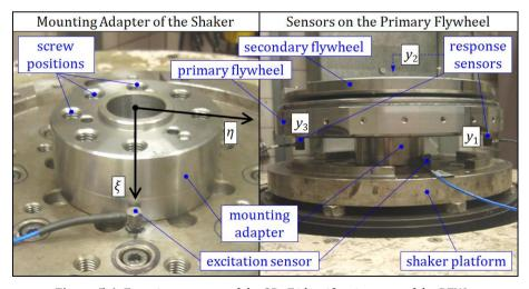
**Figure 5.6:** Experiment setup of the 3DoF identification case of the PFW.
