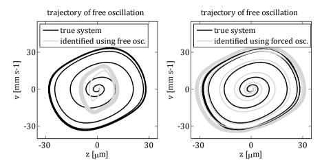
**Figure 3.17:** Comparison of the identified Van der Pol system's free oscillation to the true limit cycle for the two different identification load cases: free oscillation (left) and forced vibration (right).
