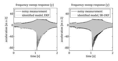
**Figure 3.14:** Comparison of the identified 1DoF system's frequency sweep response time series to the true measured response. The identification was carried out using the two KF types: EKF (left) and SR-UKF (right).
