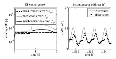
**Figure 2.5:** Classical tuning of the KF in case of quickly varying augmented states on the example of the virtual 1DoF nonlinear oscillator from Section 3.1.1.  $q_s$  and  $q_d$  have been set to 1.
