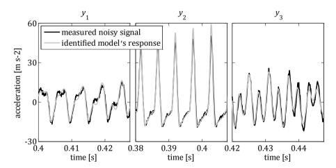
**Figure 4.5:** Noisy (5 % RMS) high amplitude response of the virtual 3DoF system (q.v. Section 3.3.2) compared to the adapted model's response using the identified RFSs and the estimated  $\bf M$  based on the high amplitude measurement with the iterated SR-UKF.
