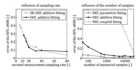
**Figure 3.23:** Investigation of the influence of measurement sampling rate (left) and the number of measured samples (right) on the estimation error of the identified RFS based on the noisy (5 % RMS) virtual measurement of a 1DoF nonlinear oscillator. The resolution of the reconstructed RFS's lookup table was set to 20 segments per dimension.
