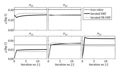
**Figure 4.3:** Convergence of the virtual 3DoF system's inertia properties from Section 3.3.2. The global iteration of the KF has been carried out based on the "nonlinear" load case with high excitation level.
