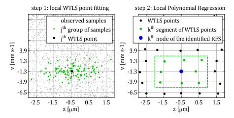
**Figure 2.16:** Illustration of the two steps of the presented nonparametric surface fitting approach in the  $\{z,v\}$  plane. Intermediate samples are generated using local WTLS point fitting (left). The intermediate samples are then used in a subsequential quadratic Local Polynomial Regression (right).
