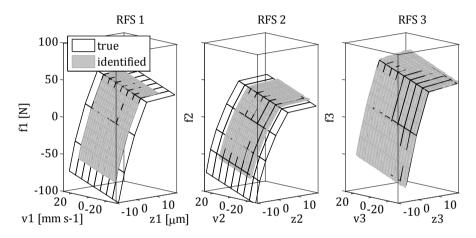
**Figure 3.19:** Comparison of the true and the identified RFSs of the 3DoF mechanical structure. The identification was carried out in its additive form using the EKF.
