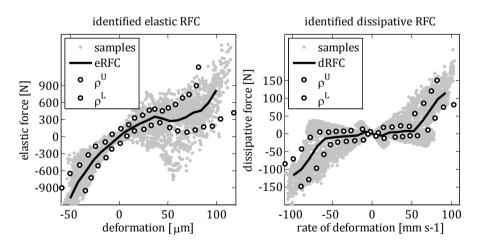
**Figure 5.3:** Identified eRFC (left) and dRFC (right) of the restoring force between the secondary flywheel and the shaker platform.  $\rho^U$  and  $\rho^L$  denote the estimated uncertainty curves according to Section 2.3.2.
