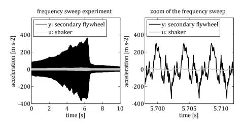
**Figure 5.2:** Measured axial vibration of the SFW during a forward frequency sweep from 200 Hz to 400 Hz without axial preload. Both u and y were measured via accelerometers. The signals were captured at a sampling rate of 20 kHz. Average RMS noise levels of 8 % and 19 % (*eRMS*%, q.v. Appendix B) have been determined for u and y respectively.
