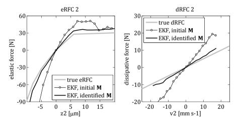
**Figure 4.4:** Identified eRFCs and dRFCs of the virtual 3DoF system's (q.v. Section 3.3.2) second spring element using the initial guess of **M** in comparison to using the identified **M** based on the high amplitude measurement with the iterated SR-UKF.
