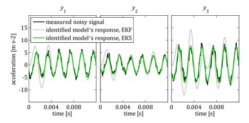
**Figure 4.8:** Initial time interval of the virtual 3DoF system's (q.v. Section 3.3.2) response signals. The true noisy time series (black) are compared to the adapted model's response involving initial states set to zero (grey) in comparison to initial states adapted using the iterated EKS (green).
