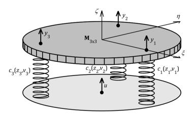
**Figure 3.18:** Virtual experiment setup of a rigid plate on elastic foundation with one translational DoF in  $\zeta$  direction and two tilting DoFs around the  $\xi$  and  $\eta$  coordinate axes. The three bipolar spring elements represent general nonlinear RFSs between the ground and the body.
