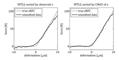
**Figure 2.13:** The true curve of a highly nonlinear eRFC is compared to the WTLS smoothed samples based on synthetic correlated noisy observations. Sorting over the observed deformation (left) is compared to the sorting over the CMA5 moving averaged deformation (right).
