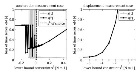
**Figure 3.10:** Bias (eM, q.v. Appendix B) of the time series of z(t) and s(t) with respect to their true values for different lower bound levels of the effective stiffness in case of acceleration (left) and displacement (right) measurement.
