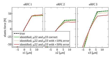
**Figure 3.24:** Influence of the incorrect values of the inverse inertia matrix's diagonal entries on the estimation accuracy of the 3DoF virtual system's three eRFCs from Section 3.3.2.
