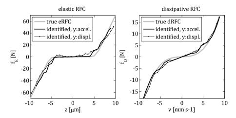
**Figure 3.8:** Comparison of the true and the identified eRFC (left) and dRFC (right) of a 1DoF nonlinear dynamic system involving backlash. The identification results for the two measurement types, displacement and acceleration, are compared.
