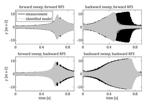
**Figure 3.5:** Measured forward (left) and backward (right) frequency sweep response time series of a 1DoF nonlinear system compared to the responses of two identified models. The first (top) has been identified during the forward sweep, while the second (bottom) is based on the backward sweep. Both sweeps has been carried out in the same frequency range of 200 Hz to 400 Hz.
