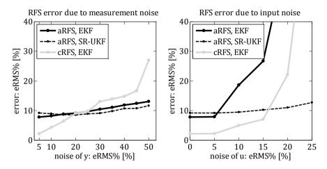
**Figure 3.22:** Comparison of different subtypes of the proposed nonparametric identification algorithm based on the estimation error of the identified RFS of the 1DoF system from Section 3.1.1 as a function of the noise level applied to the measurement signal y (left) and to the input signal u (right).
