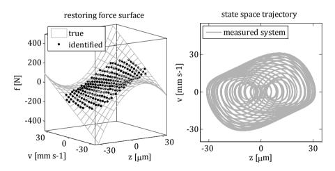
**Figure 3.16:** True and identified cRFS (left) of the Van der Pol oscillator and the state space trajectory (right) of the measured virtual system during a load case with an external excitation of  $u(t)=15\sin(2\pi 100t)$  ms<sup>-2</sup>.
