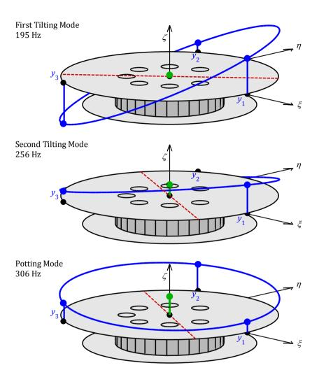
**Figure 5.12:** Eigenmodes of the measured primary flywheel based on the linearisation of its identified RFCs. Mode shapes (blue) are plotted including the modal displacement at the excitation position (green) and the gradient of the mode shape plane (red dashed line). The positions of the mounting screws are indicated by small black circles.
