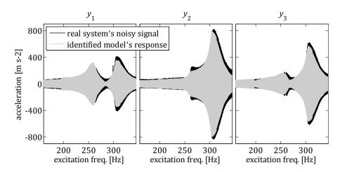
**Figure 5.11:** Comparison of the adapted 3DoF rigid body model's response to the measured continuum vibrations of the PFW during the frequency sweep experiment. The time axis is replaced by the corresponding frequency of the excitation signal.
