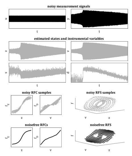
**Figure 2.19:** Workflow of the proposed synchronisation-based nonparametric identification method for nonlinear dynamic systems: Based on the measurement signals the Kalman Filter estimates the states and the instrumental variables (i.e. the instantaneous stiffness and damping). These are transformed into noisy samples of the RFCs and RFSs. Noisefree RFCs and RFSs are generated via optimal curve and surface fitting based on the noisy samples.
