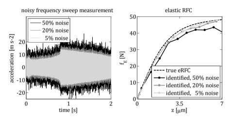
**Figure 3.21:** Comparison of the reconstructed eRFCs (right) of a 1DoF nonlinear system. The additive identification has been carried out based on frequency sweep measurements (left) at different *eRMS%* (q.v. Appendix B) noise levels using the EKF.
