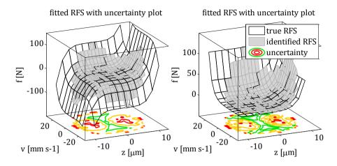
**Figure 2.18:** Comparison of the true and the identified surfaces of two nonlinear RFSs. Fitting was carried out using the presented two-step nonparametric approach based on synthetic correlated noisy samples.
