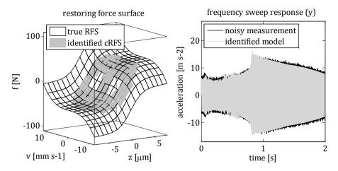
**Figure 3.3:** Comparison of the true and the identified system based on the corresponding RFSs (left) and frequency sweep response time series (right). The identification has been carried out assuming a coupled nonlinearity (cRFS).
