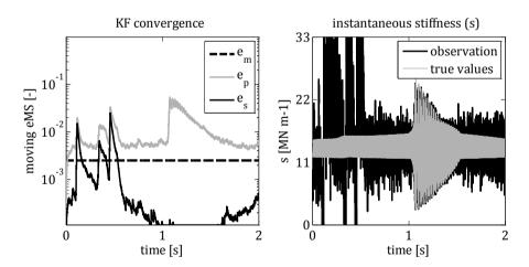
**Figure 2.10:** Convergence plot (left) and the time sequence of the instantaneous stiffness (right) according to the virtual frequency sweep measurement of the strongly nonlinear 1DoF oscillator from Section 3.1.3.
