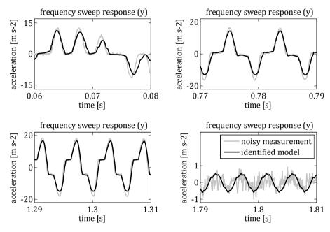
**Figure 3.9:** Comparison of the true and the identified system based on four different time segments of the corresponding frequency sweep response time series. The identification has been carried out using acceleration measurement.
