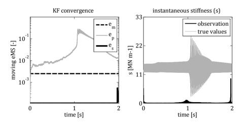
**Figure 2.9:** Convergence plot (left) and the time sequence of the instantaneous stiffness (right) in case of the inconsistence of the KF caused by the deactivation of the lower bound constraint of the stiffness. Virtual frequency sweep measurement of the strongly nonlinear 1DoF oscillator from Section 3.1.3.
