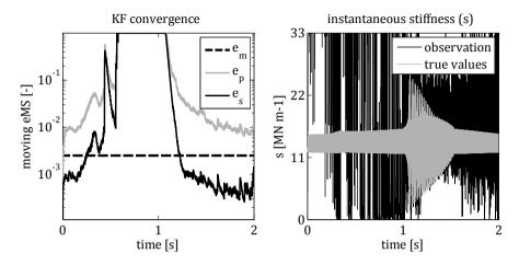
**Figure 2.8:** Convergence plot (left) and the time sequence of the instantaneous stiffness (right) in case of KF divergence due to improper tuning. Virtual frequency sweep measurement of the strongly nonlinear 1DoF oscillator from Section 3.1.3.
