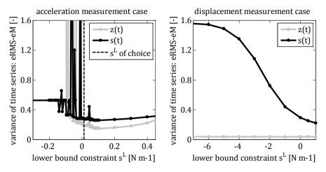
**Figure 3.11:** Variance (eRMS-eM, q.v. Appendix B) of the time series of z(t) and s(t) with respect to their true values for different lower bound levels of the effective stiffness in case of acceleration (left) and displacement (right) measurement.
