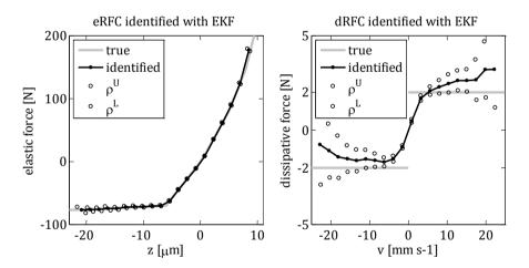
**Figure 3.12:** Comparison of the true and the identified eRFC (left) and dRFC (right) of a 1DoF dynamic system including the corresponding uncertainty curves  $\rho^L$  and  $\rho^U$ . The identification was carried out based on acceleration measurement using the EKF.
