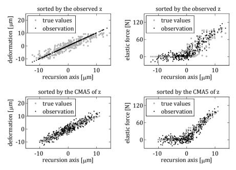
**Figure 2.12:** Sorted samples of a highly nonlinear eRFC based on synthetic correlated noisy observations. Sorting over the observed deformation (top) is compared to the sorting over the CMA5 moving averaged deformation (bottom).
