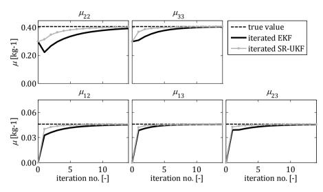
**Figure 4.2:** Convergence of the virtual 3DoF system's inertia properties from Section 3.3.2. The global iteration of the KF has been carried out based on the "linear" load case with low excitation level.
