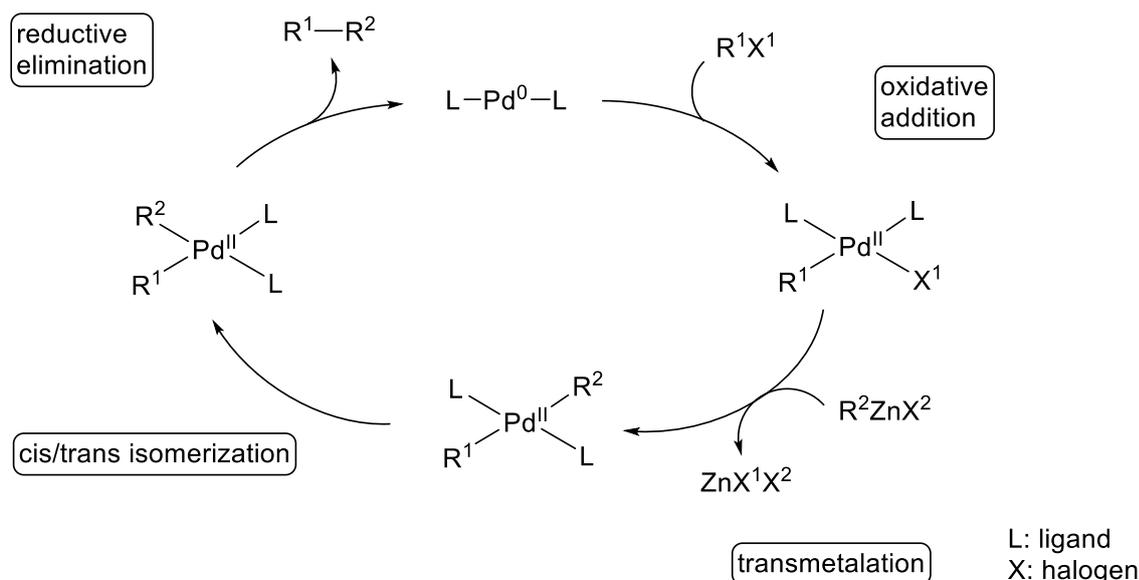
**Scheme 6:** Catalytic cycle of the Negishi reaction. The process of oxidative addition, transmetalation, cis/trans isomerization and reductive elimination is similar in other palladium catalyzed cross-coupling reactions.<sup>[118]</sup>
