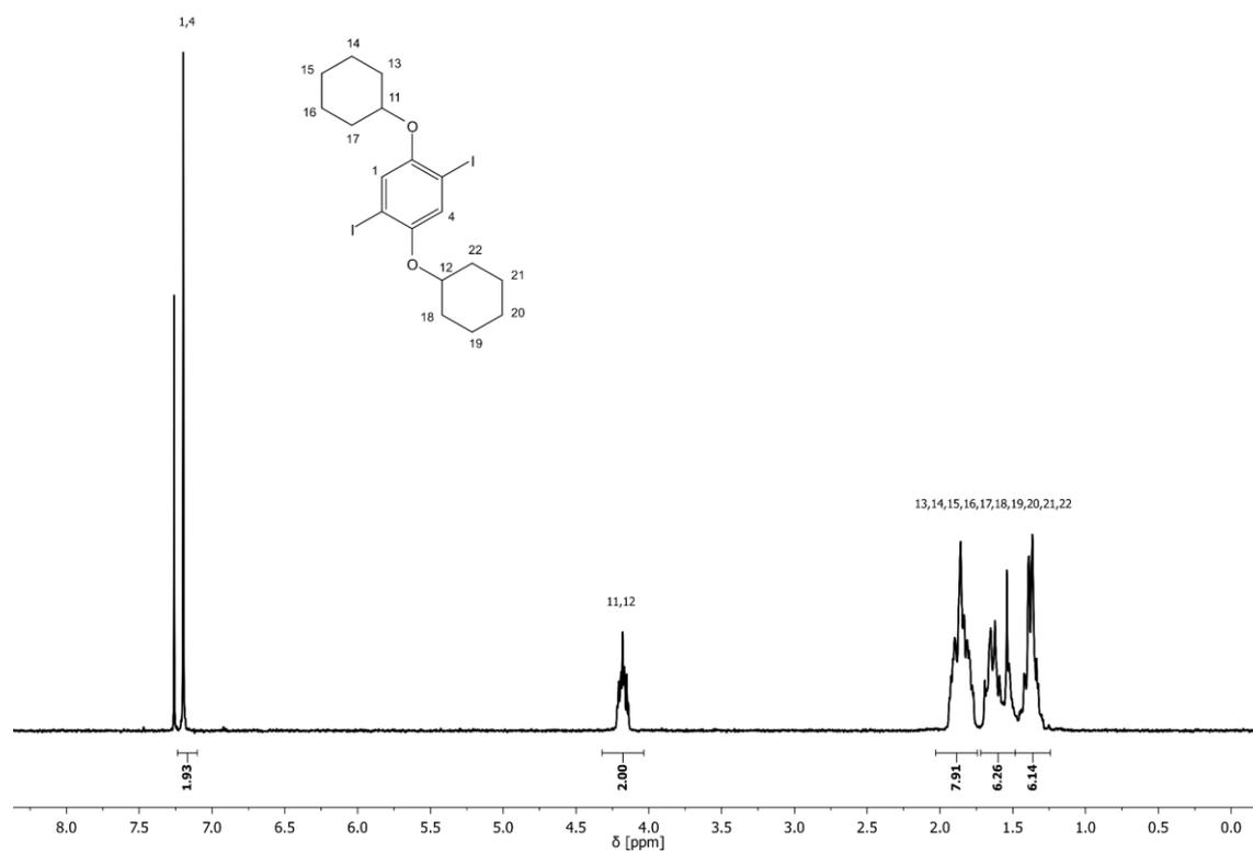
**Figure 49:** <sup>1</sup>H NMR spectrum of precursor **P3b** with assigned signals.
