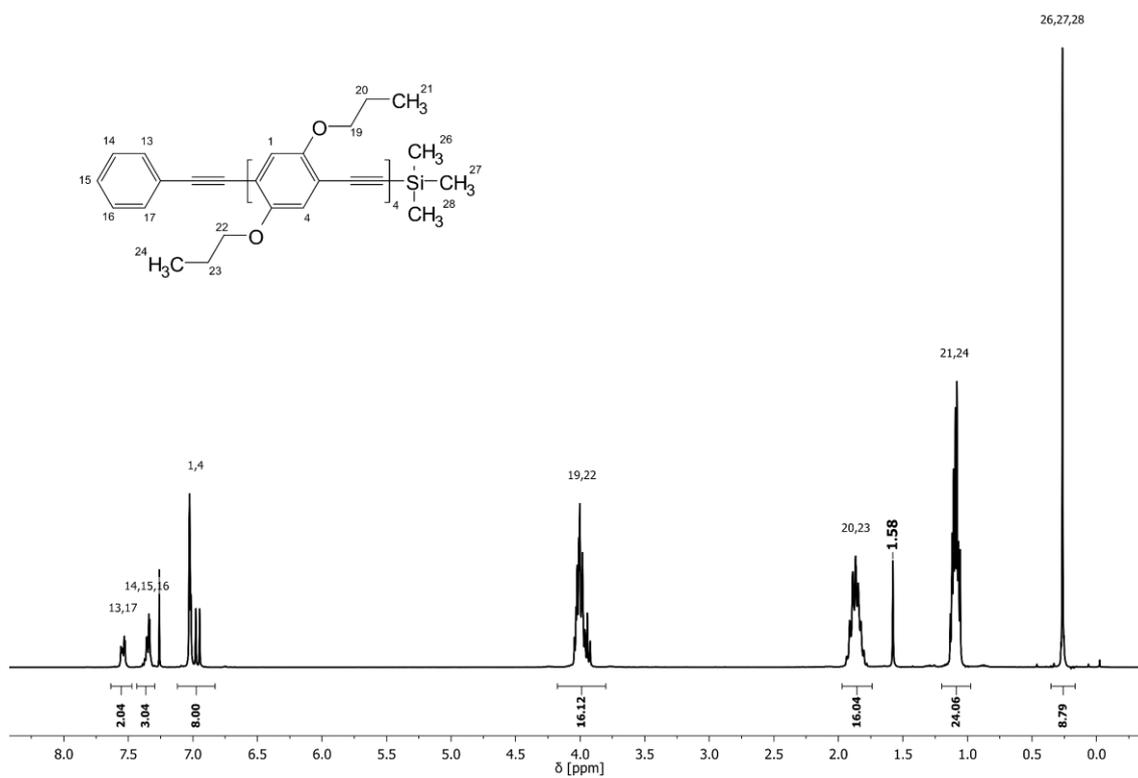
**Figure 68:** <sup>1</sup>H NMR spectrum of protected tetramer **4a** with assigned signals.
