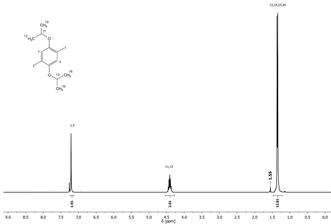
**Figure 46:** <sup>1</sup>H NMR spectrum of precursor **P2b** with assigned signals.
