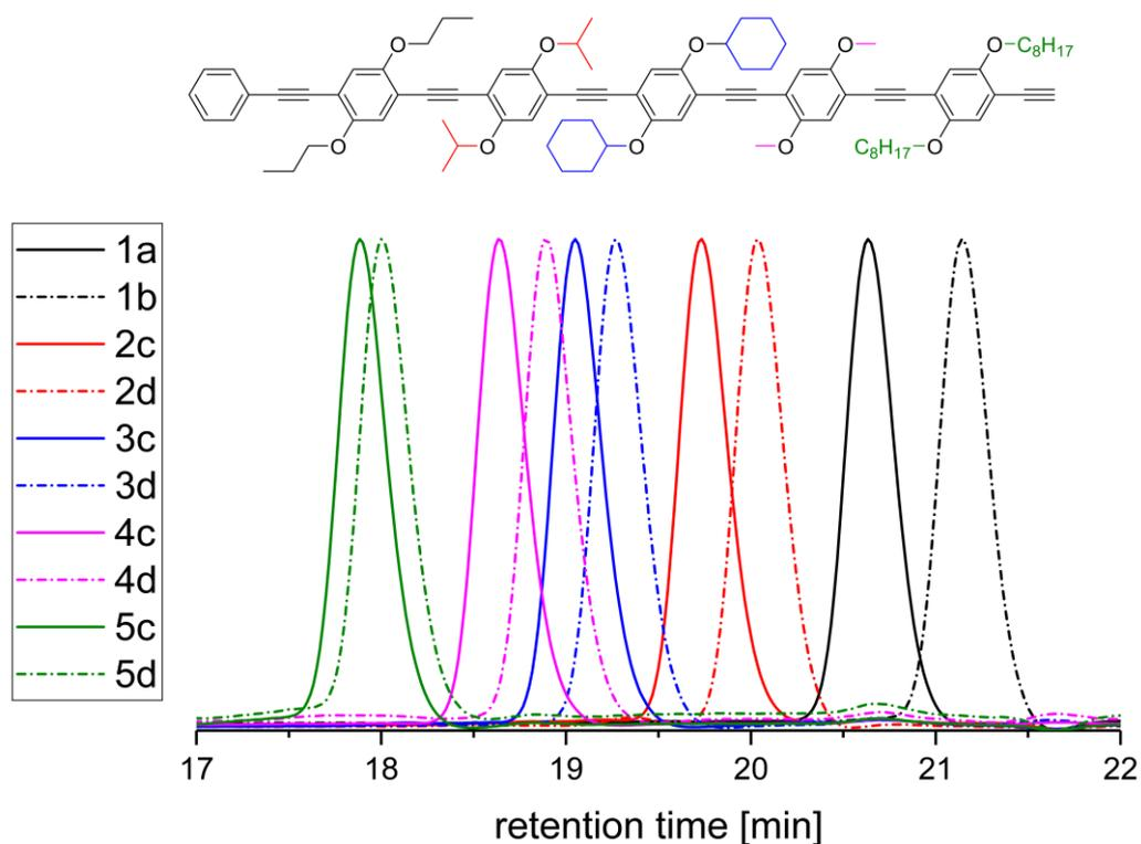
**Figure 34:** SEC traces of the sequence-defined oligomers. The bold line represents the protected, the dotted line the deprotected representatives.
