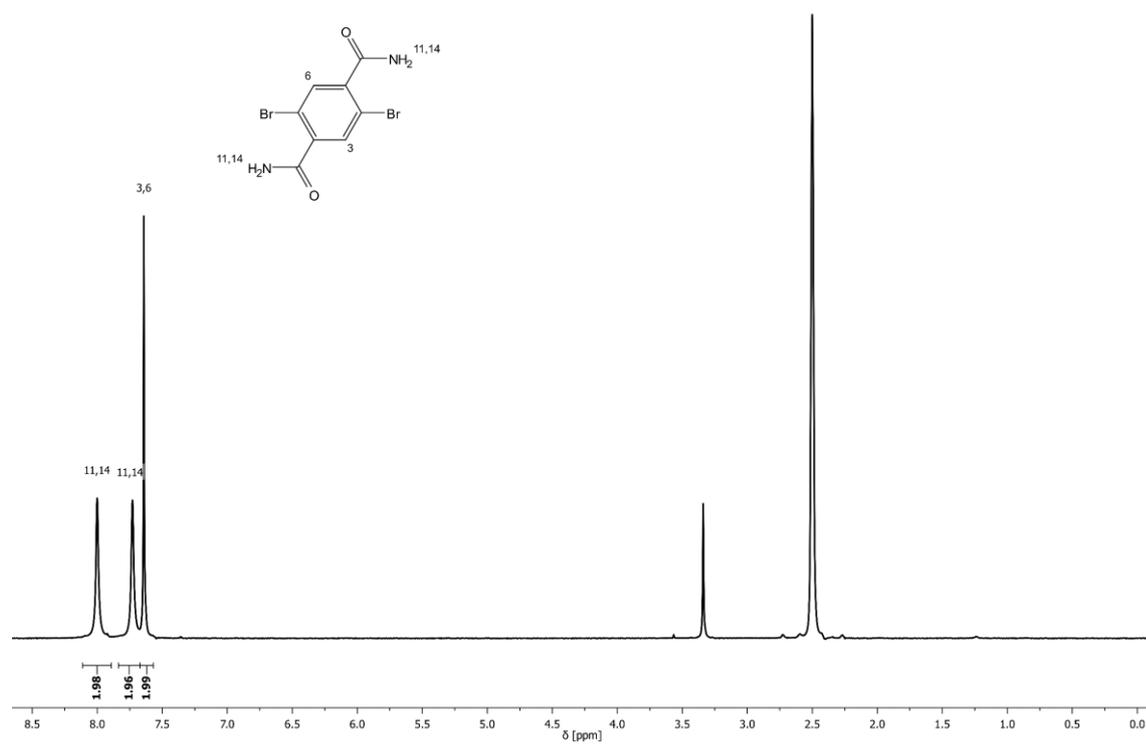
**Figure 59:** <sup>1</sup>H NMR spectrum of precursor **P8a** with assigned signals.
