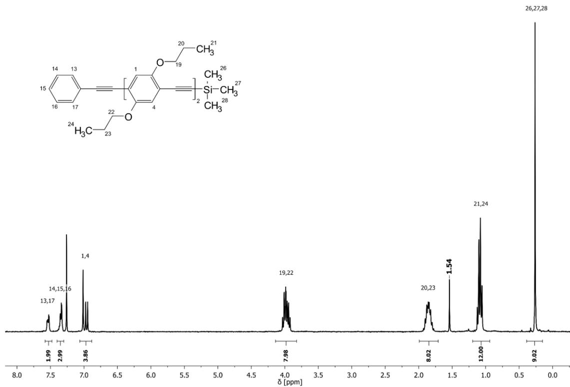
**Figure 64:** <sup>1</sup>H NMR spectrum of protected dimer **2a** with assigned signals.
