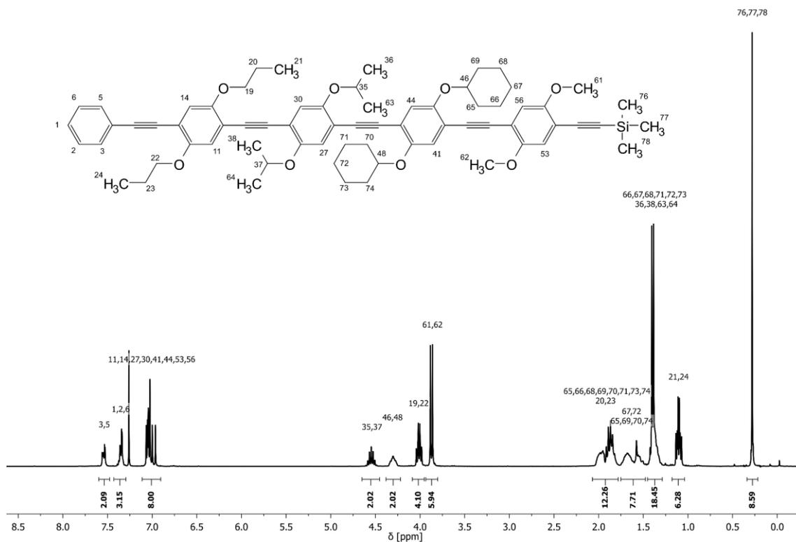
**Figure 77:**  $^1H$  NMR spectrum of protected sequence-defined tetramer **4c** with assigned signals.
