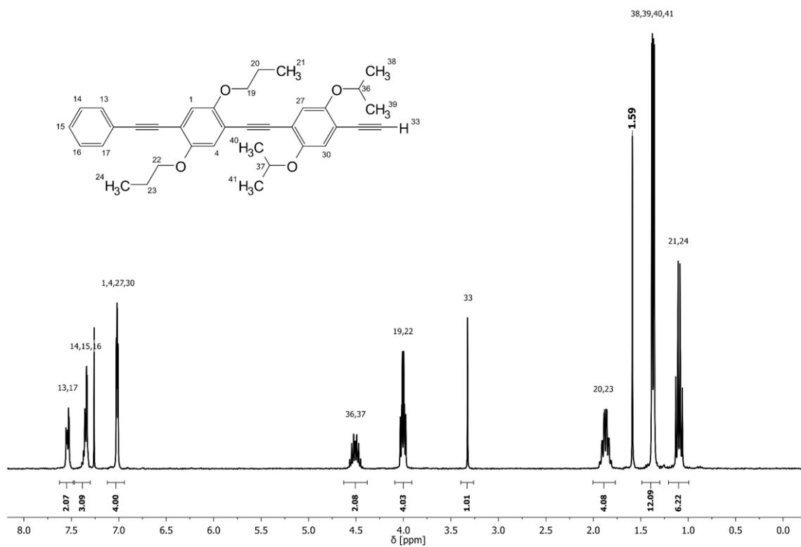
**Figure 74:** <sup>1</sup>H NMR spectrum of deprotected sequence-defined dimer **2d** with assigned signals.
