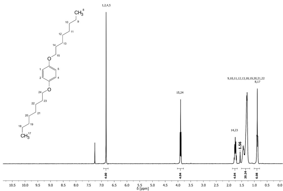
**Figure 53:** <sup>1</sup>H NMR spectrum of precursor **P5a** with assigned signals.
