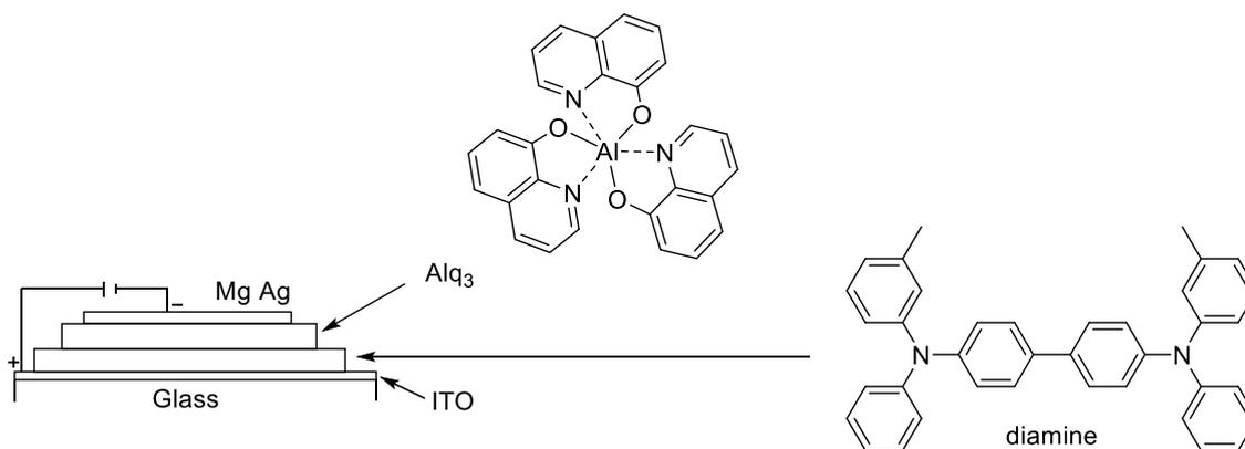
**Figure 8:** The first OLED, a double layer device.<sup>[187]</sup>
