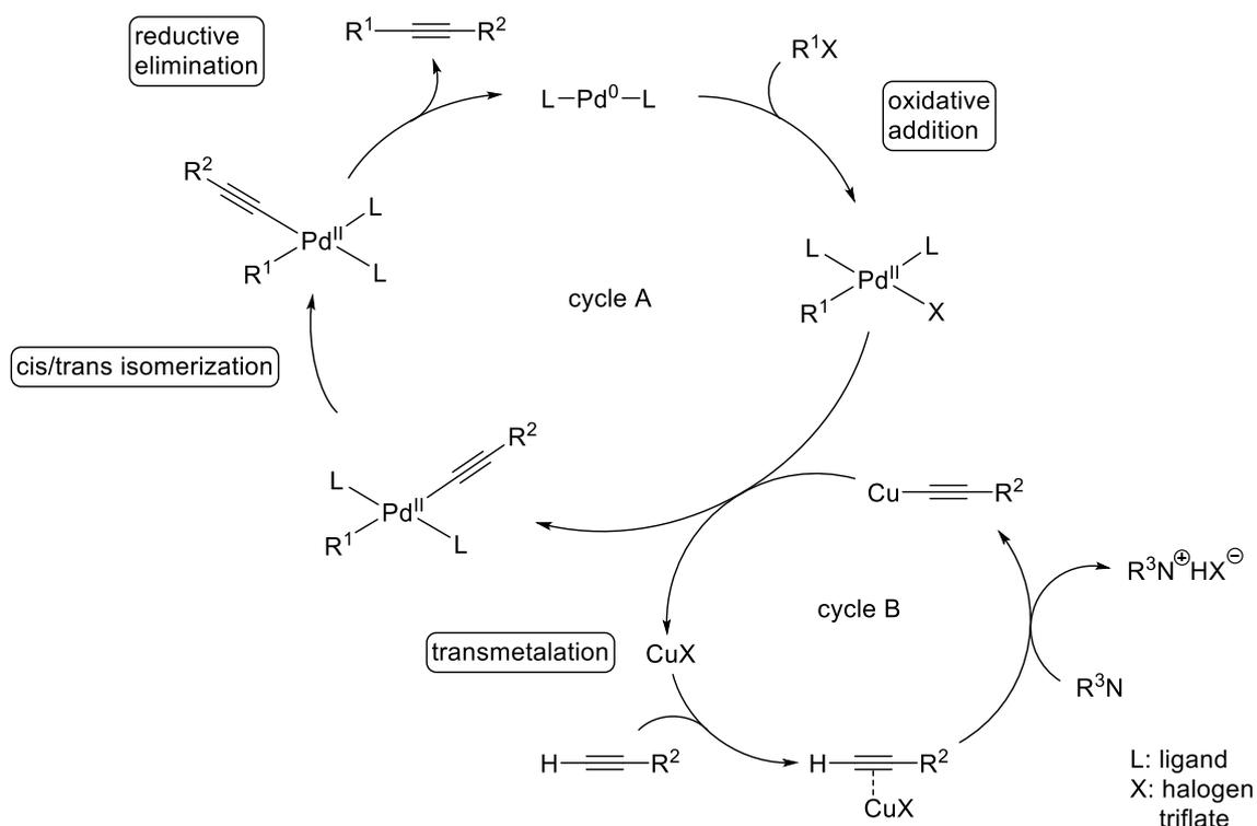
**Scheme 8:** Mechanism of the Sonogashira reaction involving two catalytic cycles.<sup>[127]</sup>
