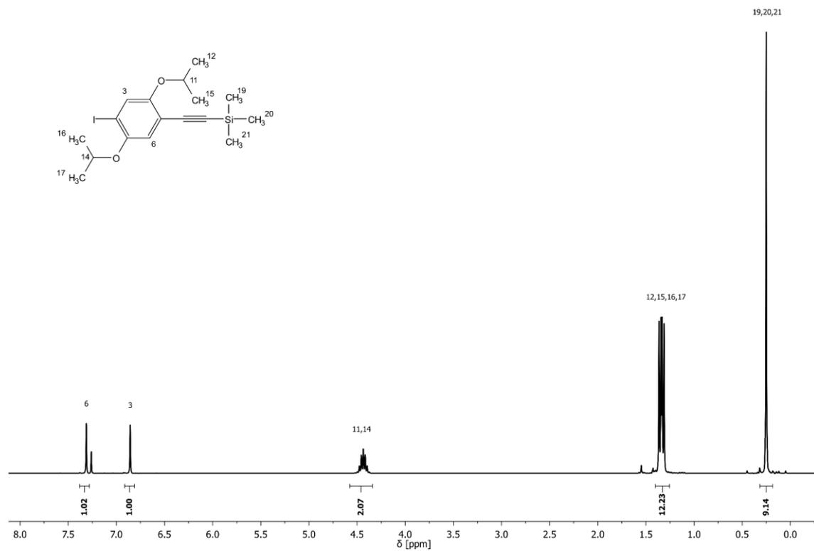
**Figure 47:** <sup>1</sup>H NMR spectrum of building block **B2** with assigned signals.
