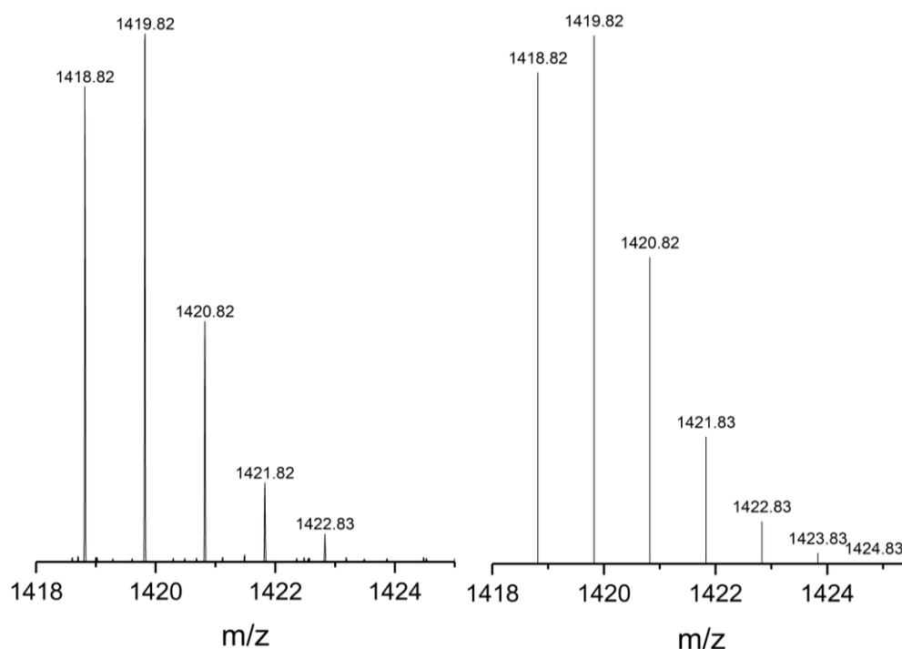
**Figure 32:** Isotope pattern of **5c** detected by ESI-MS (left) and calculated.
