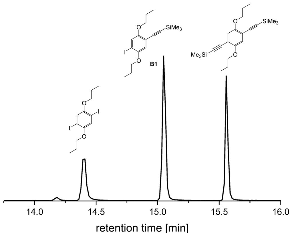
**Figure 12:** Chromatogram of the crude reaction mixture of **B1** obtained by GC. First, the starting material elutes (**P1b**), then the product **B1** followed by the difunctionalized side product.
