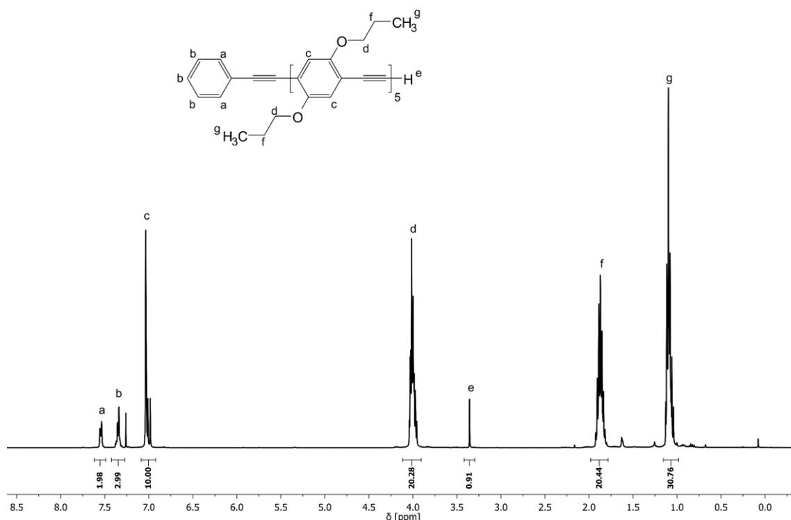
**Figure 21:**  $^1\text{H}$  NMR of pentamer **5b** with assigned signals.
