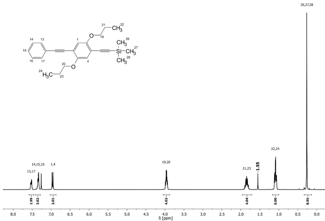
**Figure 61:** <sup>1</sup>H NMR spectrum of protected monomer **1a** with assigned signals.
