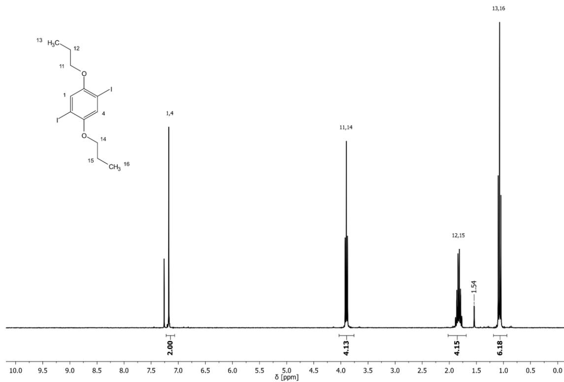
**Figure 43:** <sup>1</sup>H NMR spectrum of precursor **P1b** with assigned signals.
