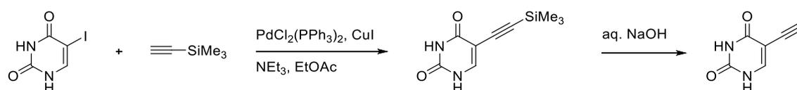
**Scheme 11:** Synthesis of eniluracil *via* Sonogashira coupling with TMSA and subsequent deprotection.<sup>[147]</sup>
