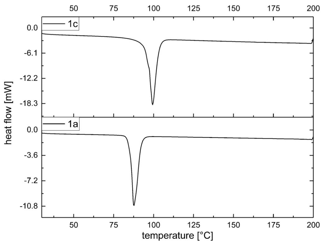
**Figure 25:** DSC trace of benzothiadiazole monomer **1c** in comparison to **1a**. The T<sub>m</sub> of **1a** is with 84.8 °C significantly lower than for **1c** with 95.4 °C. Further thermal events were not detected.
