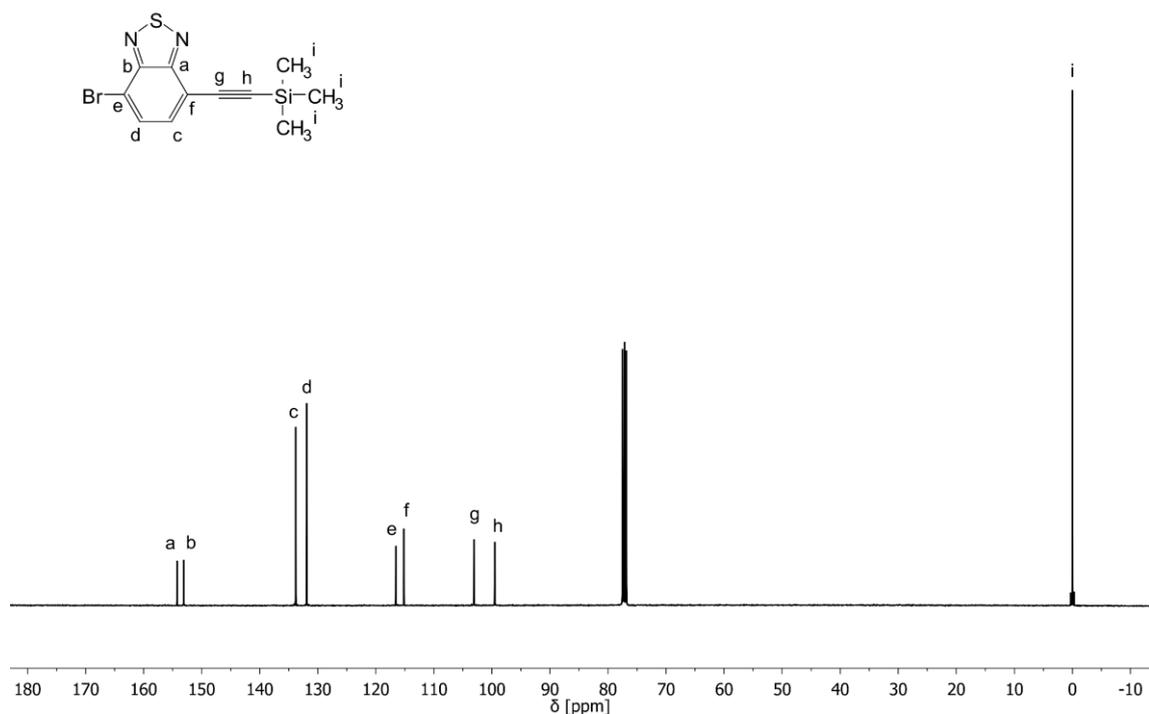
**Figure 16:**  $^{13}\text{C}$  NMR spectrum of building block **B6** with assigned signals.
