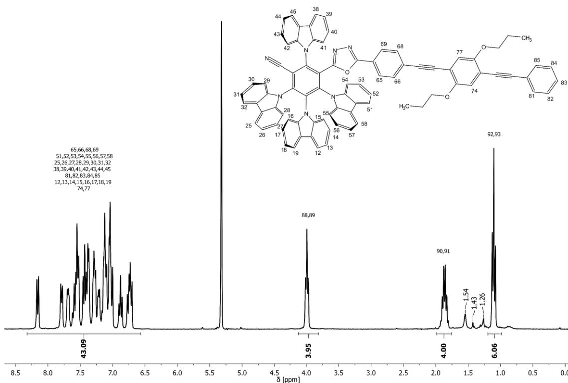
**Figure 81:** <sup>1</sup>H NMR spectrum of monomer-TADF adduct T1 with assigned signals.
