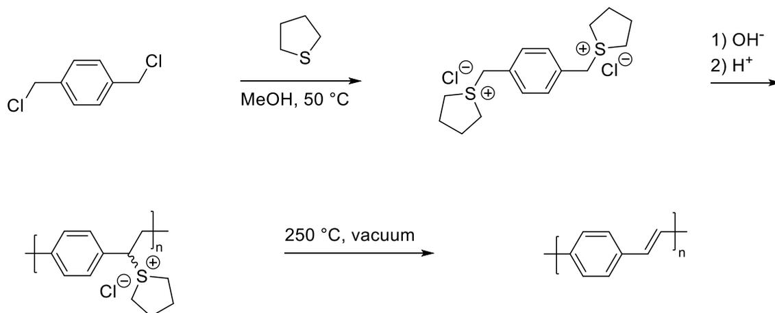
**Scheme 22:** Synthetic route to PPV via a solution-processable precursor. PPV serves as emissive layer in an OLED based on polymers.<sup>[190]</sup>
