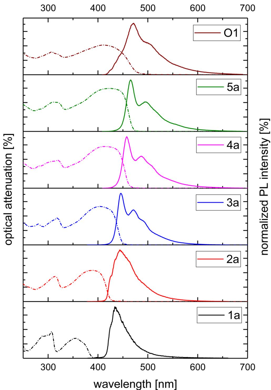
**Figure 28:** Absorption spectrum (dotted) and PL spectrum (bold) of **01** (brown) in comparison to the other protected monodisperse rod-like oligomers **5a-1a**.
