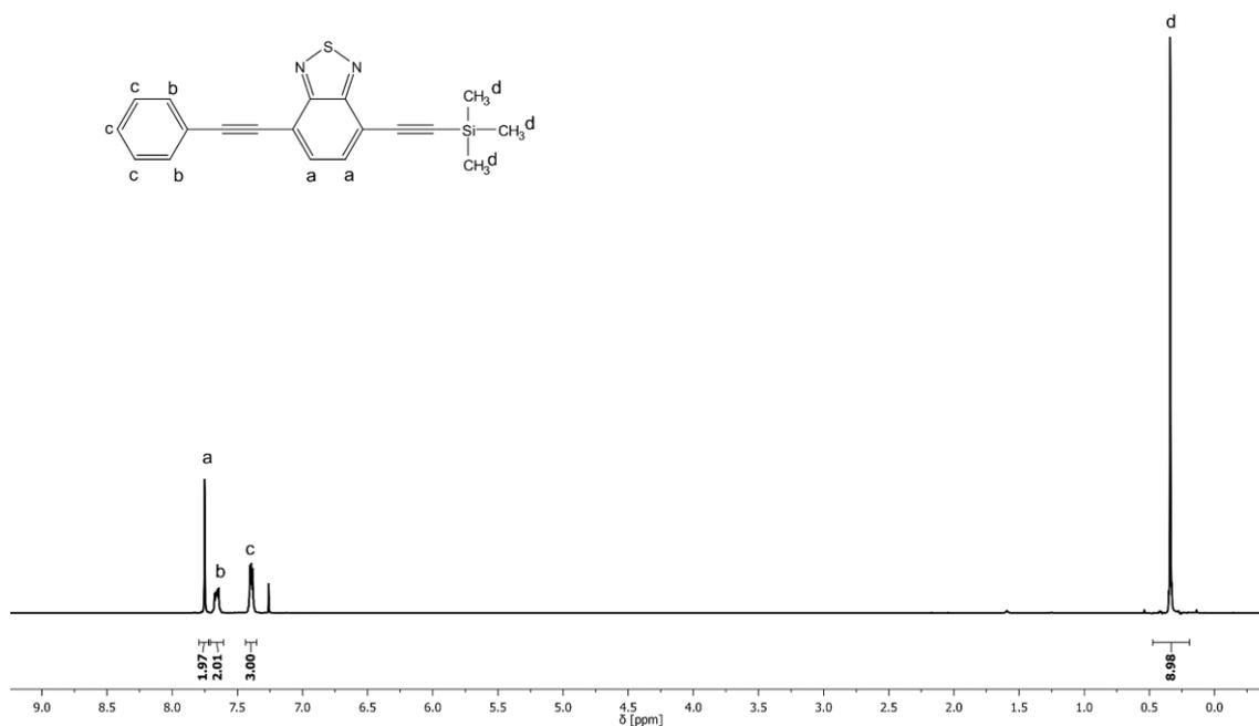
**Figure 24:** <sup>1</sup>H NMR of benzothiadiazole monomer **1c** with assigned signals.
