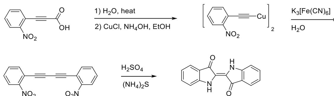
**Scheme 15:** Synthesis of indigo containing a Glaser coupling as first step.<sup>[158]</sup>
