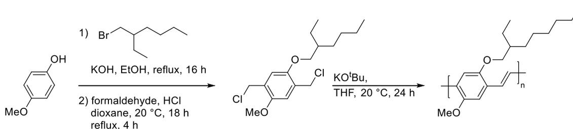
**Scheme 23:** Synthetic route to MEH-PPV. Since MEH-PPV is soluble in organic solvents no precursor was necessary.<sup>[193]</sup>
