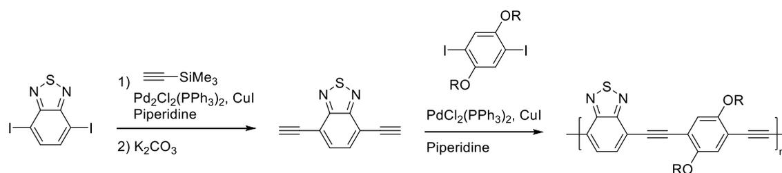
**Scheme 13:** Polymerization *via* Sonogashira cross-coupling to a donor-acceptor copolymer.<sup>[156]</sup>
