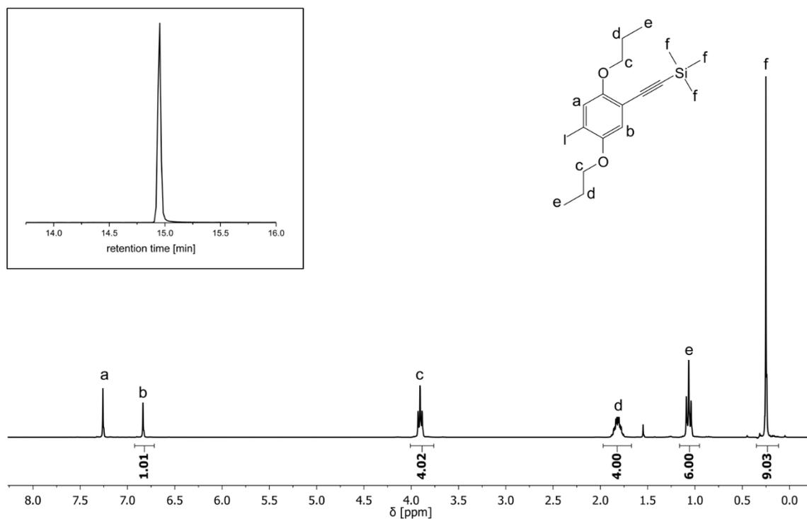
**Figure 13:**  $^1\text{H}$  NMR spectrum of building block **B1** with assigned signals. Signal **a** overlaps with the chloroform in  $\text{CDCl}_3$  (7.26 ppm) and the signal was not integrated. The signal at 1.55 ppm is water present in the  $\text{CDCl}_3$ . Additionally, the chromatogram is depicted, confirming the purity.
