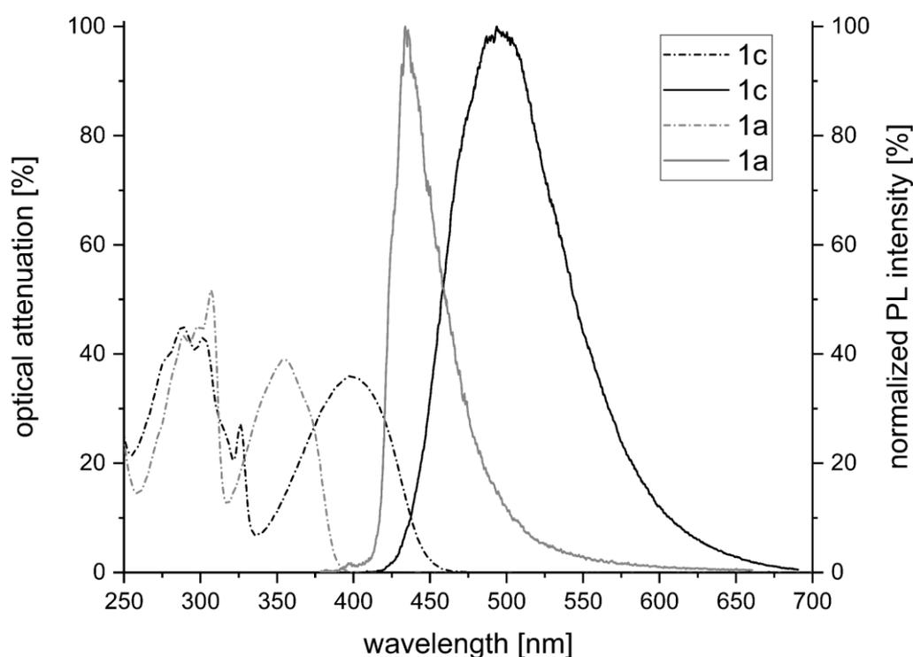
**Figure 26:** Absorption spectrum (dotted) and PL spectrum (bold) of **1c** in comparison to **1a** (grey).
