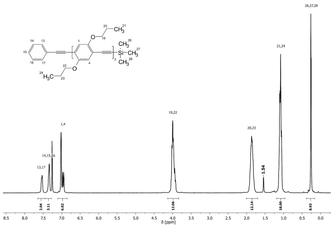
**Figure 66:** <sup>1</sup>H NMR spectrum of protected trimer **3a** with assigned signals.
