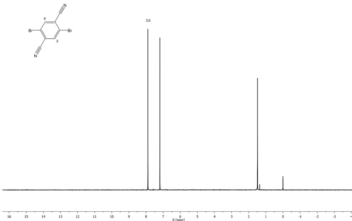
**Figure 60:**  $^1\text{H NMR}$  spectrum of precursor **P8b** with assigned signals.
