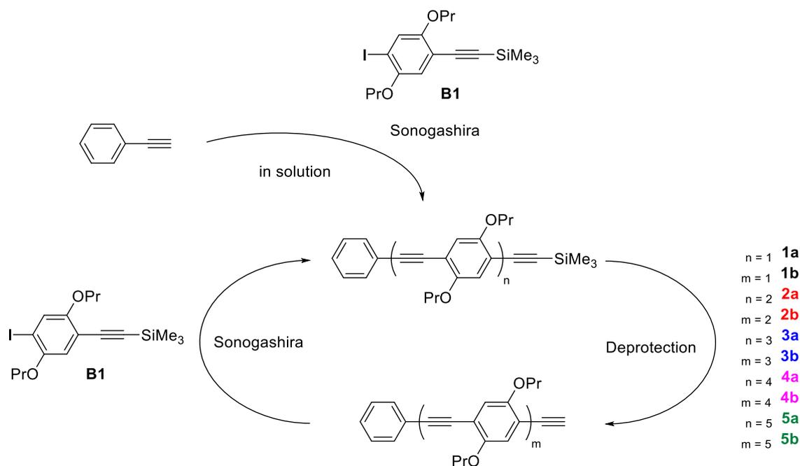
**Scheme 27:** Synthesis procedure to monodisperse rod-like oligomers by iterative Sonogashira cross-coupling and subsequent deprotection.
