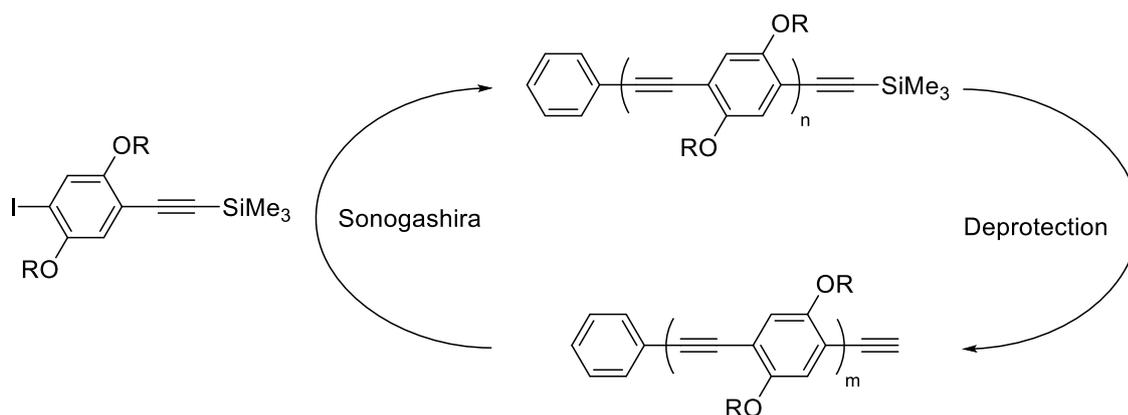
**Scheme 24:** Procedure to sequence-defined rod-like oligomers through Sonogashira reaction and subsequent deprotection.
