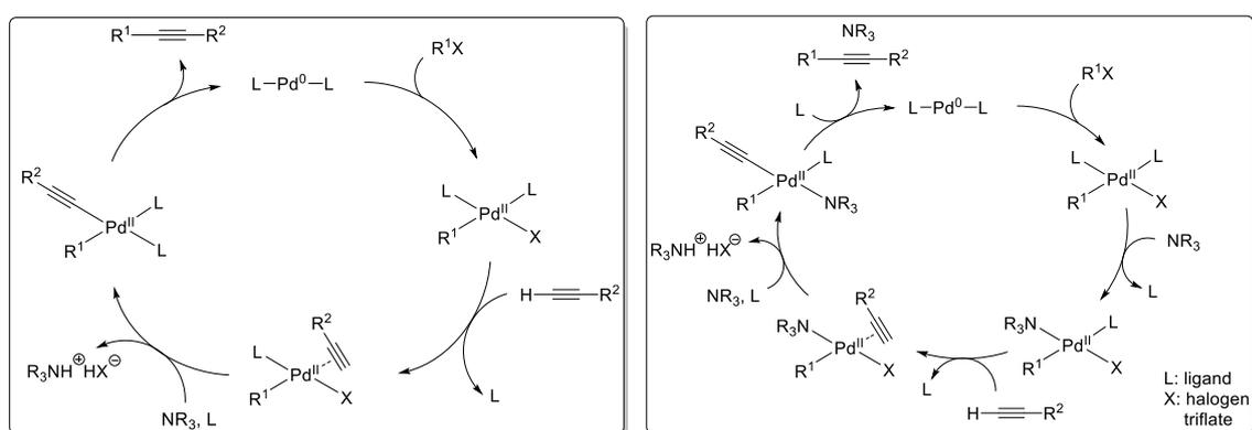
**Scheme 9:** Two possible catalytic cycles for the copper-free Sonogashira reaction.<sup>[127,139]</sup>
