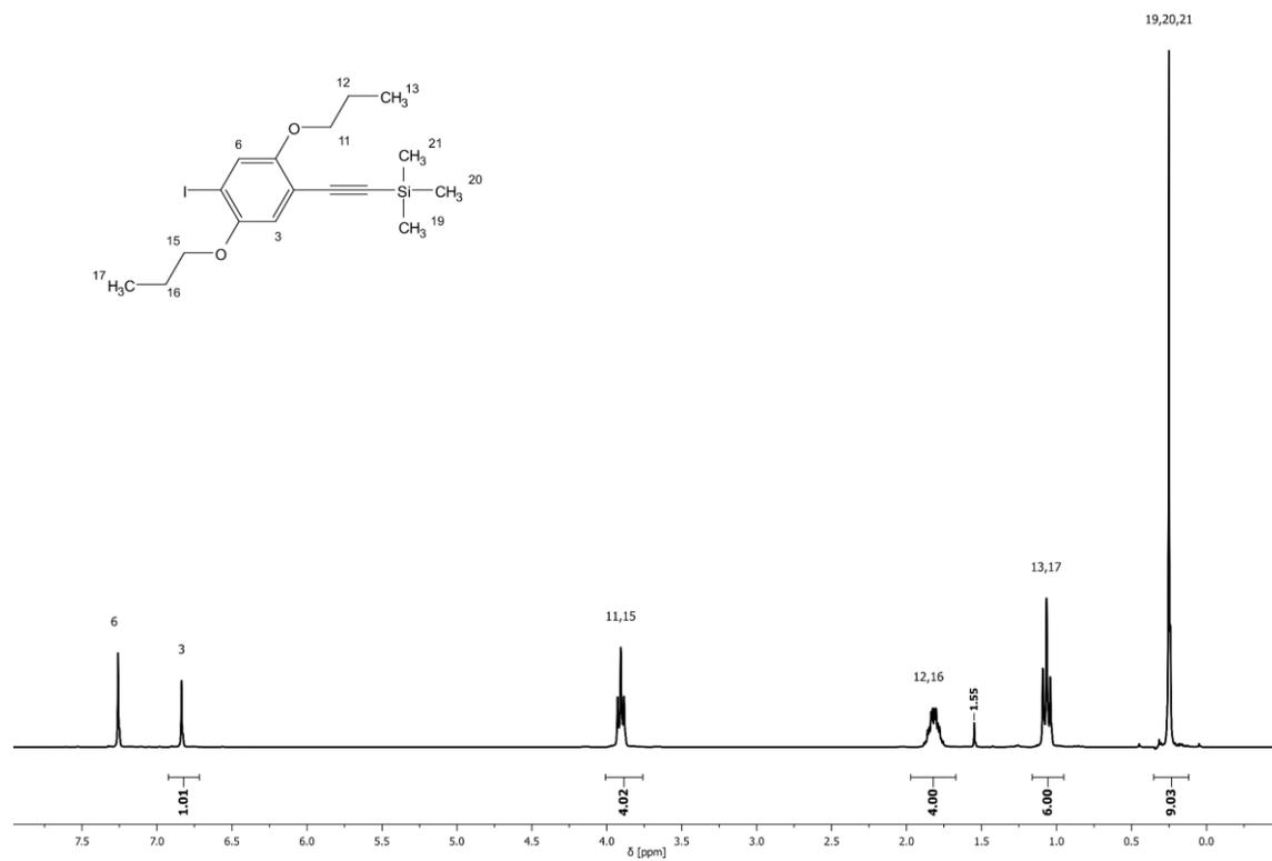
**Figure 44:** <sup>1</sup>H NMR spectrum of building block **B1** with assigned signals.
