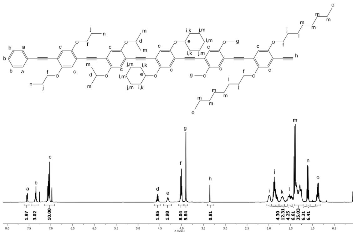
**Figure 33:**  $^1\text{H}$  NMR of deprotected, sequence-defined pentamer **5d** with assigned signals.
