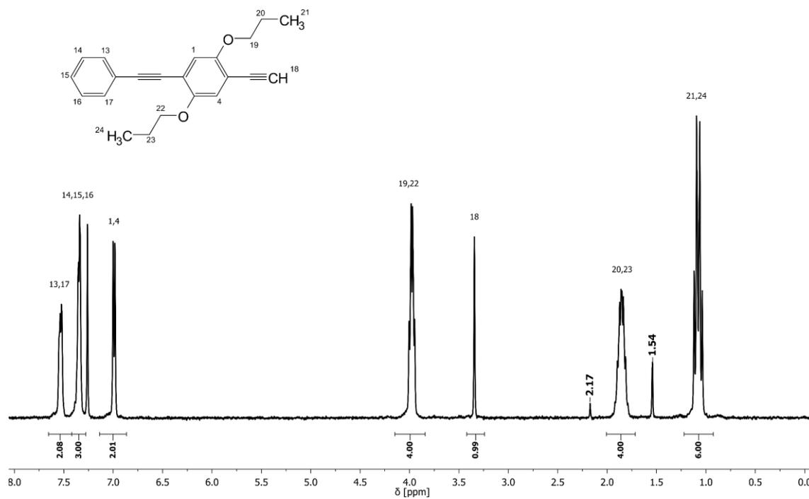
**Figure 62:** <sup>1</sup>H NMR spectrum of deprotected monomer **1b** with assigned signals.
