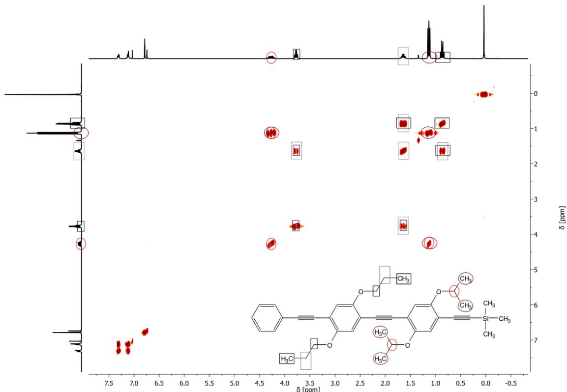
**Figure 29:** COSY spectrum of protected sequence-defined dimer **2c** with assigned signals for the side chains (black and grey rectangles for the propoxy and reddish ellipsoids for the isopropoxy signals).
