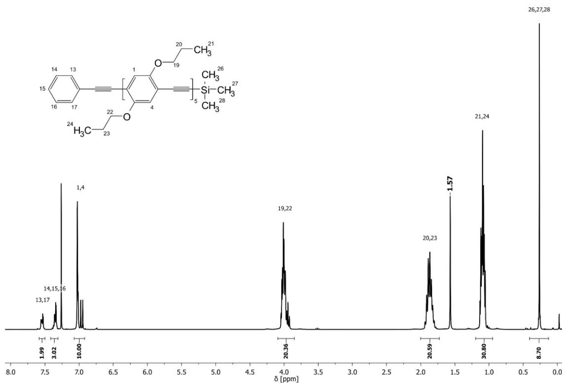
**Figure 70:**  $^1\text{H}$  NMR spectrum of protected pentamer **5a** with assigned signals.
