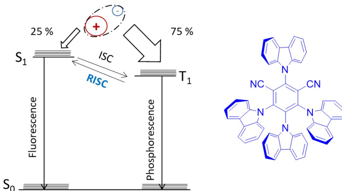
**Figure 9:** Jablonski diagram (left) illustrating the ground state ( $S_0$ ),  $S_1$  and  $T_1$  excited state and the respective ISC and RISC.<sup>[201]</sup> A carbazolyl dicyanobenzene in blue is enabling RISC and TADF is depicted on the right.<sup>[199]</sup>
