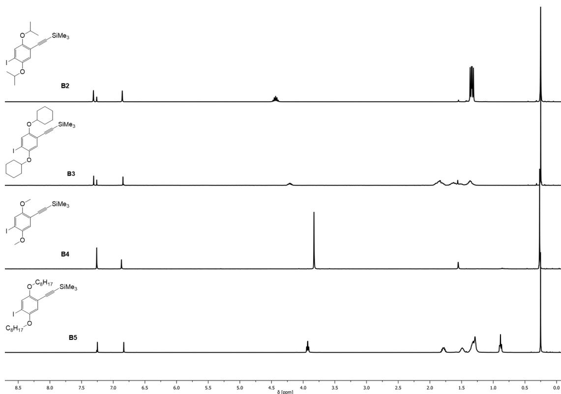
**Figure 15:**  $^1\text{H}$  NMR spectra of the building blocks **B2-B5**. The aromatic signals differ slightly, the respective alkyl signals can be distinguished according to the different moieties.
