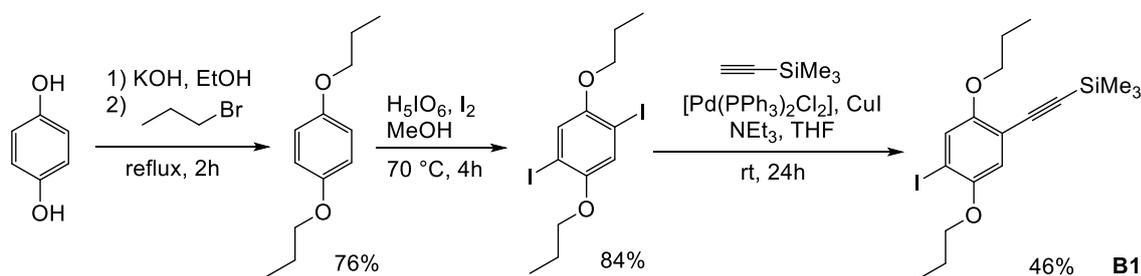
**Scheme 25:** Synthesis of the first building block **B1** based on hydroquinone. First, a Williamson ether synthesis with 1-bromopropane was performed to precursor **P1a**. In the iodination, periodic acid was used as oxidizing agent to form **P1b** and finally, a Sonogashira monocoupling with TMSA was performed. The overall yield of **B1** amounted to 29%.
