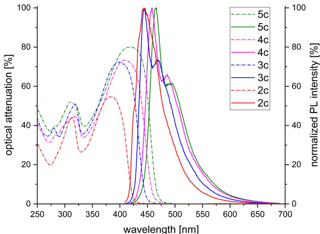
**Figure 35:** Absorption (dotted) and PL (bold) spectra of sequence-defined, protected oligomers **2c-5c**.
