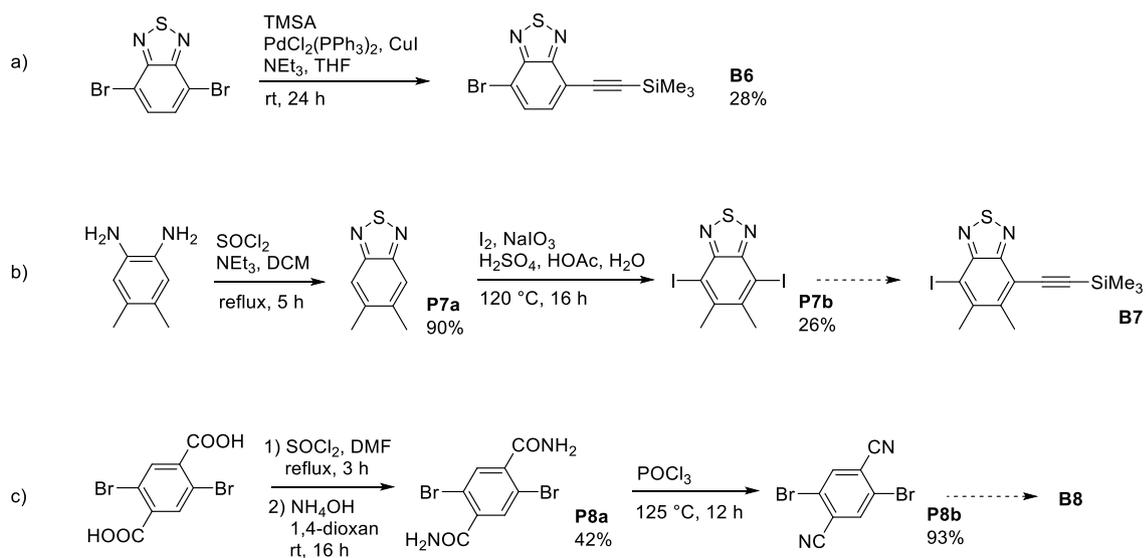
**Scheme 26:** Overview of the syntheses of building blocks with electron accepting properties. a) synthesis of building block **B6** based on a benzothiadiazole, b) synthesis of building block **B7** to a benzothiadiazole with methyl side chains for better solubility, c) synthesis of building block **B8** with cyano moieties.
