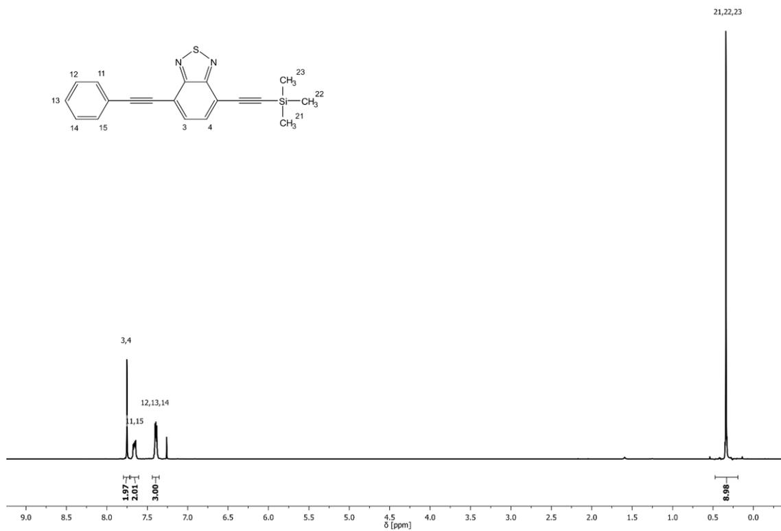
**Figure 63:** <sup>1</sup>H NMR spectrum of protected monomer **1c** with assigned signals.
