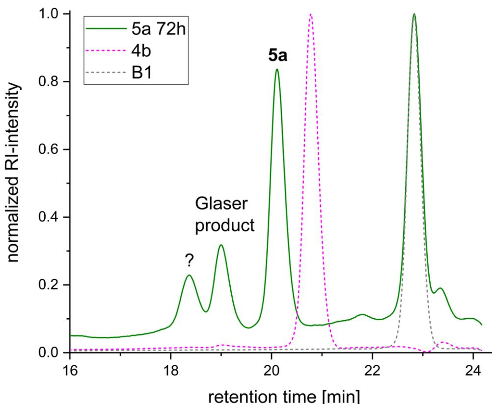
**Figure 20:** SEC trace of crude reaction mixture **5a** (green) in order to check conversion from **4b** (pink). The building block **B1** is depicted in grey. Apart from the Glaser side product, a signal with lower retention time emerges.
