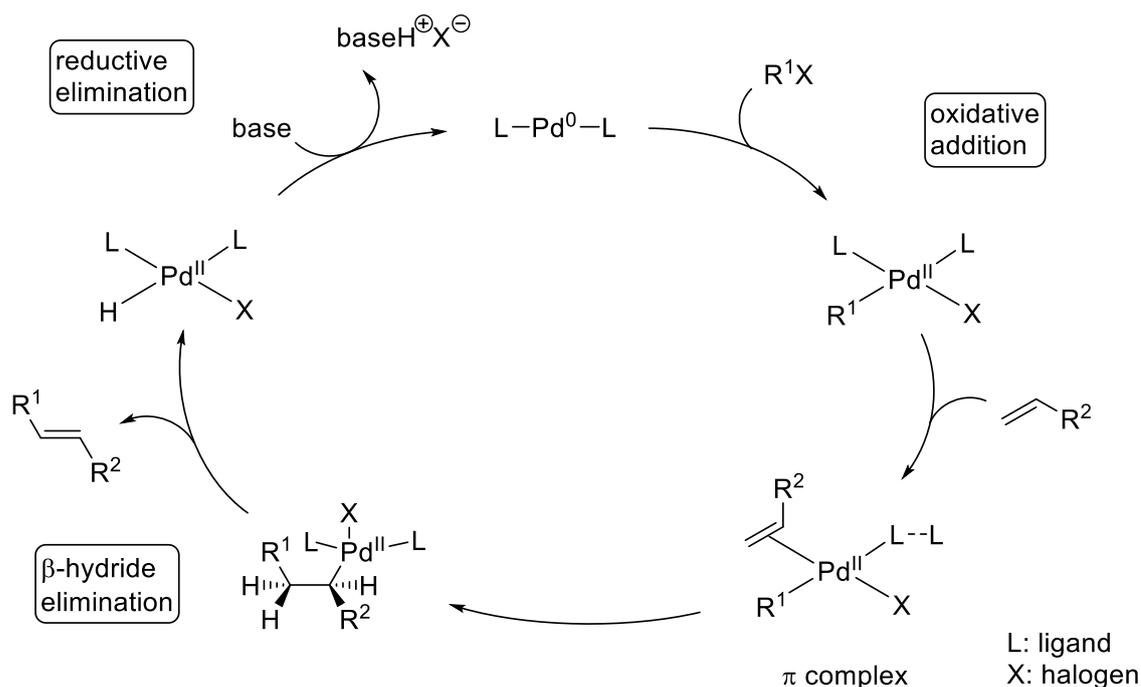
**Scheme 5:** Catalytic cycle of the Heck reaction *via* oxidative addition, migratory insertion,  $\beta$ -hydride elimination and the recovery of the catalyst.<sup>[114]</sup>
