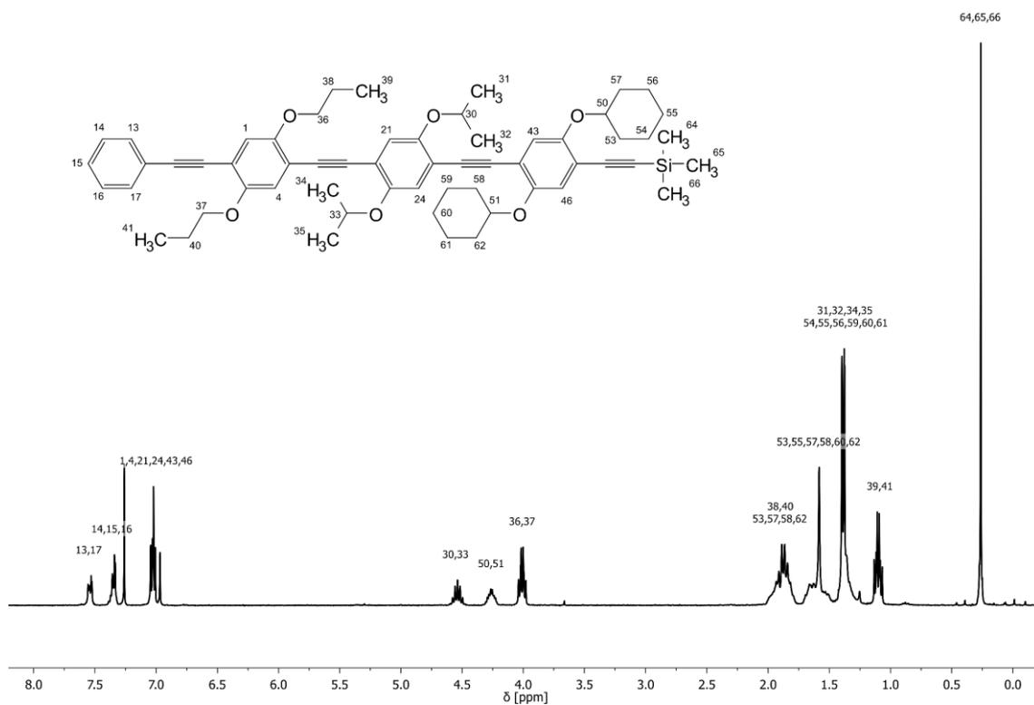
**Figure 75:**  $^1H$  NMR spectrum of protected sequence-defined trimer **3c** with assigned signals.
