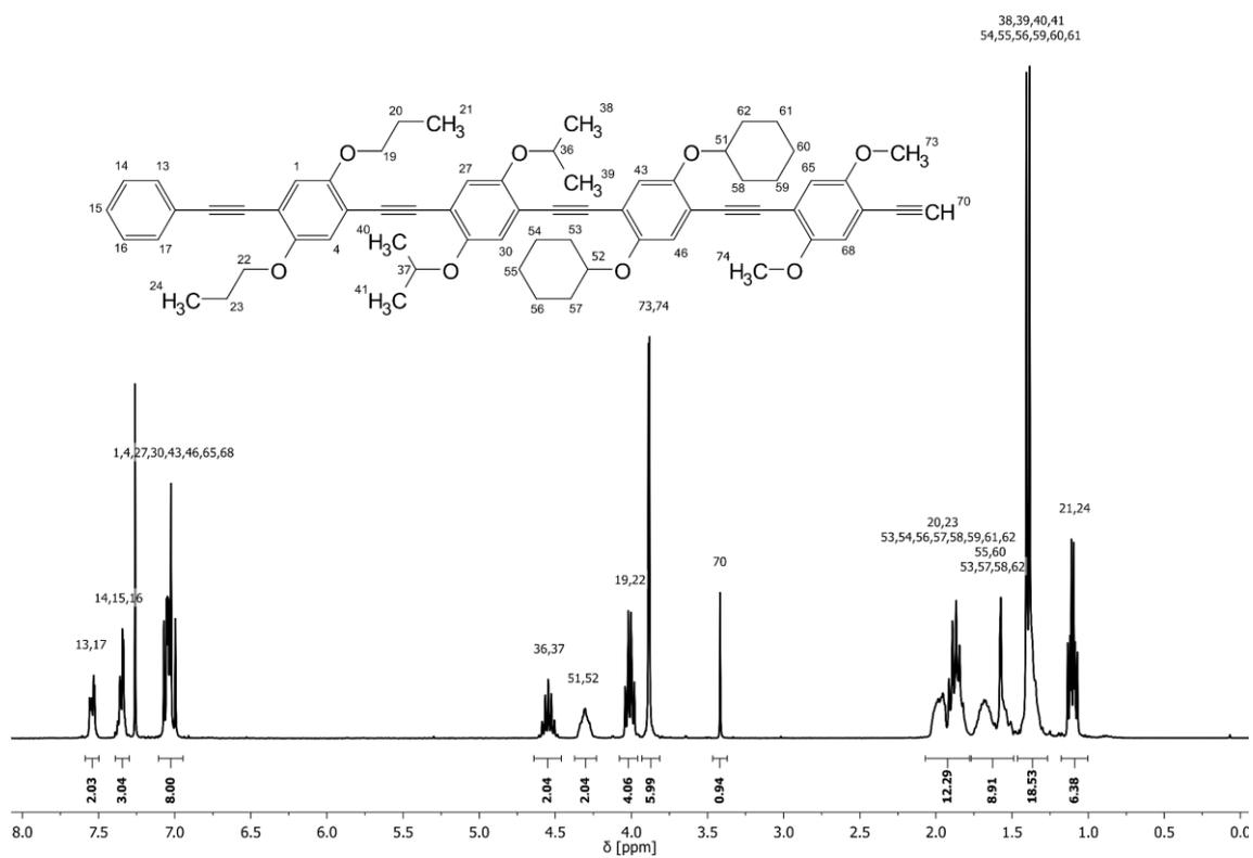
**Figure 78:** <sup>1</sup>H NMR spectrum of deprotected sequence-defined tetramer **4d** with assigned signals.
