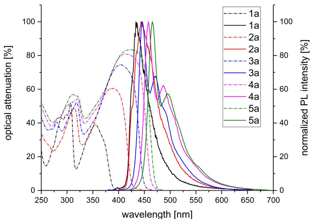
**Figure 23:** Absorption spectra (dotted) and PL spectra (bold) of protected monodisperse rod-like oligomers **1a-5a** in dichloromethane.
