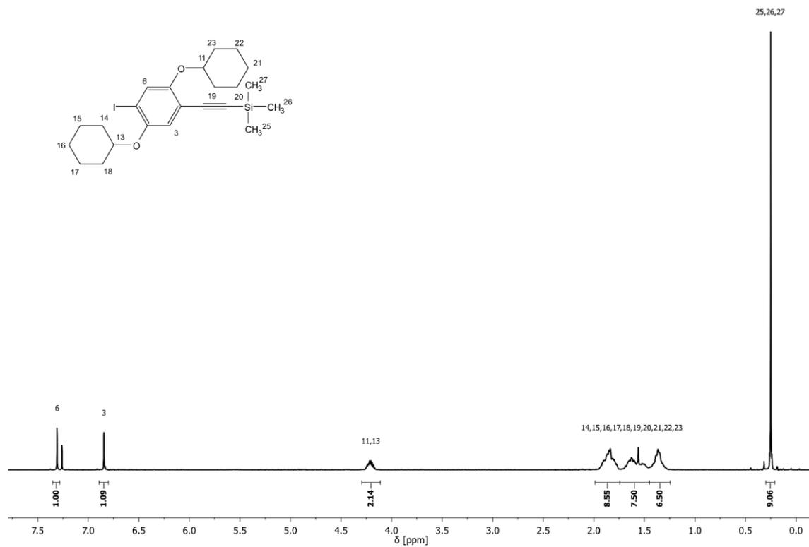
**Figure 50:** <sup>1</sup>H NMR spectrum of building block **B3** with assigned signals.
