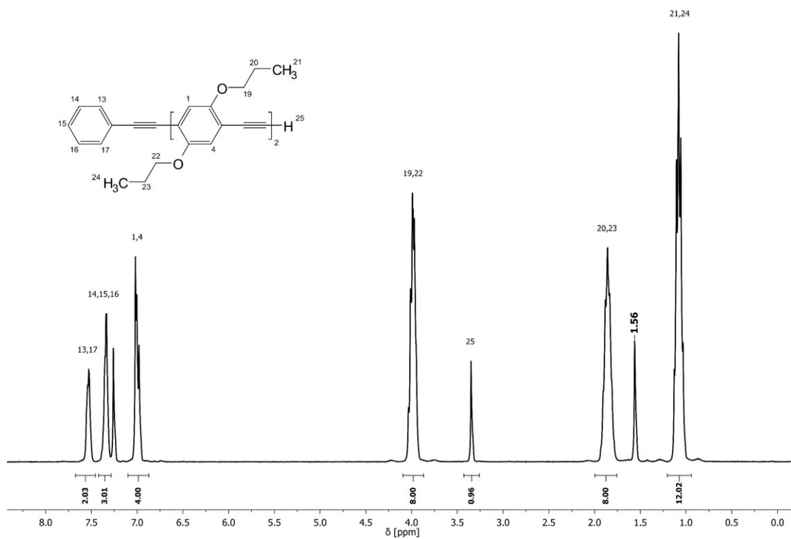
**Figure 65:** <sup>1</sup>H NMR spectrum of deprotected dimer **2b** with assigned signals.
