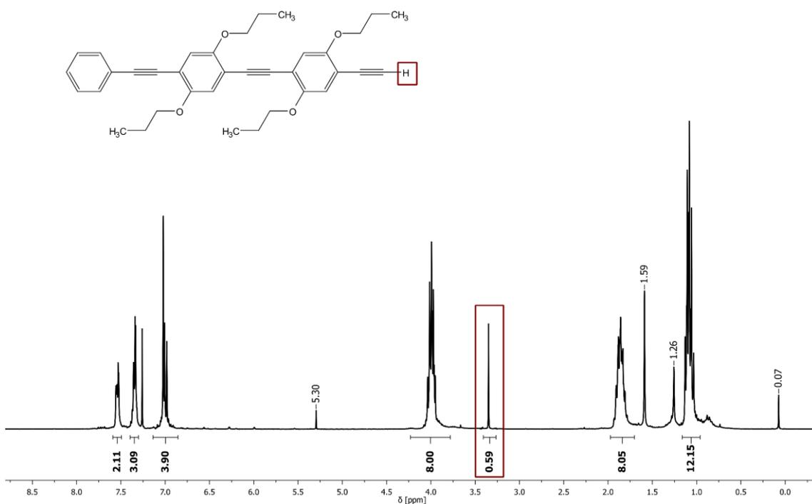
**Figure 18:** <sup>1</sup>H NMR spectrum of crude, deprotected dimer **2b**. The product is not pure, as the signal for the free hydrogen is too low (compare rectangles). However, the signals for the trimethylsilyl group around 0.26 ppm vanished, indicating that Glaser side product of **2b** is present.
