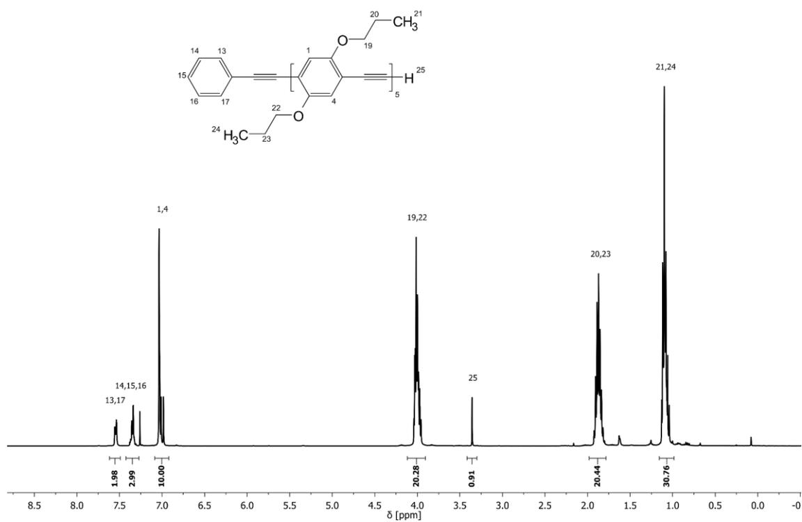
**Figure 71:** <sup>1</sup>H NMR spectrum of deprotected pentamer **5b** with assigned signals.
