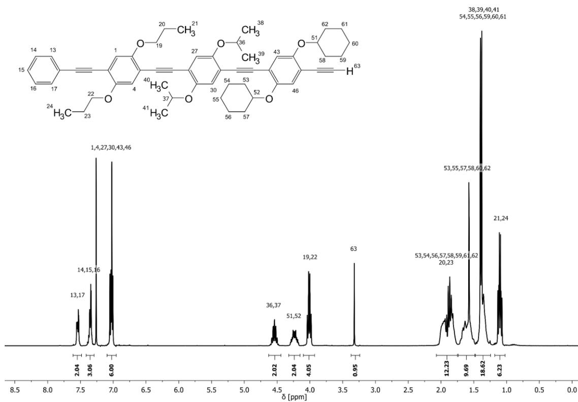
**Figure 76:** <sup>1</sup>H NMR spectrum of deprotected sequence-defined trimer **3d** with assigned signals.
