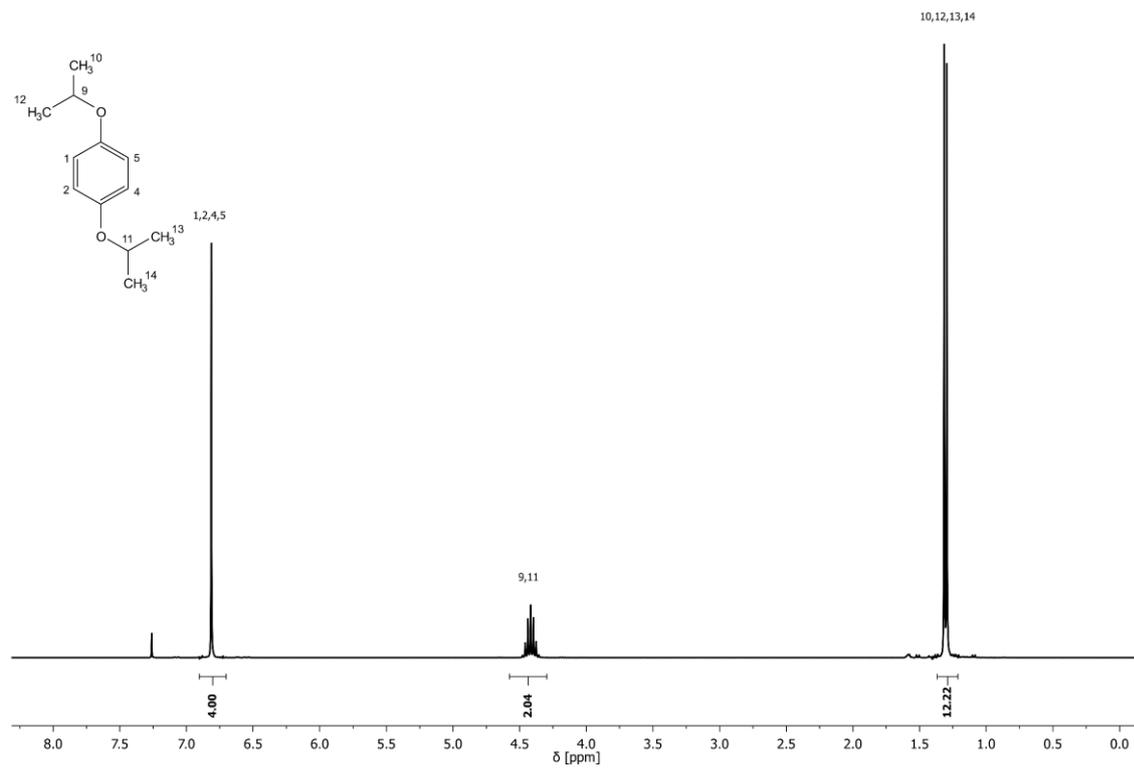
**Figure 45:** <sup>1</sup>H NMR spectrum of precursor **P2a** with assigned signals.
