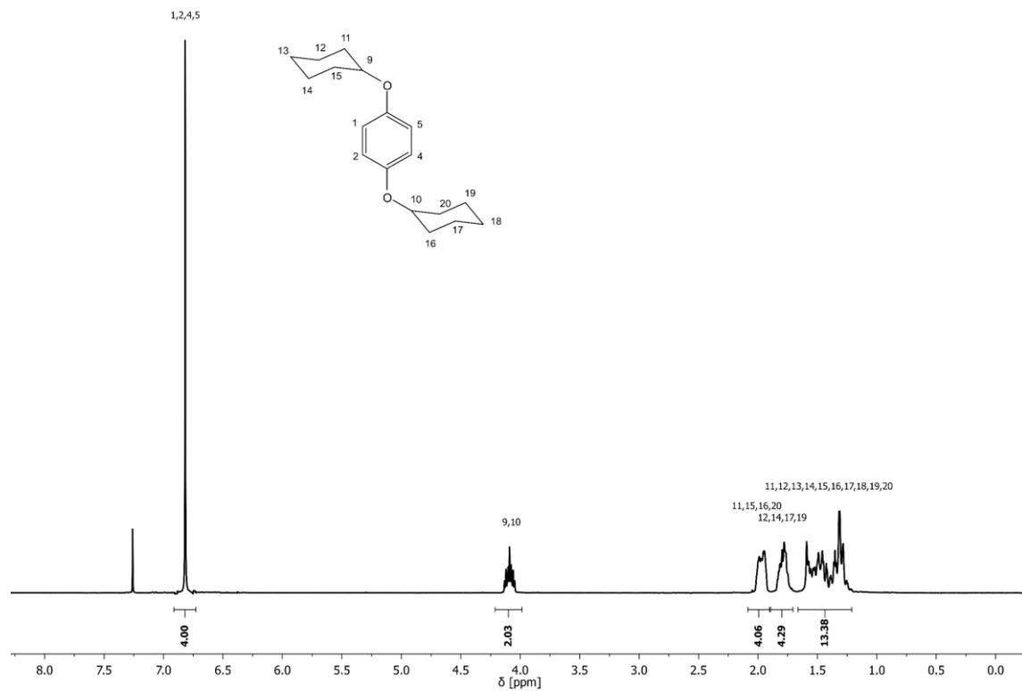
**Figure 48:** <sup>1</sup>H NMR spectrum of precursor **P3a** with assigned signals.
