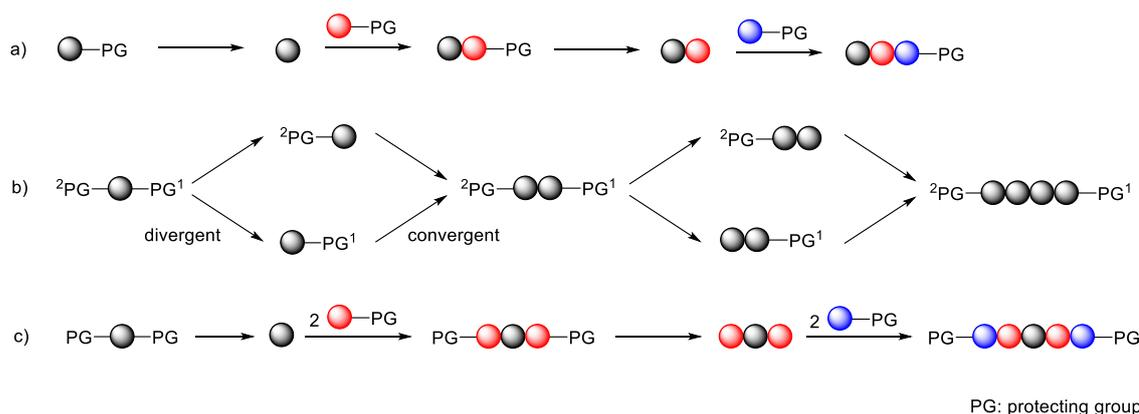
**Scheme 1:** Different approaches to monodisperse conjugated oligomers: a) linear approach, b) divergent/convergent approach (also termed iterative exponential growth), which requires two orthogonal protecting groups (PG)s, and c) bidirectional approach.
