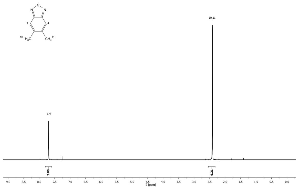
**Figure 57:** <sup>1</sup>H NMR spectrum of precursor **P7a** with assigned signals.
