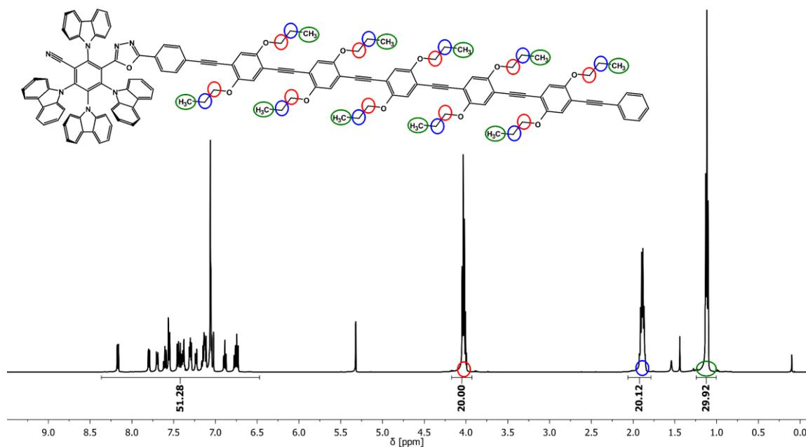
**Figure 40:**  $^1\text{H}$  NMR of pentamer-TADF adduct **T5** with assigned propoxy signals. The spectrum was recorded in dichloromethane- $d_2$  in order to suppress interference of the reference signals with other signals. The intensity of the aromatic signals amounts to 51, which corresponds to 51 aromatic protons.
