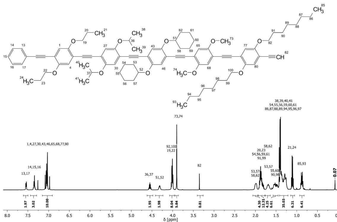
**Figure 80:**  $^1\text{H}$  NMR spectrum of deprotected sequence-defined pentamer **5d** with assigned signals.
