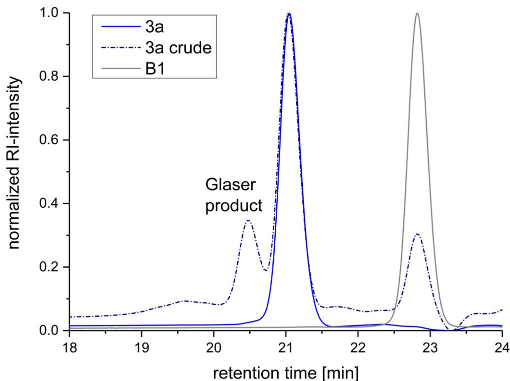
**Figure 19:** SEC trace of crude reaction mixture of trimer **3a** (dotted) in comparison to purified trimer **3a** (blue, bold) and the building block **B1** (grey, bold).
