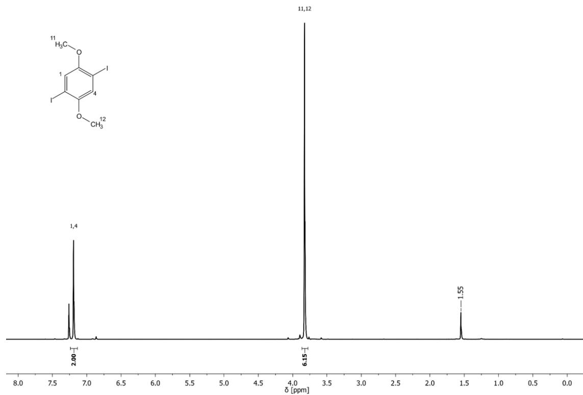
**Figure 51:**  $^1\text{H}$  NMR spectrum of precursor **P4** with assigned signals.
