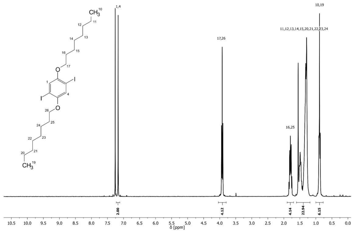
**Figure 54:** <sup>1</sup>H NMR spectrum of precursor **P5b** with assigned signals.
