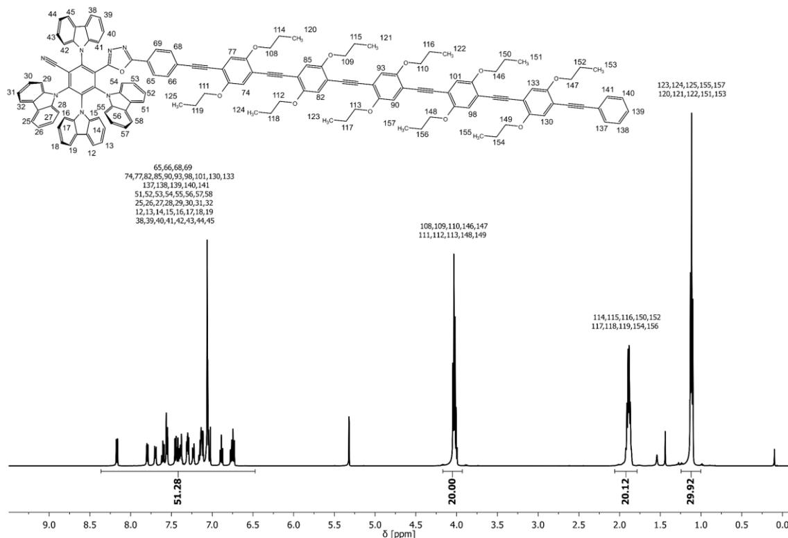
**Figure 83:** <sup>1</sup>H NMR spectrum of pentamer-TADF adduct T5 with assigned signals.
