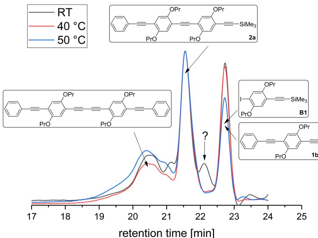
**Figure 17:** SEC traces of three crude mixtures for dimer **2a** formation, performed at different temperature (black: room temperature, red: 40 °C, blue: 50 °C). The respective compounds are assigned to the maximum intensities within the traces (from lower to higher retention times): Glaser side product, dimer **2a**, unknown (for room temperature trace only), building block **B1** and monomer **1b**, which exhibit the same retention time.
