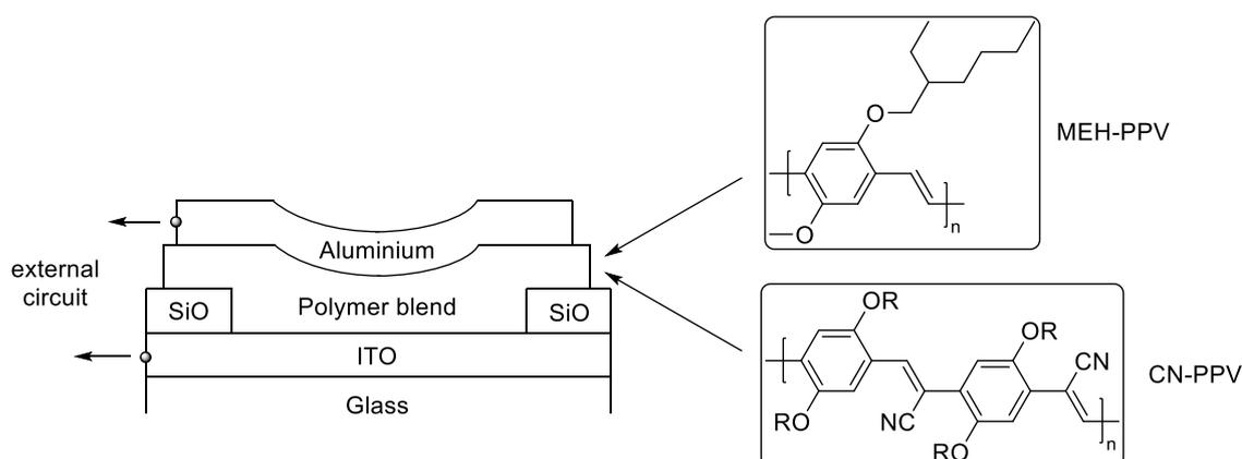
**Figure 10:** Plastic solar cell with ITO and aluminium electrodes. The polymer blend consists of MEH-PPV as donor and CN-PPV as acceptor.<sup>[215]</sup>
