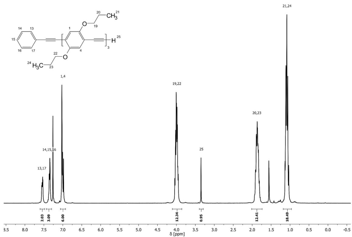
**Figure 67:** <sup>1</sup>H NMR spectrum of deprotected trimer **3b** with assigned signals.
