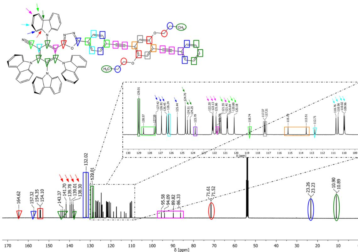
**Figure 37:**  $^{13}\text{C}$  NMR spectrum of monomer-TADF adduct **T1** with assigned signals. The spectrum was recorded in dichloromethane- $d_2$  in order to suppress interference of the reference signals with other signals. The carbazole unit signals are assigned by arrows in various colors, further aromatic signals are either allocated with rectangles or triangles and the propoxy signals with ellipsoids.
