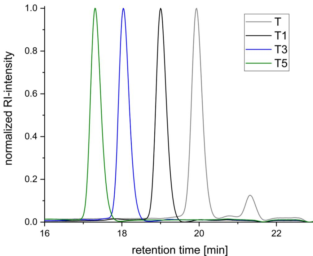
**Figure 41:** SEC traces of molecule **T** with TADF function (grey) and oligomer-TADF conjugates **T1** (black), **T3** (blue) and **T5** (green). The TADF molecule **T** exhibits a small impurity of 8% at a retention time of 21 min.
