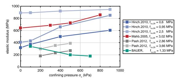
Figure 3.9: Elastic modulus as a function of confining pressure at 28 days
