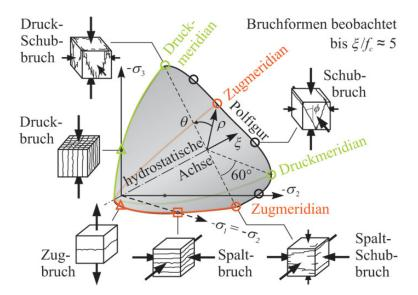
Figure 3.5: Change in concrete failure mode depending on stress level relationship (in German) [121]
