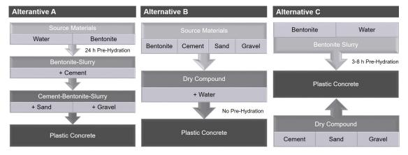
Figure 2.5: Representative examples of Plastic Concrete mixing sequences
