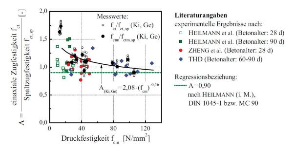
Figure 3.4: Overview of the  $f_{ct}/f_{ct,sp}$ -ratio of concrete over compressive strength  $f_{cm}$  (in German) [102]
