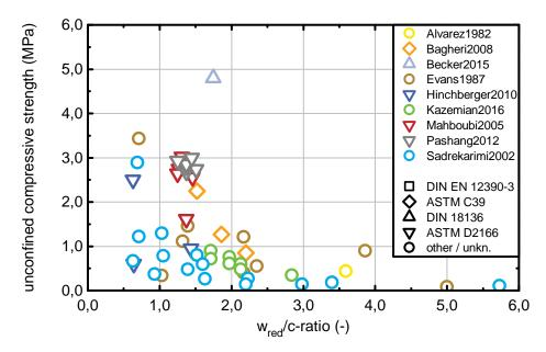
Figure 3.2: Overview of the UCS of Plastic Concrete as a function of w<sub>red</sub>/c at 28 days
