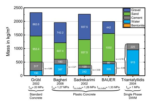
Figure 2.4: Representative examples of Plastic Concrete mix designs
