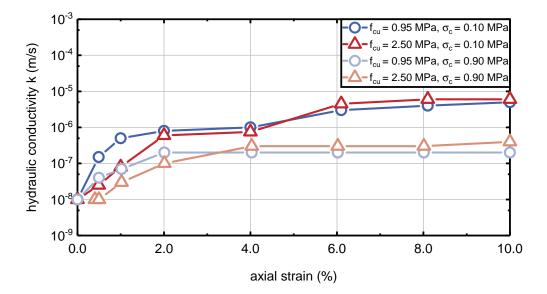
Figure 4.3: Hydraulic conductivity of Plastic Concrete with distinct compressive strengths  $f_{cu}$  at varying confining pressures  $\sigma_c$  (following [80])
