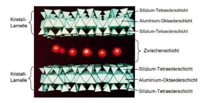
Figure 2.2: Schematic illustration of montmorillonite structure [112]
