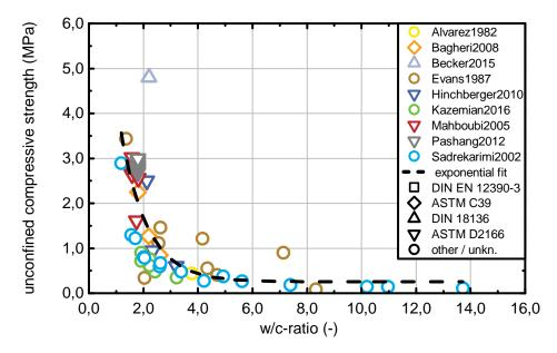
Figure 3.1: Overview of the UCS of Plastic Concrete as a function of w/c-ratio at 28 days
