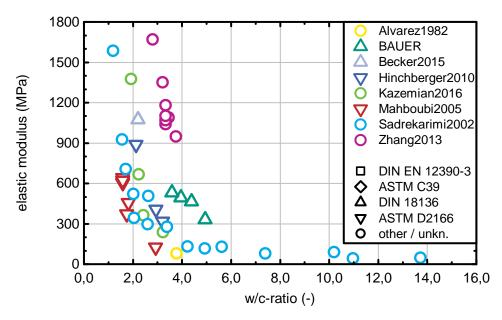
Figure 3.7: Overview of the elastic modulus as a function of the w/c-ratio at 28 days
