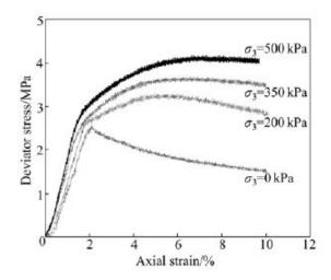
Figure 3.6: Variation of deviator stress versus axial strain for unconfined and triaxial compression tests [110]
