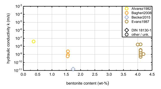
Figure 4.4: Hydraulic conductivity of Plastic Concrete over bentonite content at  $\sigma_c = 0$
