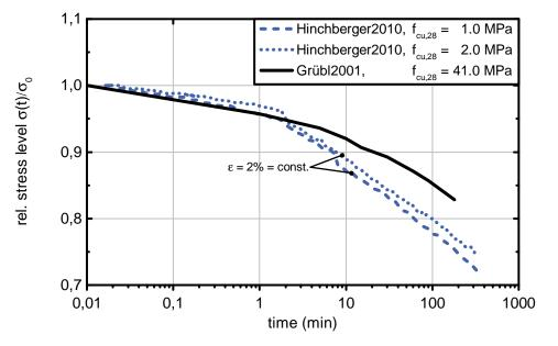
Figure 3.10: Stress relaxation of concrete samples over time
