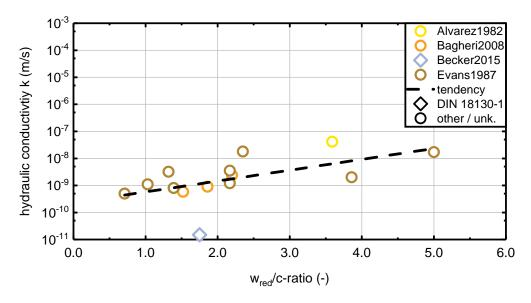
Figure 4.1: Hydraulic conductivity of Plastic Concrete over  $w_{red}/c$ -ratio at  $\sigma_c = 0$
