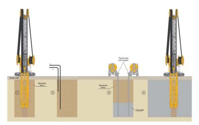
Figure 1.2: Construction of a Cut-Off Wall with the Two-Phase Method [27]
