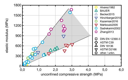
Figure 3.8: Elastic modulus as a function of the compressive strength at 28 days
