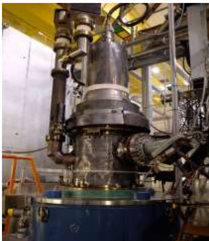
Fig. 3: The coaxial-cavity long-pulse gyrotron in the Oxford Instruments superconducting magnet with the calorimeter for the RF power measurement.
