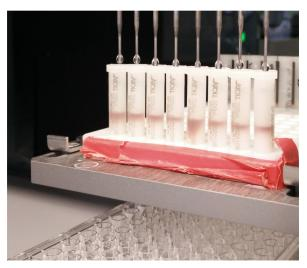
Figure 3.1: Microscale chromatography executed on a liquid-handling station
