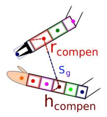
Fig. 1: Separation distance calculation between robot and human key points.
