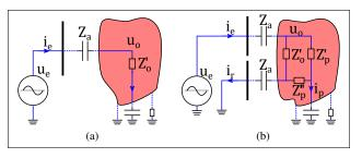
Fig. 1: Projected capacitance measurement methods: 1a) self capacitance, 1b) mutual capacitance.
