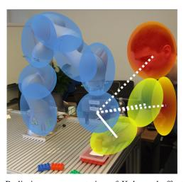
Fig. 3: Preliminary representation of Kuka end-effector and human key point pairs. Ellipses approximate the key point compensation coefficient areas.
