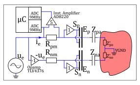
Fig. 2: Schematic of the analog front-end. Creation of a virtual ground within the target with a second differential signal.
