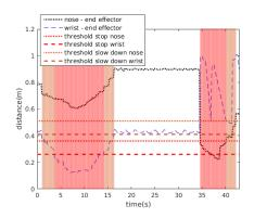
Fig. 2: Head and body discrimination: A higher separation threshold for the human head region w.r.t. Nao robot's end-effector. Yellow areas mark the robot's slower movement and red areas mark when he stopped.
