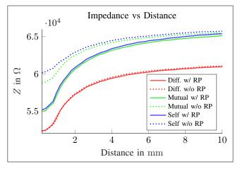
Fig. 3: Measurement of impedance at distances ranging from 0.2 mm to 10 mm. Dotted lines represent an isolated target without return path, whereas solid lines represent targets with return path.
