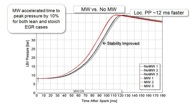
Figure 8. MW Can Accelerate Stoichiometric EGR Combustion
