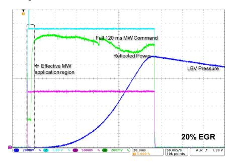
Figure 7. Example MEC MW Instrumentation Signal Traces - Accelerated Combustion Test
