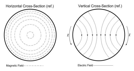
Figure 1: Cross-Section of Spherical Cavity Mode, TM101
