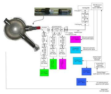
Figure 3: MEC system for Combustion Tests
