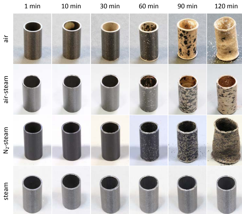
Figure 3: Post-test appearance of samples oxidised at 900°C in specified atmospheres.
