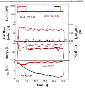
**Figure 5.** Comparison of two plasmas without (20171207.038) and with ECCD (20171207.049) to compensate the bootstrap current. The time traces (of ECRH power, gas flow and line integrated density, plasma energy, central electron temperature from ECE and plasma current) of the reference case without ECCD are plotted in black. In the counter-ECCD case (plotted in red), the total current (measured by a Rogowski coil) remains close to zero.
