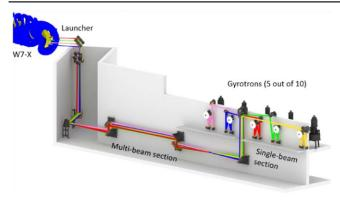
**Figure 1.** Illustration of one-half of the W7-X ECRH facility (reproduced with permission from [22]). The gyrotron beams are collected in the single-beam section and optically transmitted together over approximately 30 m in the multi-beam section, before they are divided into single beams again near the launchers. The other half of the facility (not shown) is a mirror image of the one shown.
