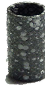
SiC-SiC f cladding after 64 h at 1600°C in steam
