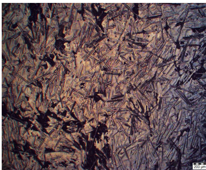
Figure 12. An example image of lightly pressed paraffin wax-based feedstock with 50 vol % of fibers in solid content for measuring the fiber length.
