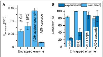
FIGURE 7 | Comparison of expected and experimental conversion in flow reactor experiments. (A) Reaction rate constant calculated from batch experiments for the respective enzymes. (B) Expected conversion in the flow reactor experiments based on first-order kinetics, calculated with kapp,hydro,exp (A) compared to the experimental conversion of the respective reactor experiments (see Figure 6) in the steady state.
