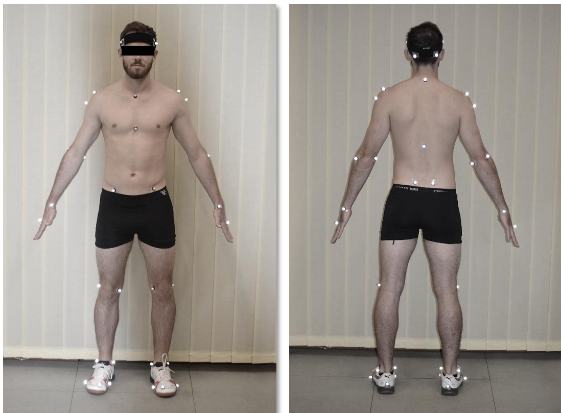
Figure 7. Marker Set. Left: Frontal view and Right: Dorsal view of a subject with the attached 42 retro-reflective spherical markers (diameter 19 mm) according to the ALASKA Dynamicus 9 model (HÄRTEL & HERMSDORF 2006).
