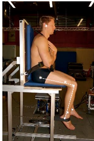
Figure 11. Isometric Force Test. This figure presents the testing condition under 90° knee flexion angle. The subjects were fixed to the rigid chair with seat belts around the chest and the stomach. The backrest was fixed perpendicular to the seat. The subjects had to cross the arms over their chests to prevent any support of the arms during the force measurements. The strap, which was connected to the force sensor (strain-gauge system), was fixed around the ankle joint in horizontal extension to the force sensor. This ensured a stable knee angle position throughout the contraction. The subjects had to perform maximum voluntary contractions against the resistance of the fixed strap under isometric conditions. By changing the direction of the strap, force capacities were detectable under isometric knee flexion and isometric knee extension situation with the same measurement device.
