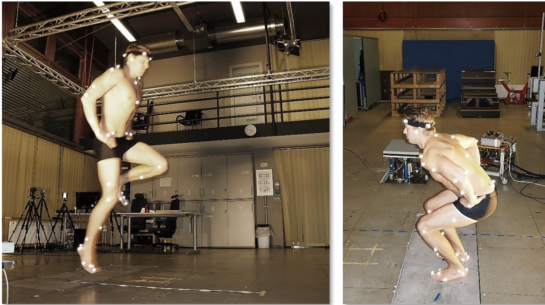
Figure 10. Jumping Tasks of the Test Battery. Left: One-legged jumping task for distance akimbo. In this task, the subjects had to jump-off and land stable on the same leg. The task was performed with both legs separately. Right: Bilateral counter movement jumping task akimbo. The subjects had to jump-off and land stable on both force plates. The jumping task was determined valid, if each foot was placed separately on one force plate during the jump-off and landing phase.
