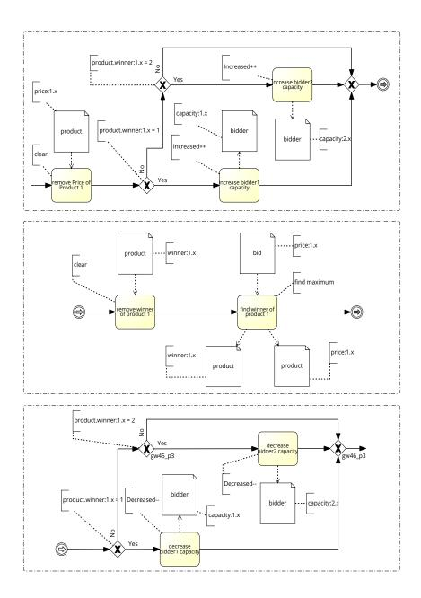
Figure 14: BPMN enhancement of Process 1 for winner determination and capacity rule regarding product 1
