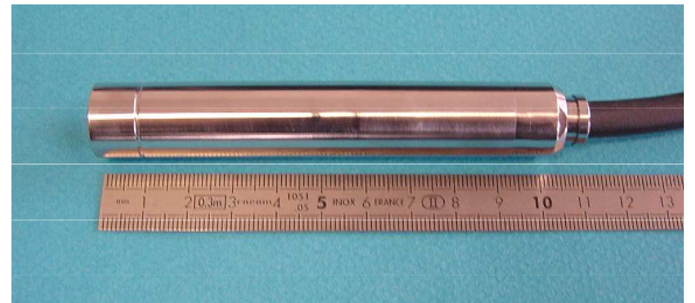
SO16 type CdTe detector from EURORAD. The metal tube contains the CdTe detector and the charge-sensitive preamplifier.
