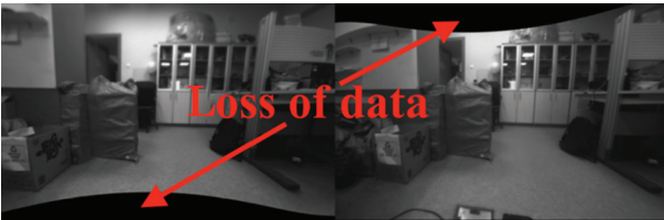
Figure 12 | Loss of data after calibration of the robot's stereo pair (rectification process). Black areas represent the lost pixels
