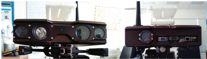
Figure 2 | Servosila Engineer's front and rear view cameras
