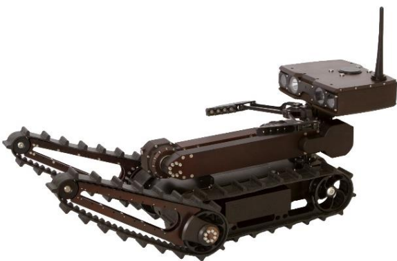
Fig. 1. "Servosila" Engineer crawler-type UGV. Courtesy of "Servosila" company.
