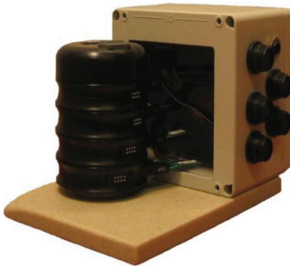
Supplementary Figure 3.1. Braille stimulator. A Braille stimulator has five Braille cells built-in (four on the side, one on the top) and a response button (also on the top). Each Braille cell contains 8 pins, aligned in 2 series of 4, that can be raised and lowered. Individual Braille cell positions are adjustable. When grasped, all five fingertips overlie a Braille cell. Two such devices were used in the experiment, one for each hand.
