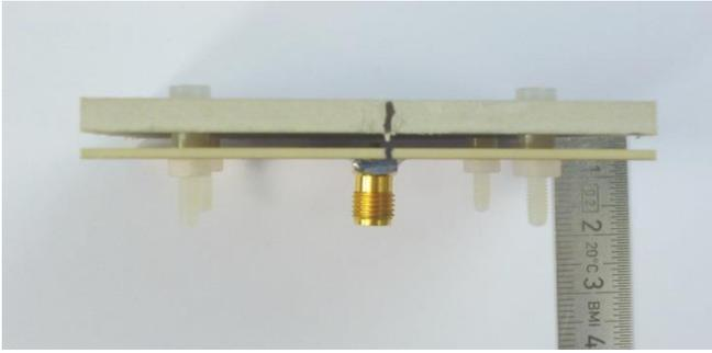
Figure 4. Side view of milled patch array
