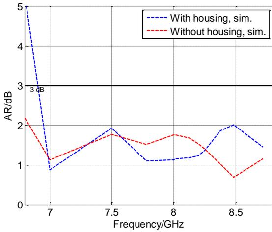
Figure 8. Simulated axial ratio of the antenna array
