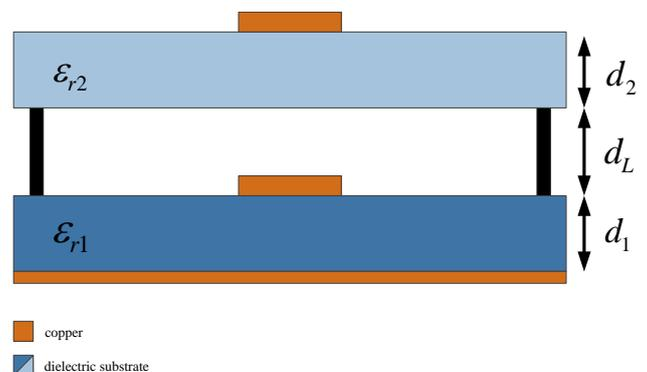
Figure 1. Schematic representation of stacked patch structure
