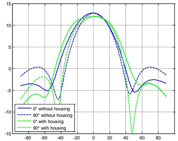
Figure 7. Simulated radiation pattern for 8.25 GHz
