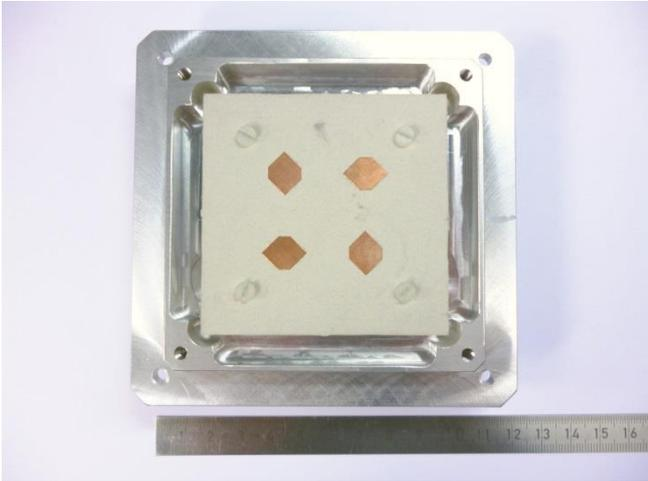
Figure 5. Patch antenna array with mounted housing
