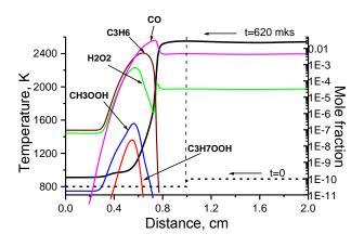
The system has stratification in the form of the alternation of discharge filaments (x>1cm in figure) and free space (x $\leq$ 1cm). The initial heating and concentrations of radicals produced by the discharge were determined in an approximation of a constant reduced electric field at the different input specific energies Q. The spatial distribution of components at the ignition moment of at t = 620 µs
